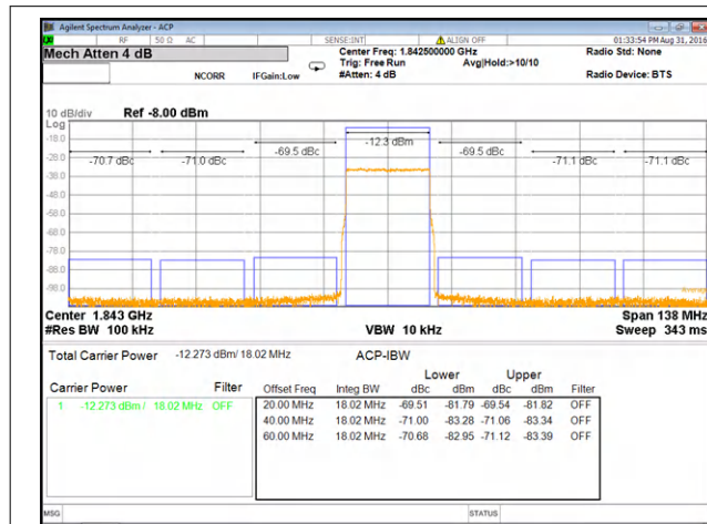
Figure 8-4. Dual band ACPR Performance in Downlink Band 3 with On-chip PLL
