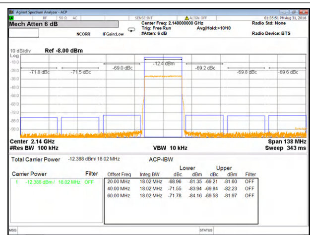
Figure 8-5. Dual band ACPR Performance in Downlink Band 1 with On-chip PLL
