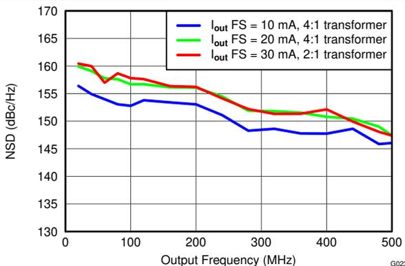
Figure 5-23. NSD vs Output Frequency Over  $I_{OUTFS}$
