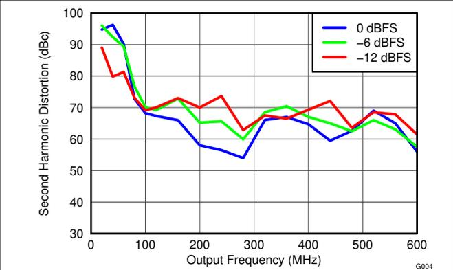
**Figure 5-4. Second Harmonic Distortion vs Output Frequency Over Input Scale**
