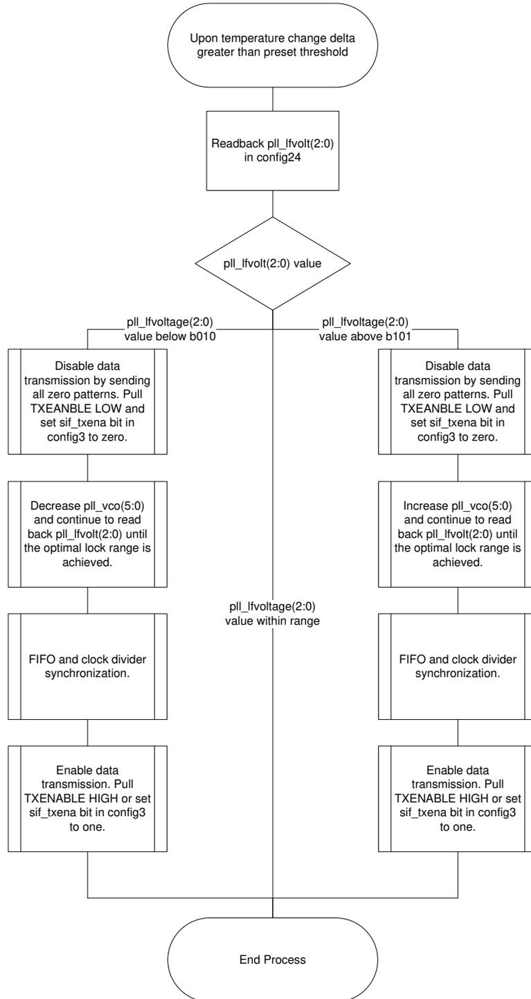
**Figure 6-10. Example PLL Lock Status and Adjustment Algorithm**
