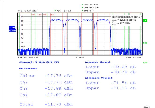
**Figure 5-31. Four Carrier W-CDMA Test Model 1**
