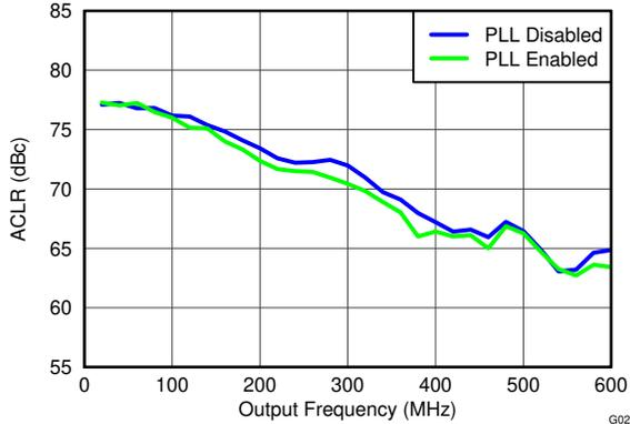
**Figure 5-25. Single Carrier WCDMA ACLR (Adjacent) vs Output Frequency Over Cloning Options**
