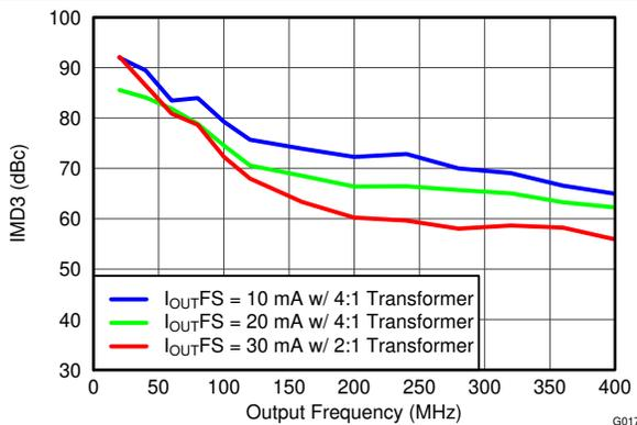
Figure 5-17. IMD3 vs Output Frequency Over  $I_{OUTFS}$
