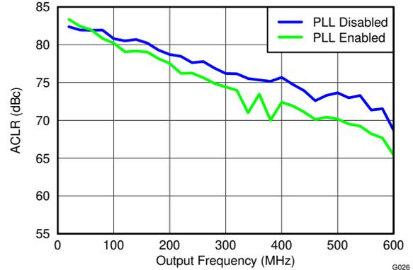
**Figure 5-26. Single Carrier WCDMA ACLR (Alternate) vs Output Frequency Over Cloning Options**
