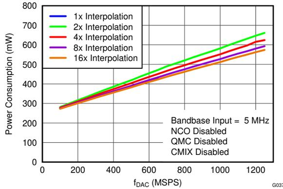
Figure 5-37. Power Consumption vs  $f_{DAC}$  Over Interpolation
