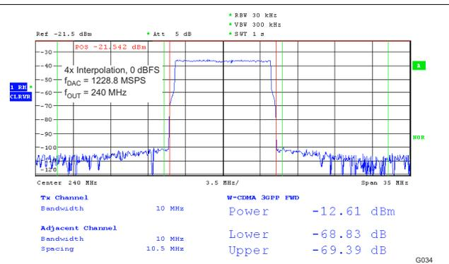
**Figure 5-34. 10 MHz Single Carrier LTE Test Model 3.1**
