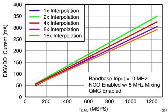
Figure 5-41. DIGVDD Current vs  $f_{DAC}$  Over Interpolation
