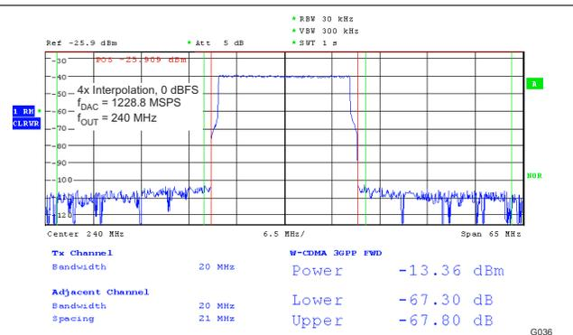
**Figure 5-36. 20 MHz Single Carrier LTE Test Model 3.1**
