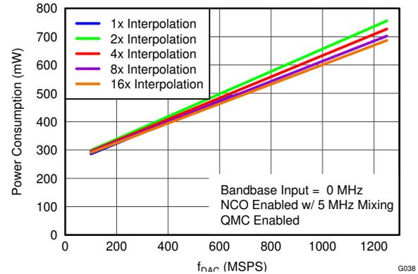
Figure 5-38. Power Consumption vs  $f_{DAC}$  Over Interpolation
