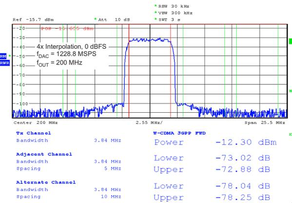
**Figure 5-29. Single Carrier W-CDMA Test Model 1**
