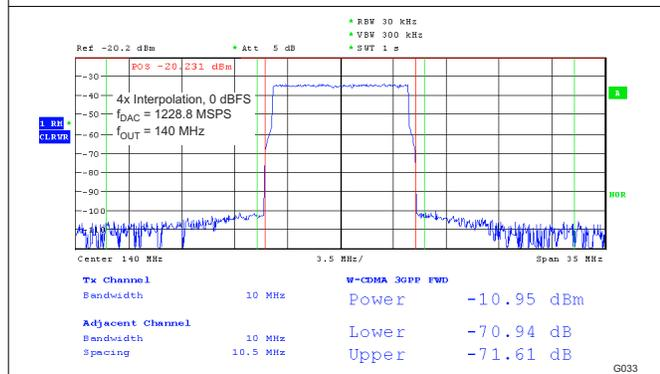
**Figure 5-33. 10 MHz Single Carrier LTE Test Model 3.1**
