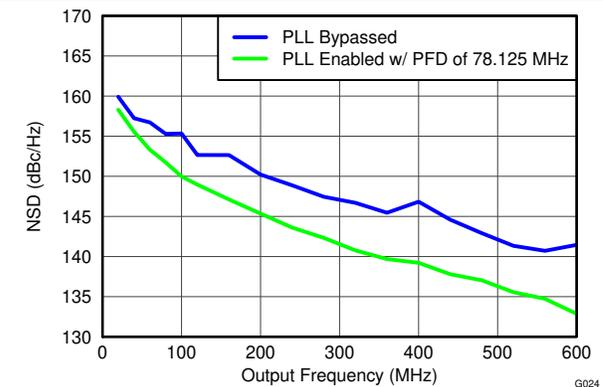
Figure 5-24. NSD vs Output Frequency Over Clocking Options
