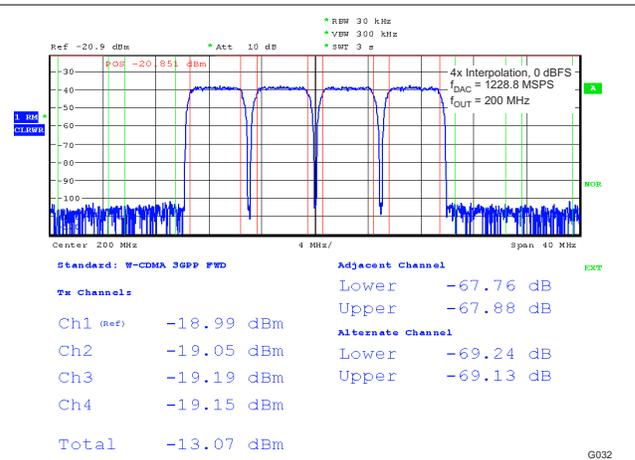
**Figure 5-32. Four Carrier W-CDMA Test Model 1**
