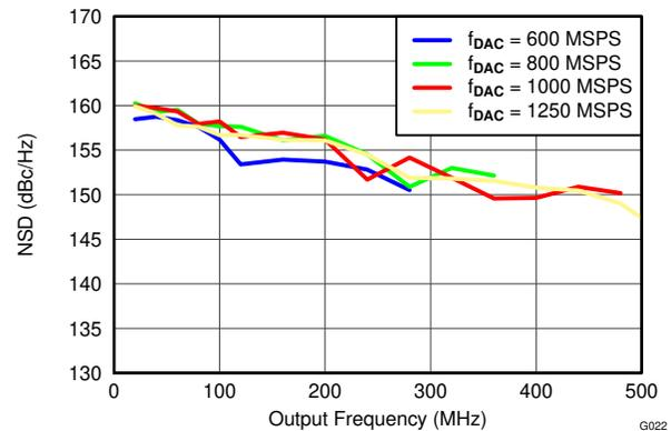
Figure 5-22. NSD vs Output Frequency Over  $f_{DAC}$
