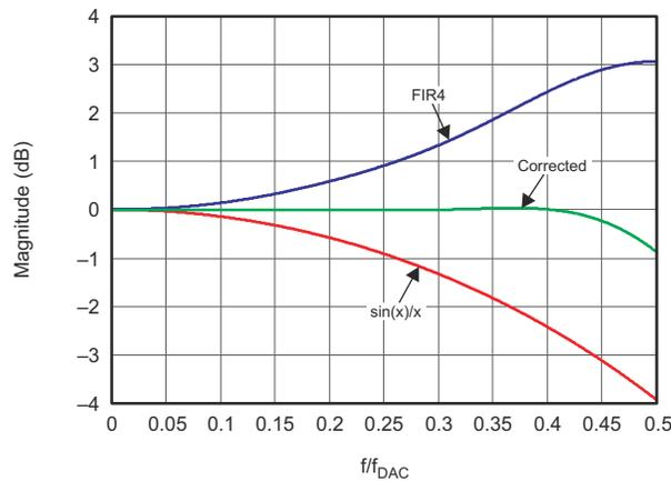
**Figure 6-20. Magnitude Spectrum for Inverse Sinc Filter**
