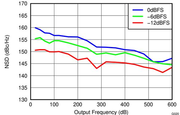
Figure 5-20. NSD vs Output Frequency Over Input Scale
