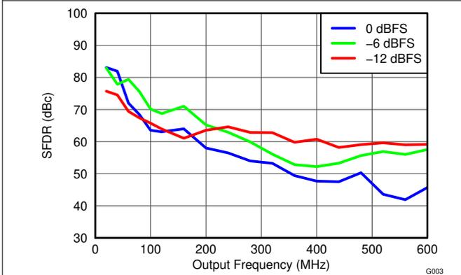
**Figure 5-3. SFDR vs Output Frequency Over Input Scale**
