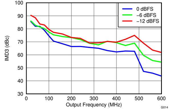
Figure 5-14. IMD3 vs Output Frequency Over Input Scale
