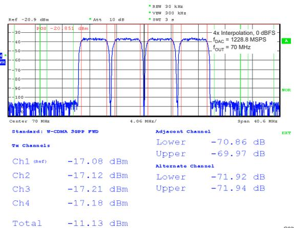
**Figure 5-30. Four Carrier W-CDMA Test Model 1**
