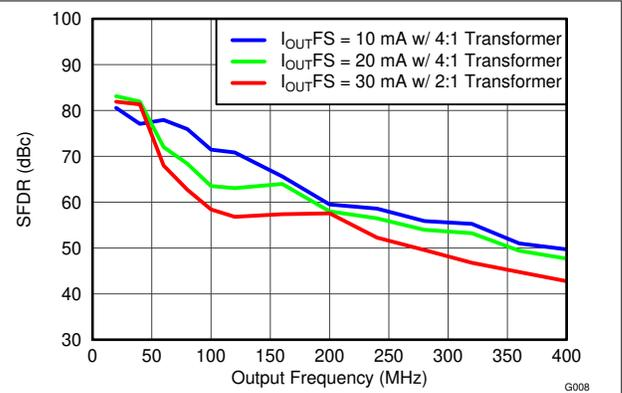
Figure 5-8. SFDR vs Output Frequency Over  $I_{OUTFS}$
