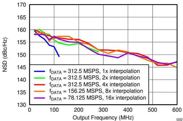
Figure 5-21. NSD vs Output Frequency Over Interpolation
