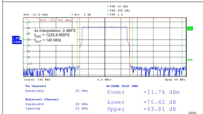
**Figure 5-35. 20 MHz Single Carrier LTE Test Model 3.1**
