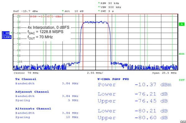
**Figure 5-27. Single Carrier W-CDMA Test Model 1**
