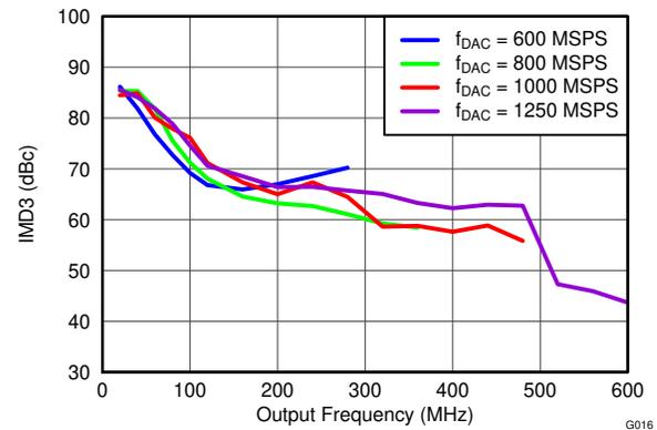
Figure 5-16. IMD3 vs Output Frequency Over  $f_{DAC}$
