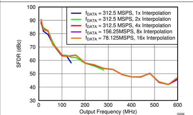
**Figure 5-6. SFDR vs Output Frequency Over Interpolation**
