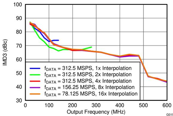
Figure 5-15. IMD3 vs Output Frequency Over Interpolation
