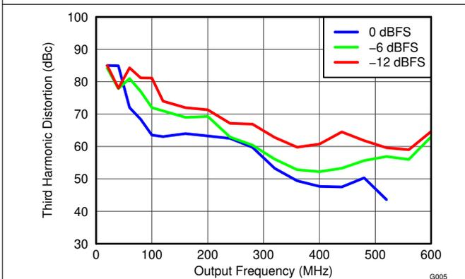
**Figure 5-5. Third Harmonic Distortion vs Output Frequency Over Input Scale**
