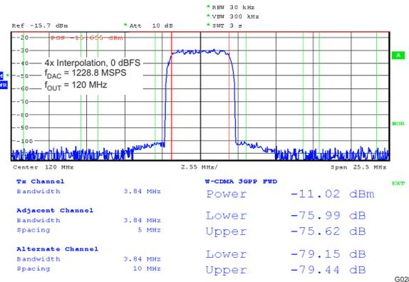
**Figure 5-28. Single Carrier W-CDMA Test Model 1**
