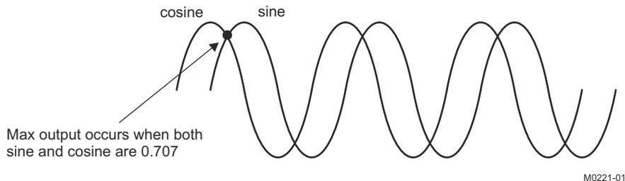
**Figure 6-24. Maximum Output of the Complex Signal Multiplier**
