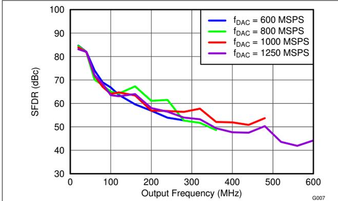
Figure 5-7. SFDR vs Output Frequency Over  $f_{DAC}$
