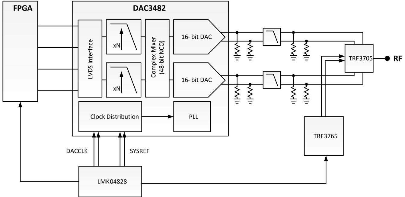
**Figure 7-1. Dual Low-IF Wideband LTE Transmitter Diagram**
