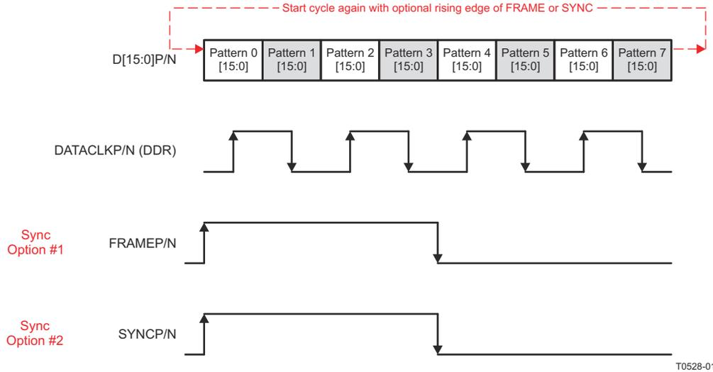
Figure 6-27. IO Pattern Checker Data Transmission Format
