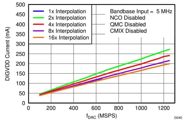
Figure 5-40. DIGVDD Current vs  $f_{DAC}$  Over Interpolation
