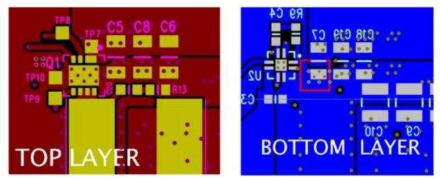
Figure 33. Recommended PCB Layout (Top Down)
