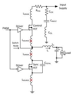
Figure 28. Elimination of Parasitic Inductances
