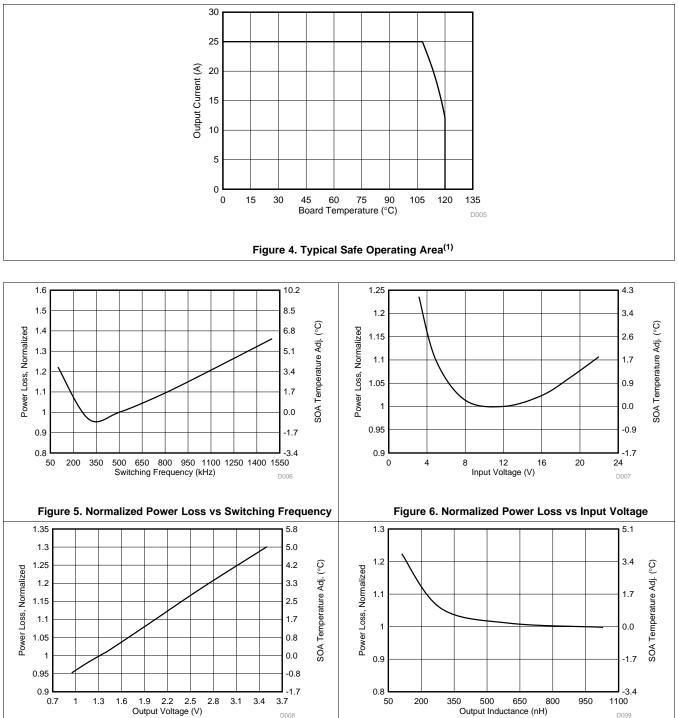
Figure 7. Normalized Power Loss vs Output Voltage
