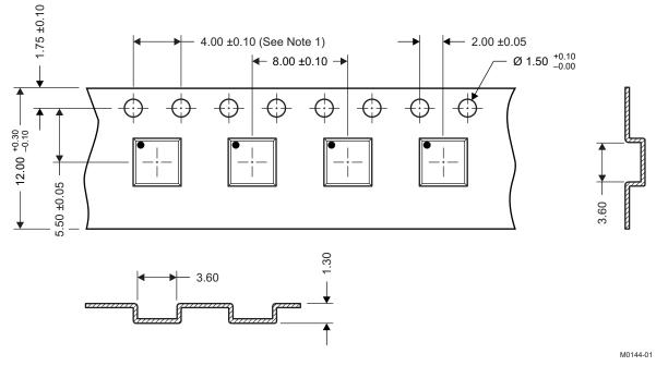
NOTES: 1. 10-sprocket hole-pitch cumulative tolerance ±0.2.
