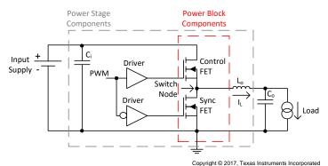
Figure 27. Equivalent System Schematic
