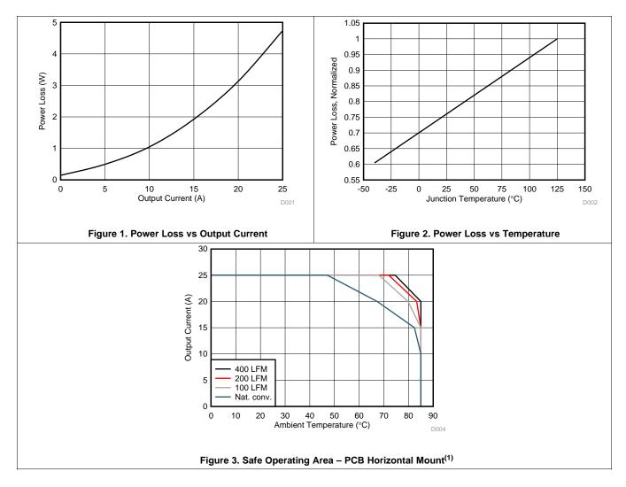
(1) The Typical Power Block System Characteristic curves are based on measurements made on a PCB design with dimensions of 4 in (W) × 3.5 in (L) × 0.062 in (H) and 6 copper layers of 1-oz copper thickness. See *Applications and Implementation* section for detailed explanation.
