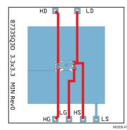
$\label{eq:rescaled} \begin{array}{l} Max \; R_{\theta JA} = 73 \mbox{°C/W} \\ \mbox{when mounted on 1 } in^2 \\ (6.45 \; cm^2) \; of \; 2\text{-}oz \\ (0.071\text{-}mm) \; thick \; Cu. \end{array}$
