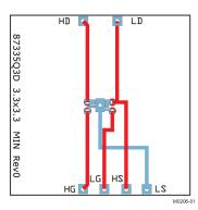
Max  $R_{\theta JA} = 135^{\circ}C/W$ when mounted on minimum pad area of 2-oz. (0.071-mm) thick Cu.
