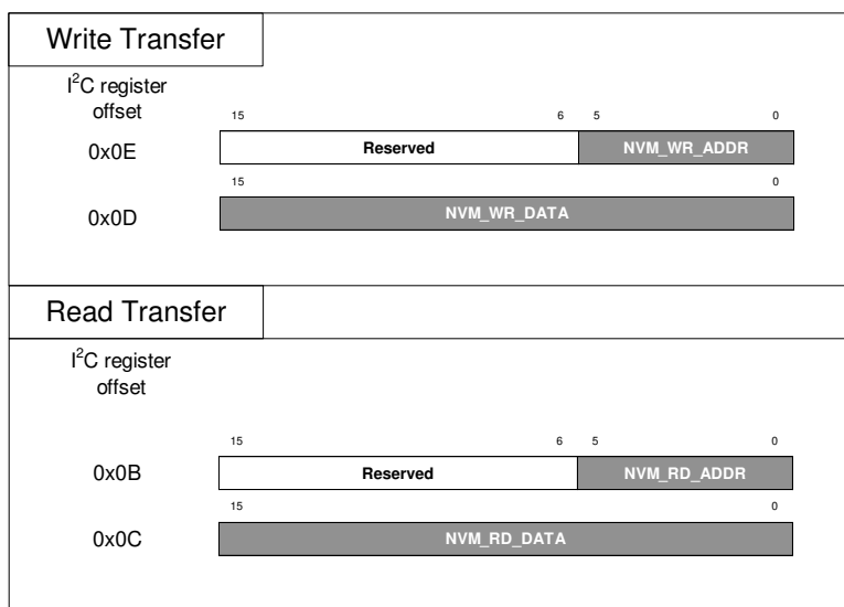
Figure 8-12. EEPROM Direct Access Using I 2 C
