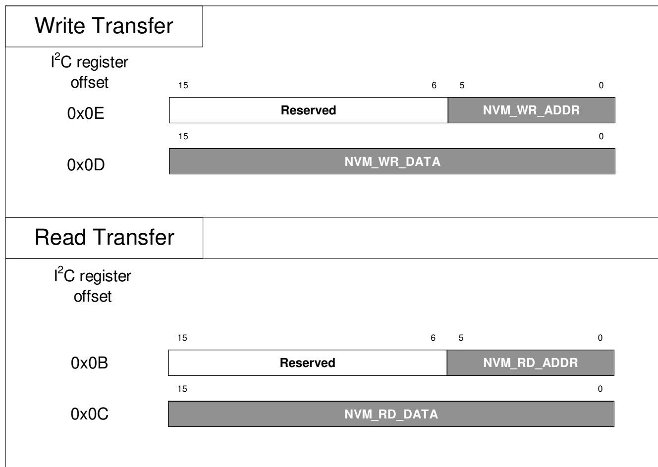
Figure 7-12. EEPROM Direct Access Using I 2 C
