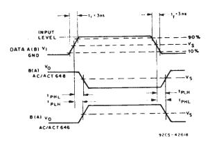
Fig. 3 - Propagation delay times.
