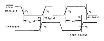
Fig. 4 - Data setup and hold times.
