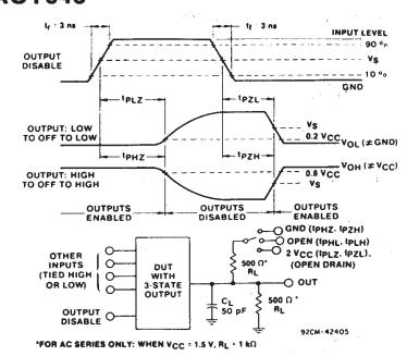
Fig. 2 - Three-state propagation delay waveforms and test circuit.
