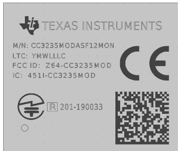
Figure 8-6. CC3235MODASF Module Marking
