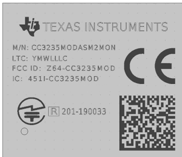
Figure 8-5. CC3235MODAS Module Marking
