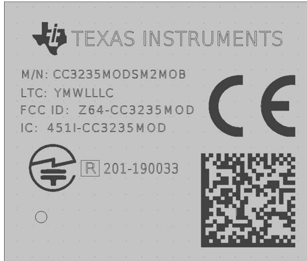
Figure 8-3. CC3235MODS Module Marking
