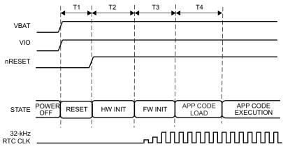
T1 should be  $\geq$ 200 ms without a pulldown resistor on the XTAL\_N pin or T1 should be  $\geq$ 100  $\mu$ s if there is 2-M $\Omega$  pulldown resistor on the XTAL N pin.
