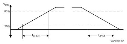
Figure 8-17. GPIO Timing Diagram
