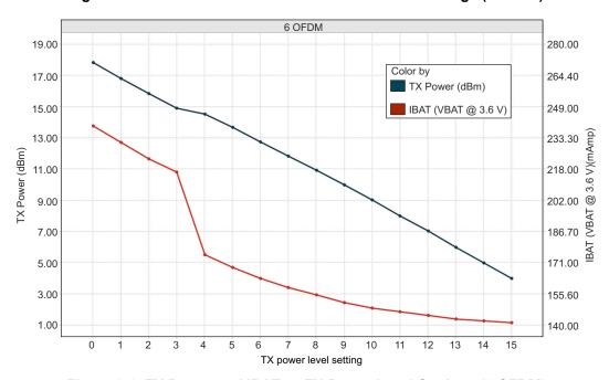
Figure 8-2. TX Power and IBAT vs TX Power Level Settings (6 OFDM)
