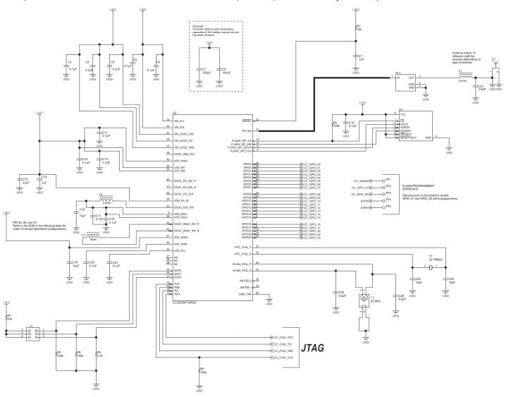
Figure 10-2. CC3220x Preregulated 1.85-V Mode Application Circuit
