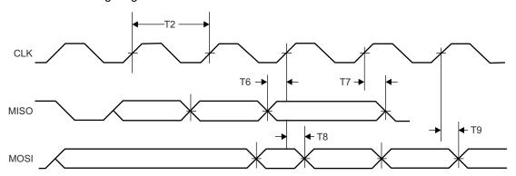
Figure 8-13. SPI Master Timing Diagram
