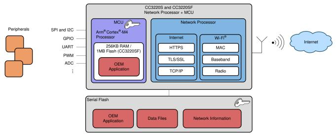
Figure 9-2. CC3220S and CC3220SF High-Level Structure
