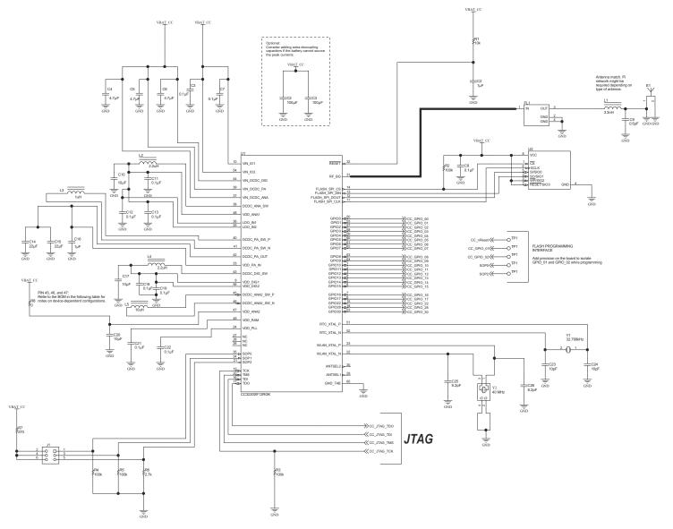
Figure 10-1. CC3220x Wide-Voltage Mode Application Circuit
