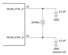
A. The crystal capacitance must be tuned to ensure that the PPM requirement is met. See CC31xx & CC32xx Frequency Tuning for information on frequency tuning.
