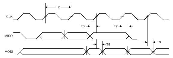
Figure 8-14. SPI Slave Timing Diagram
