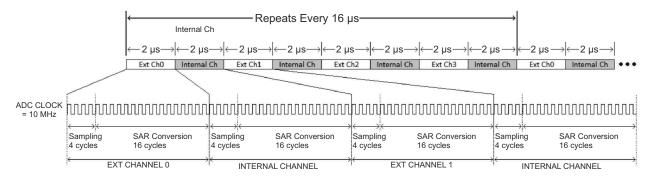
Figure 8-20. ADC Clock Timing Diagram
