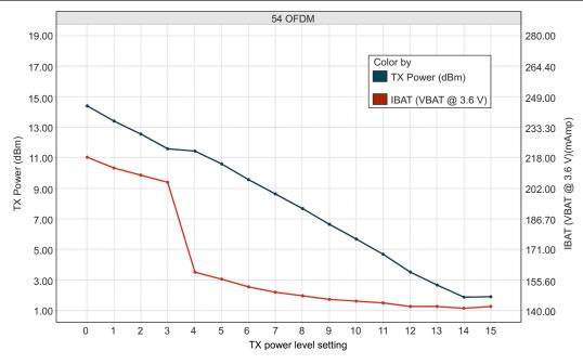
Figure 8-3. TX Power and IBAT vs TX Power Level Settings (54 OFDM)
