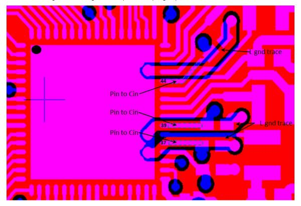
Figure 10-3. Ground Routing for the Input Decoupling Capacitors
