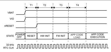
Figure 8-7. First-Time Power-Up and Reset Removal Timing Diagram (External 32-kHz)
