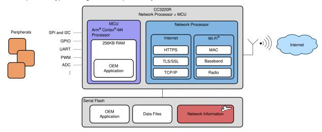
Figure 9-1. CC3220R High-Level Structure
