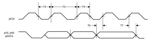
Figure 8-21. Camera Parallel Port Timing Diagram
