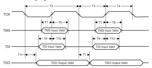
Figure 8-19. JTAG Timing Diagram
