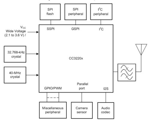
Figure 4-1. Functional Block Diagram
