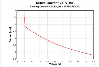
Figure 8-4. Active Mode (MCU) Current vs. Supply Voltage (VDDS) (Running CoreMark, SCLK\_HF = 48 MHz RCOSC)
