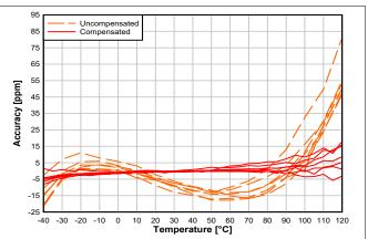
Figure 8-32. Temperature Compensation of the RF Frequency
