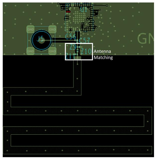
Figure 10-2. Module Layout Guidelines
