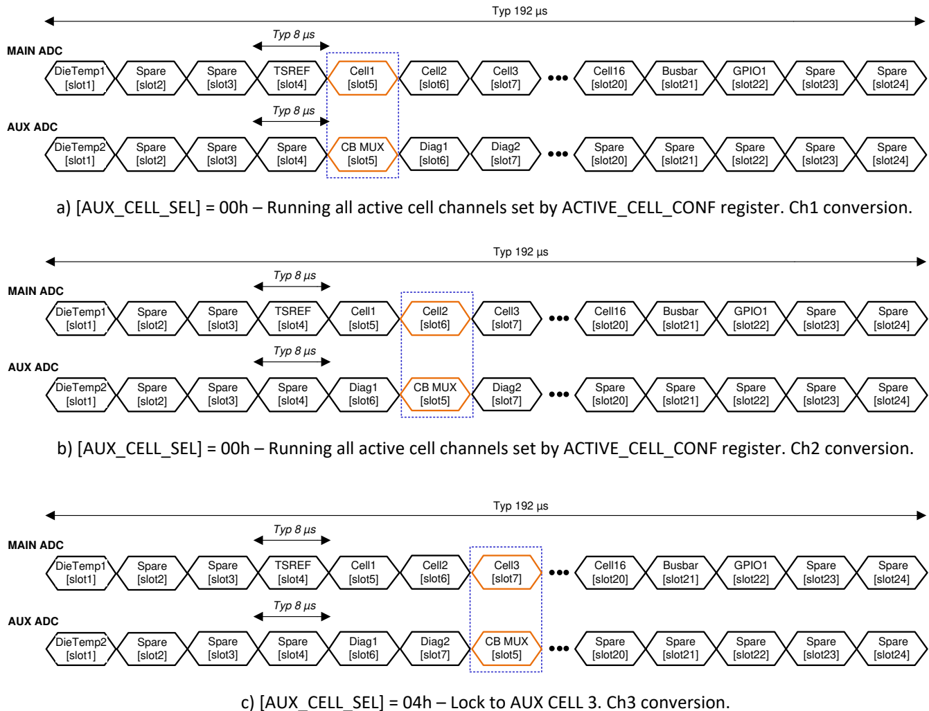
Figure 9-12. Synchronization between MAIN and AUX ADC Sampling
