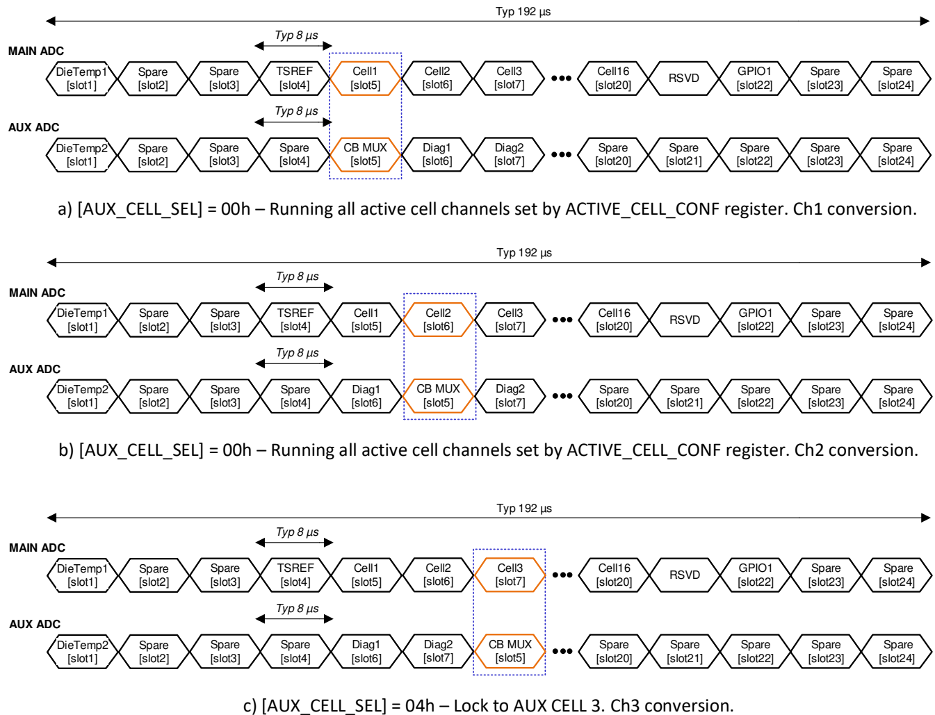
Figure 8-11. Synchronization between MAIN and AUX ADC Sampling
