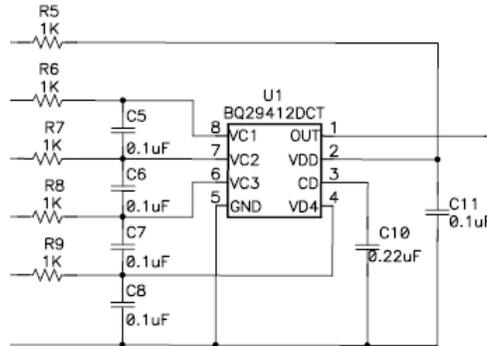
Figure 22. bq29705 Cell Inputs and Time-Delay Capacitor
