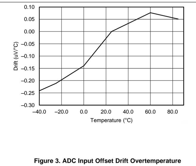
Figure 3. ADC Input Offset Drift Overtemperature
