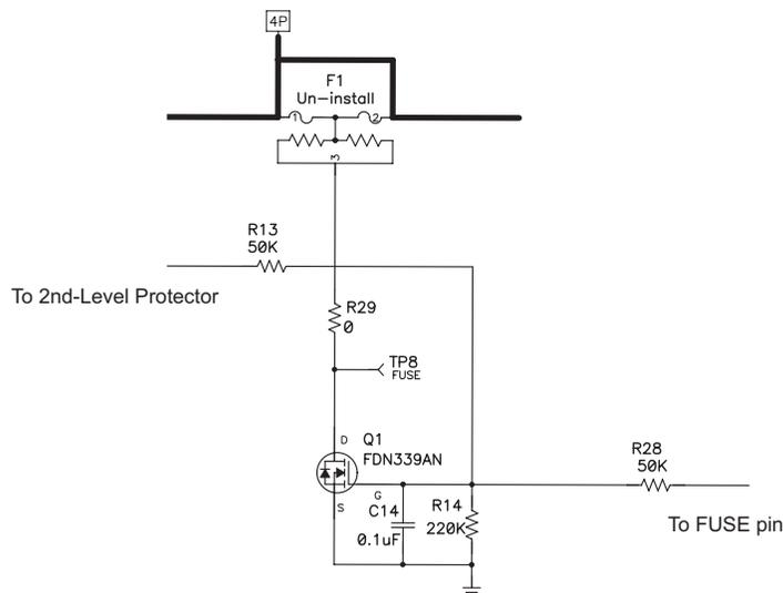
Figure 16. FUSE Circuit
