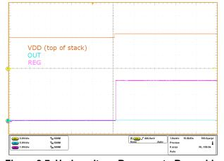
Figure 8-7. Undervoltage Recovery to Re-enable the Regulator
