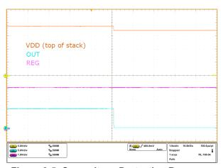
Figure 8-5. Overvoltage Protection Recovery
