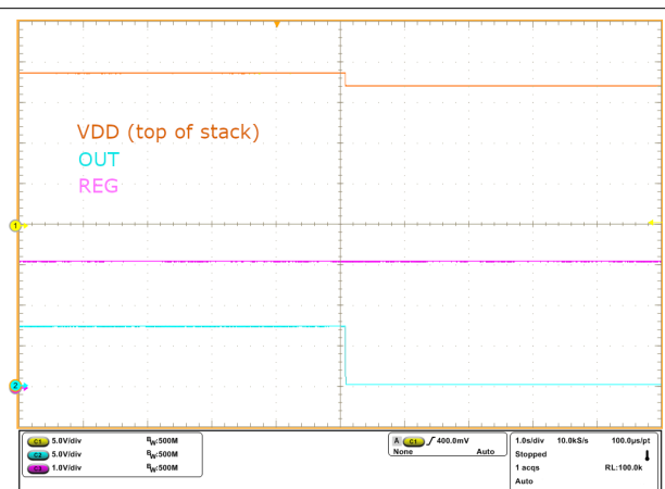
Figure 8-5. Overvoltage Protection Recovery
