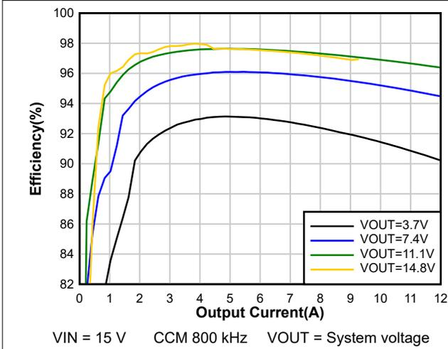
Figure 8-3. System Efficiency
