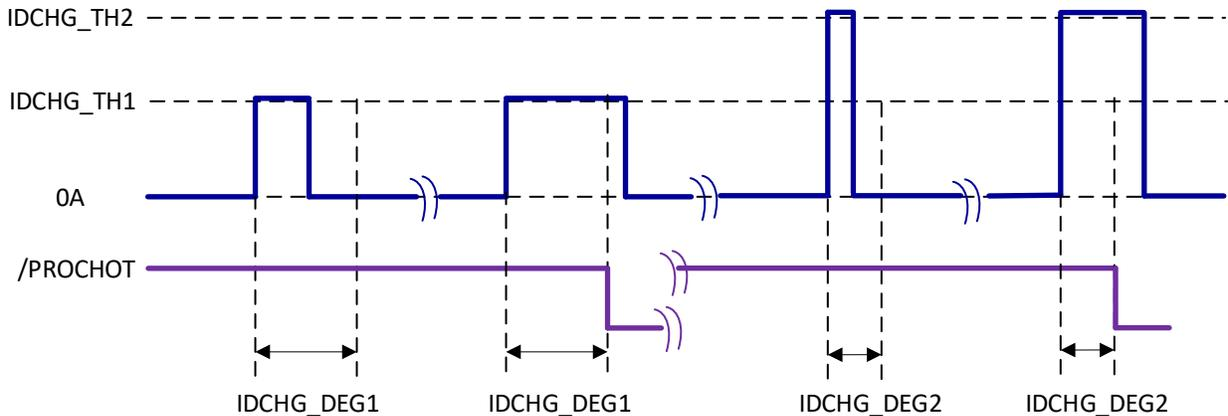
Figure 9-1. Two-Level Battery Discharging Current Trigger  $\overline{\text{PROCHOT}}$  Diagram
