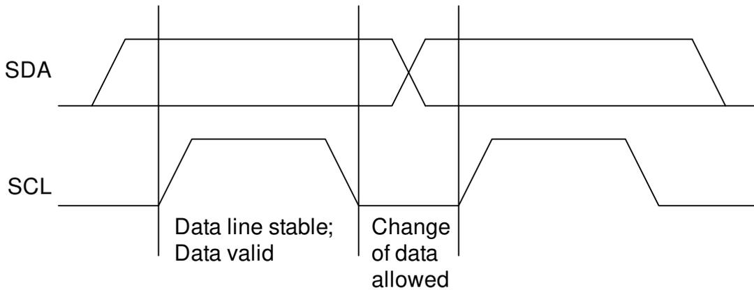
Figure 9-8. Bit Transfer on the I<sup>2</sup>C Bus
