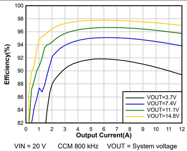
Figure 8-4. System Efficiency
