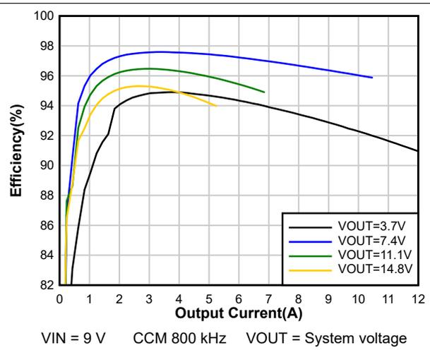
Figure 8-2. System Efficiency
