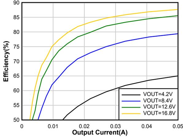
VIN = 20 V EN\_OOA = 0b VOUT = System voltage
