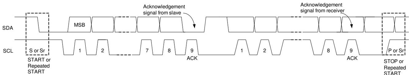
**Figure 9-10. Data Transfer on the I<sup>2</sup>C Bus**
