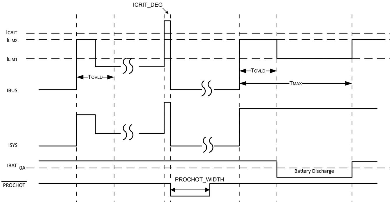
Figure 9-3. Two-Level Adapter Current Limit Timing Diagram
