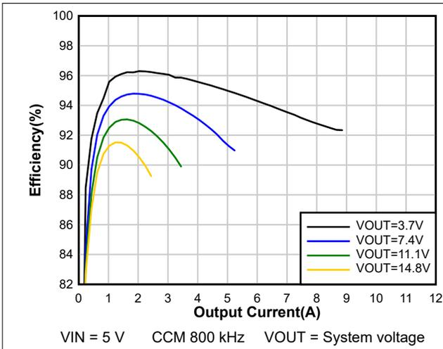
Figure 8-1. System Efficiency
