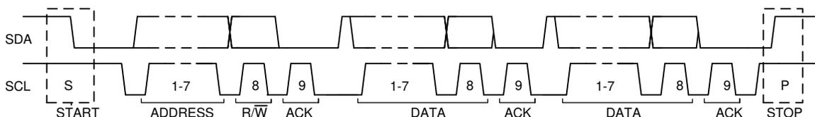
**Figure 8-10. Complete Data Transfer on the I<sup>2</sup>C Bus**
