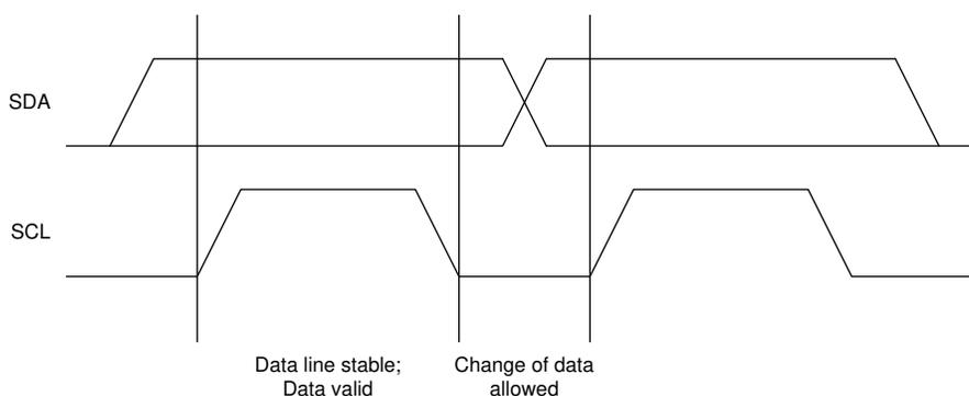
**Figure 8-7. Bit Transfer on the I<sup>2</sup>C Bus**
