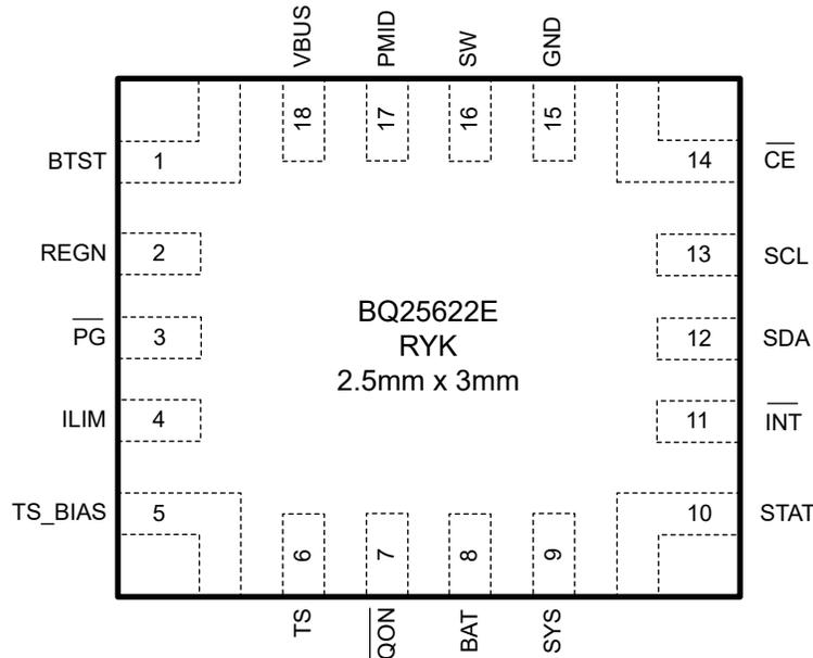
**Figure 6-1. BQ25622E Pinout, 18-Pin WQFN Top View**
