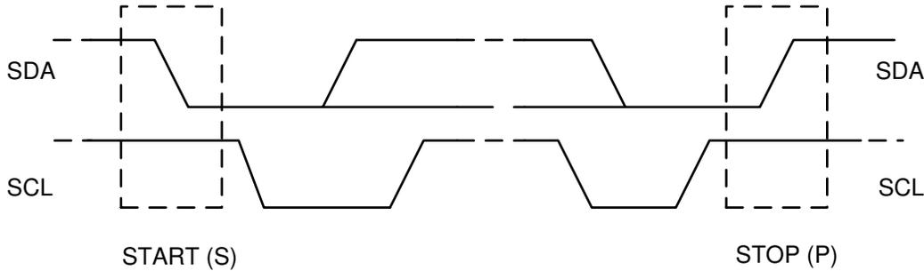
**Figure 8-8. START and STOP Conditions on the I<sup>2</sup>C Bus**
