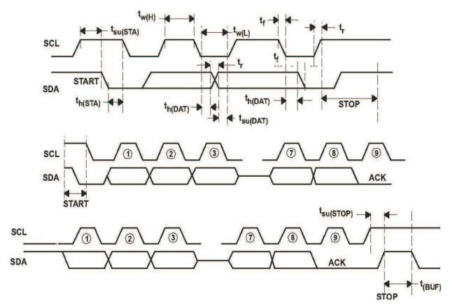
Figure 3. SMBus Communication Timing Waveforms
