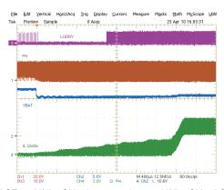
CH1: PHASE, 20V/div, CH2: battery voltage, 5V/div, CH3: LODRV, 10V/div, CH4: inductor current, 2A/div, 400us/div
