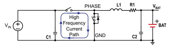
Figure 24. High Frequency Current Path
