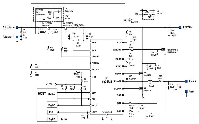
$F_s = 750 \text{kHz}$ ,  $I_{ADPT} = 4.096 \text{A}$ ,  $I_{CHRG} = 2.944 \text{A}$ ,  $I_{LIM} = 4 \text{A}$ ,  $V_{CHRG} = 12.592 \text{V}$ , 90W adapter and 3S2P battery pack See the application information about negative output voltage protection for hard shorts on battery to ground or battery reverse connection.
