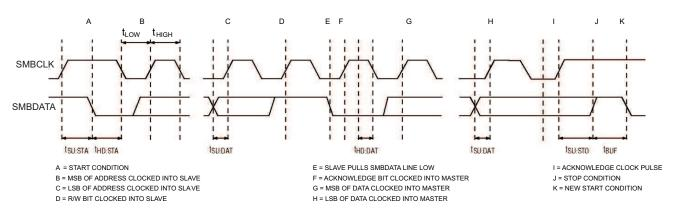
Figure 19. SMBus Read Timing
