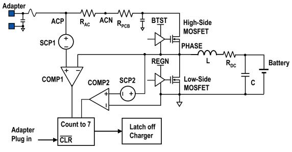
Figure 21. Block Diagram of bq24725 Short Circuit Protection
