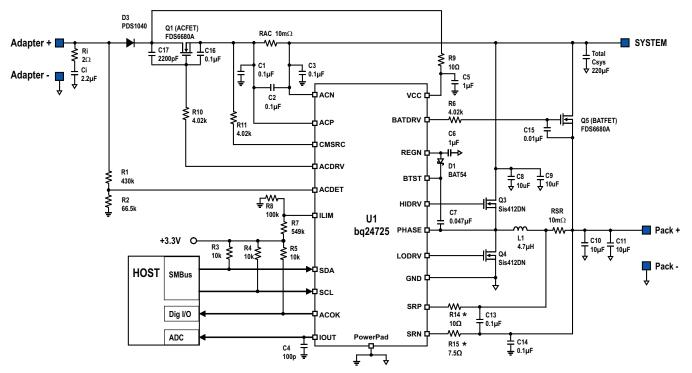
$F_s = 750 \text{kHz}$ ,  $I_{ADPT} = 2.688 \text{A}$ ,  $I_{CHRG} = 1.984 \text{A}$ ,  $I_{LIM} = 2.54 \text{A}$ ,  $V_{CHRG} = 12.592 \text{V}$ , 65W adapter and 3S2P battery pack See the application information about negative output voltage protection for hard shorts on battery to ground or battery reverse connection.
