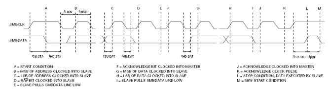
Figure 18. SMBus Write Timing
