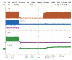
CH1: PHASE, 20V/div, CH2: LODRV, 10V/div, CH3: battery voltage, 5V/div, CH4: inductor current, 2A/div, 2ms/div Figure 13. Battery to Ground Short Protection
