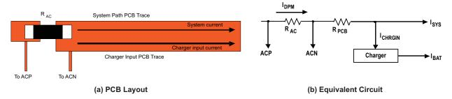
Figure 22. Need improve PCB layout example.
