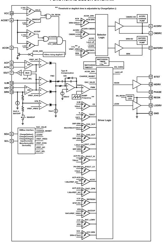
Figure 16. Functional Block Diagram for bq24725
