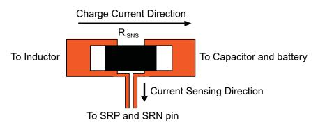
Figure 25. Sensing resistor PCB layout.
