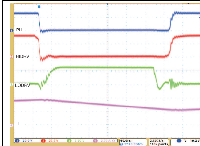
Figure 3. Current Soft Start (CE = HIGH)
