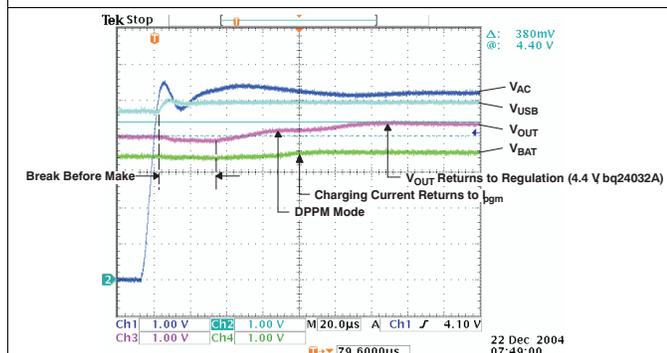
Figure 12. Apply AC – PWR XFER From USB to AC
