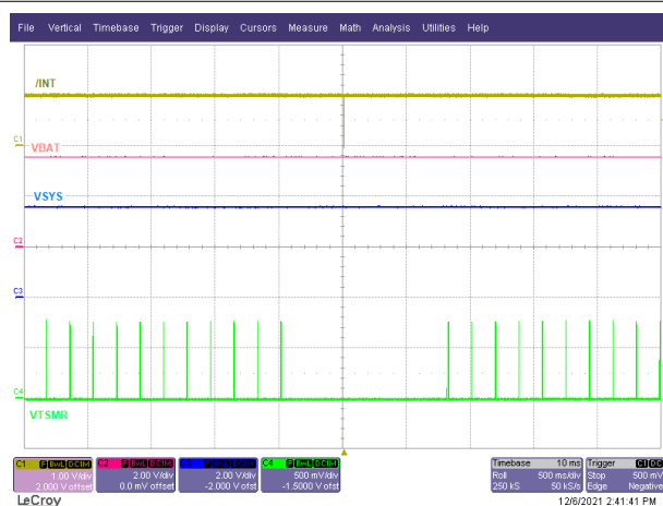
Figure 9-18. Wake1 Interrupt without VIN
