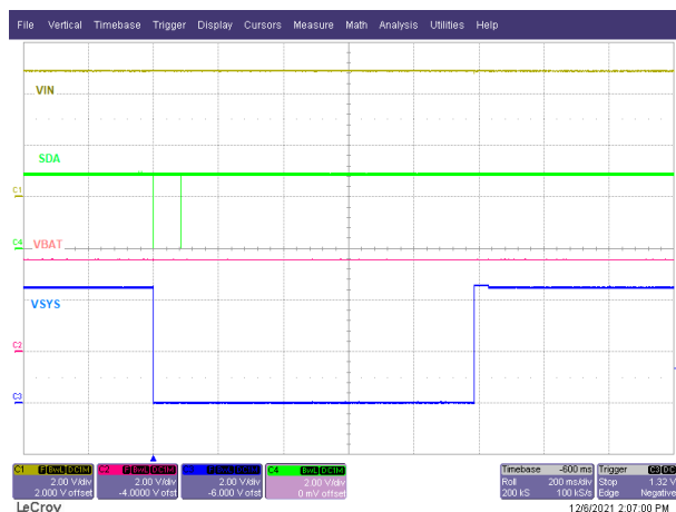
Figure 9-8. Hardware Reset Through I 2 C
