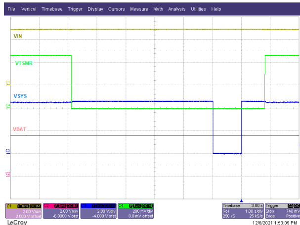
Figure 9-6. Hardware Reset with /TSMR Press
