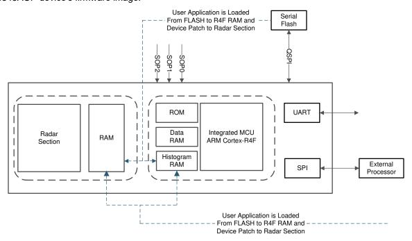
Figure 8-8. Bootloader's Functional Mode
