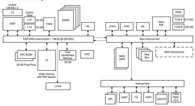
Figure 8-5. Processor Subsystem
