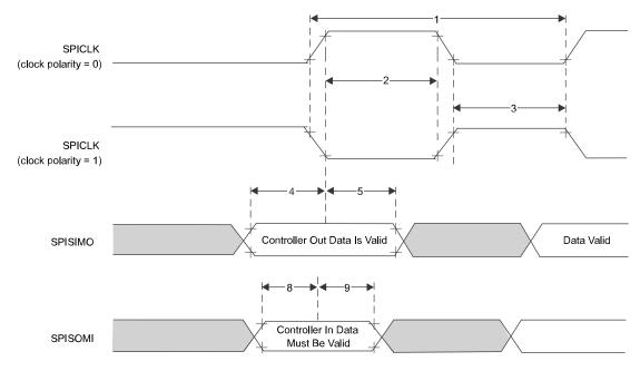
Figure 7-9. SPI Controller Mode External Timing (CLOCK PHASE = 1)
