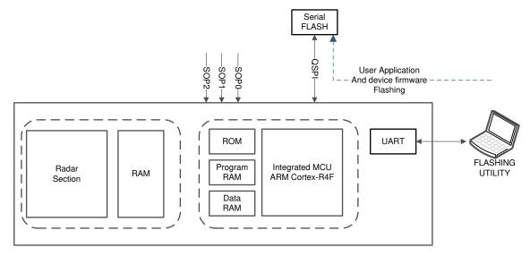
Figure 8-7. Figure 5. Bootloader Flashing Mode
