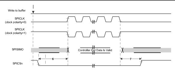
Figure 7-10. SPI Controller Mode Chip Select Timing (CLOCK PHASE = 1)
