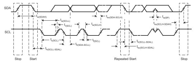
Figure 7-16. I2C Timing Diagram
