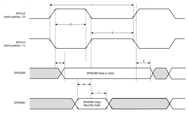
Figure 7-11. SPI Peripheral Mode External Timing (CLOCK PHASE = 0)
