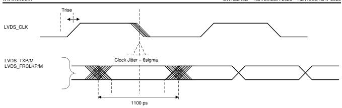
Figure 7-15. Timing Parameters
