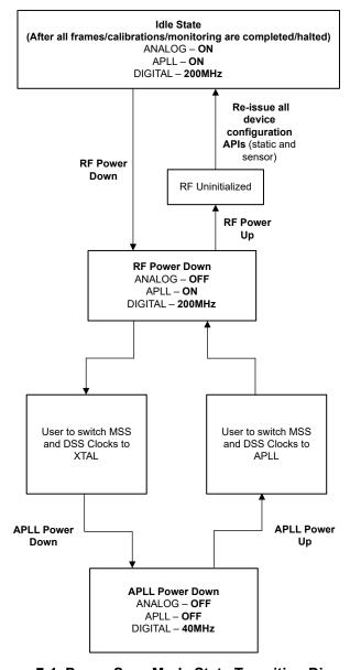
Figure 7-1. Power Save Mode State Transition Diagram
