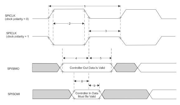
Figure 7-7. SPI Controller Mode External Timing (CLOCK PHASE = 0)
