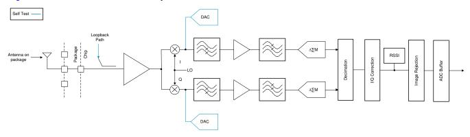
Figure 8-4. Receive Subsystem (Per Channel)
