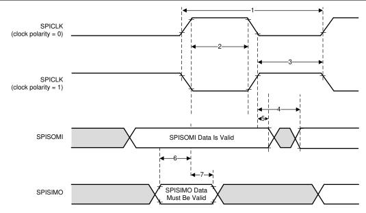
Figure 7-12. SPI Peripheral Mode External Timing (CLOCK PHASE = 1)
