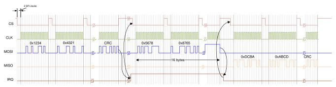
Figure 7-13. SPI Communication
