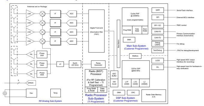
Figure 4-1. Functional Block Diagram
