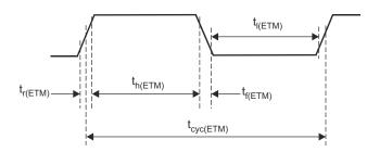
Figure 7-19. ETMTRACECLKOUT Timing
