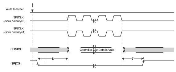
Figure 7-8. SPI Controller Mode Chip Select Timing (CLOCK PHASE = 0)
