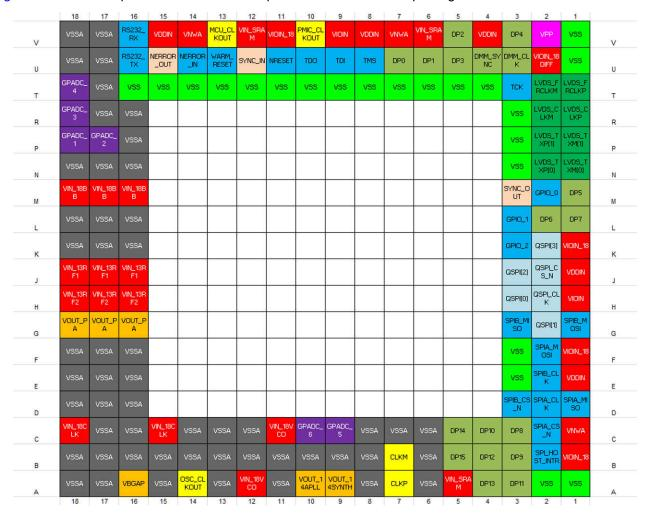
Figure 6-1. Pin Diagram (Top View)
