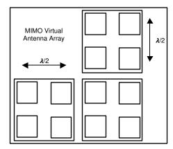
Figure 7-4. Antenna Positions (Placement and Relative Spacing)
