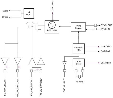
$<sup>^{\</sup>star}$  These pins are 20GHz LO input pins. Connect LO to one pin while grounding the other pin.
