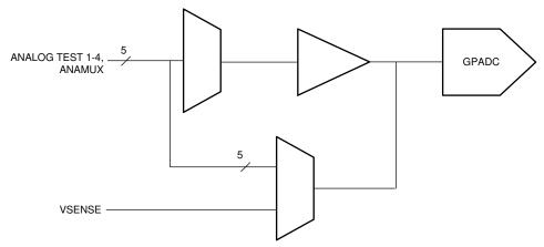
A. GPADC structures are used for measuring the output of internal temperature sensors. The accuracy of these measurements is ±7°C.
