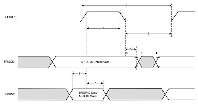
Figure 7-5. SPI Slave Mode External Timing
