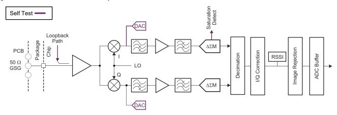
Figure 8-3. Receive Subsystem (Per Channel)
