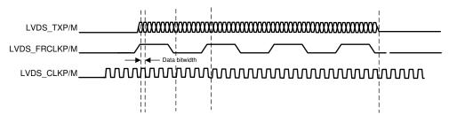
Figure 7-8. LVDS Interface Lane Configuration And Relative Timings
