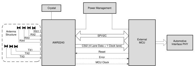
Figure 2-1. Radar Sensor for Automotive Applications
