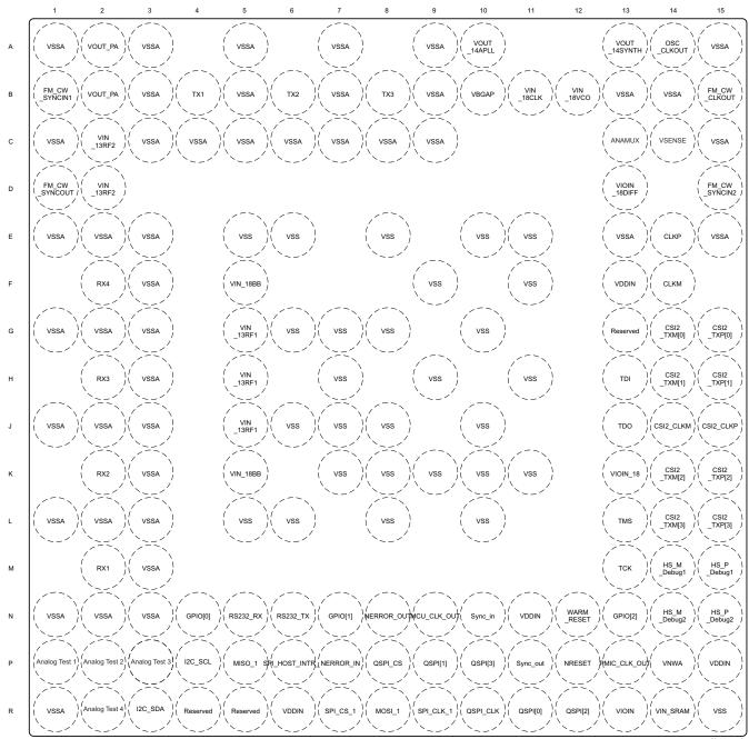
Figure 6-1. Pin Diagram
