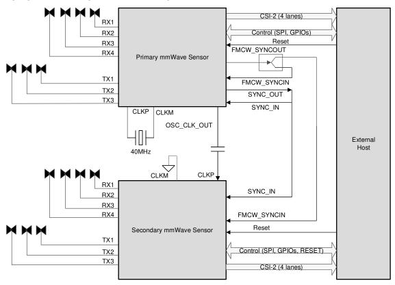
Figure 10-2. Imaging Radar using Cascade Configuration
