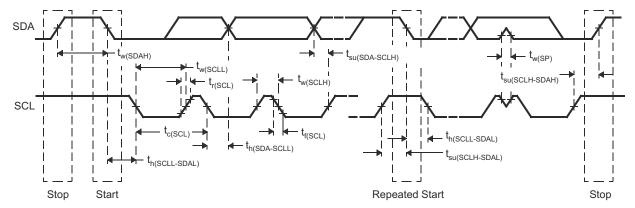
Figure 7-7. I2C Timing Diagram
