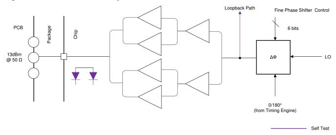
Figure 8-2. Transmit Subsystem (Per Channel)
