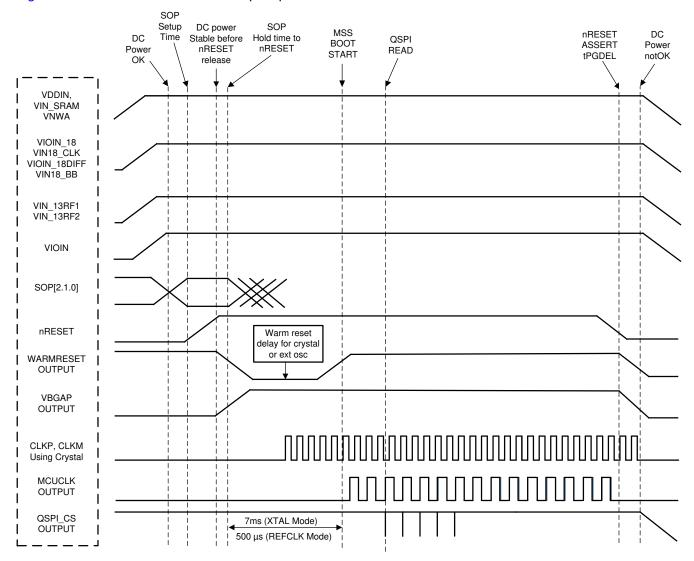
Figure 7-2. Device Wake-up Sequence
