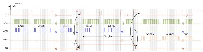
Figure 7-6. SPI Communication
