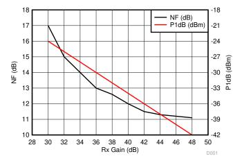
Figure 7-1. Noise Figure, In-band P1dB vs Receiver Gain
