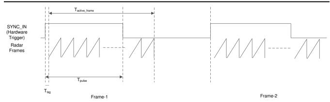
Figure 7-3. Sync In Hardware Trigger
