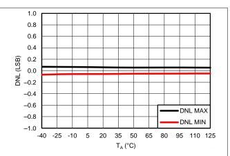
Figure 15. DAC Linearity Error vs Temperature DAC Range: 0 to 5 V
