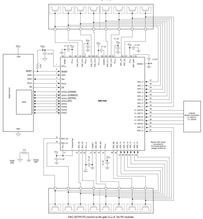
Figure 118. AMC7836 Example Schematic
