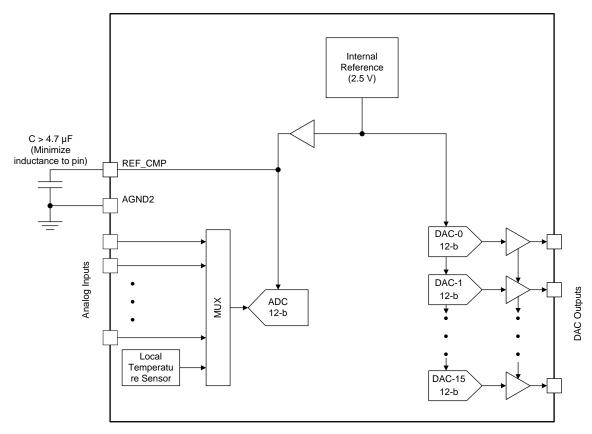
Figure 58. AMC7836 Internal Reference
