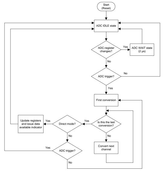
Figure 52. ADC Conversion Sequence
