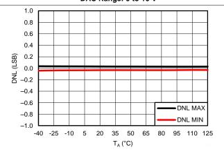
Figure 13. DAC Linearity Error vs Temperature DAC Range: -10 to 0 V
