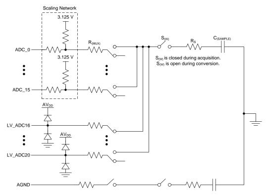
Figure 51. ADC External Inputs Equivalent Circuit
