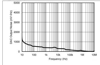
Figure 27. DAC Output Noise vs Frequency
