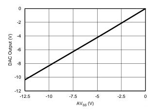
Figure 50. DAC Clamp Output vs AV<sub>SS</sub>
