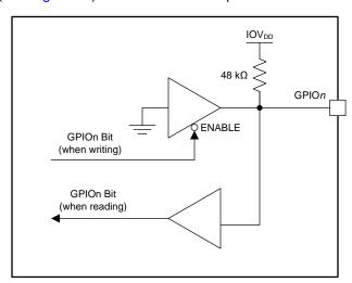
Figure 60. AMC7836 GPIO Pin
