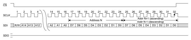
Figure 63. Serial Interface Streaming Write Example
