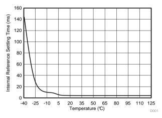
Figure 59. Internal Reference Settling Time vs Temperature
