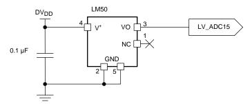
Figure 116. Temperature Sensing Application With LM50
