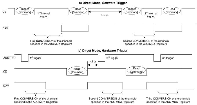
Figure 53. ADC Direct-Mode Trigger Synchronization
