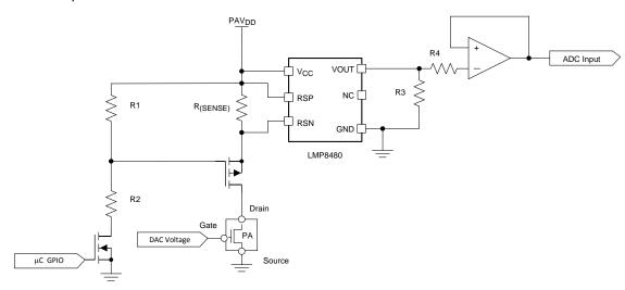
Figure 117. Current-Sense Application With PMOS ON and OFF
