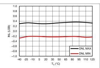
Figure 42. ADC Linearity Error vs Temperature Bipolar Input
