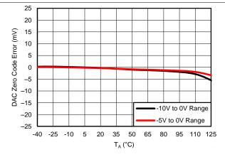
Figure 19. DAC Offset Error vs Temperature
