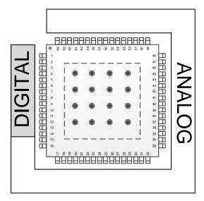
Figure 122. AMC7836 Example Board Layout — Component Placement
