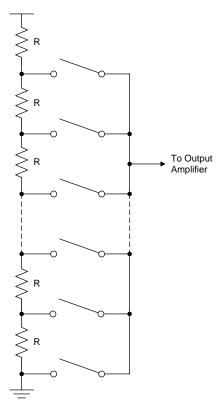
Figure 48. DAC Resistor String
