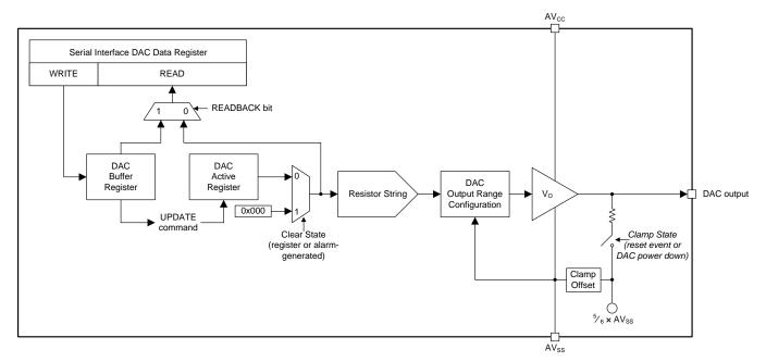
Figure 49. DAC Block Diagram
