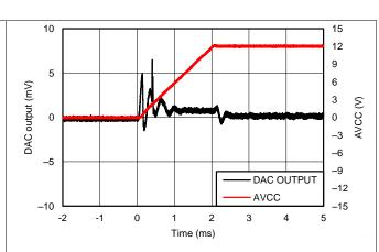
$AV_{SS} = AV_{EE} = AGND$ ,  $AV_{CC} = 0$  to 12 V, 2-ms ramp
