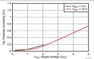
Figure 7-5. Trip Threshold Sensitivity to VDD1 Ripple Voltage (Cmp1, f<sub>RIPPLE</sub> = 10kHz)
