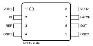
Figure 4-1. D Package, 8-Pin SOIC (Top View)
