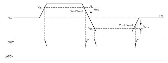
Figure 6-1. Switching Thresholds and Hysteresis
