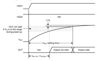
Figure 6-2. Output Behavior for Long Settling Times of the Reference Voltage
