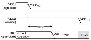
Figure 6-7. VDD2 Turns On, Followed by VDD1 (Short Delay)
