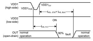
Figure 6-13. Output Response to a Power-Loss Event on VDD1
