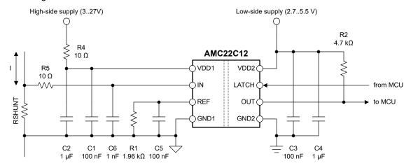
Figure 7-6. Decoupling of the AMC22C12
