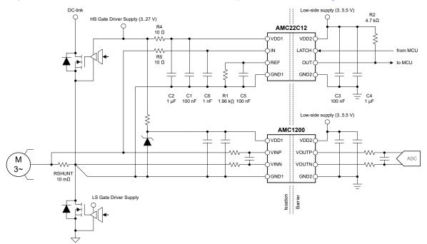
Figure 7-1. Using the AMC22C12 for Overcurrent Detection
