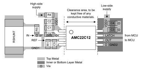
Figure 7-7. Recommended Layout of the AMC22C12
