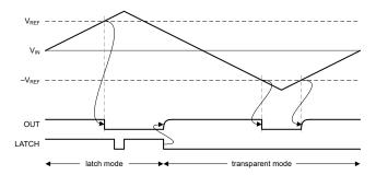
Figure 5-2. Functional Timing Diagram
