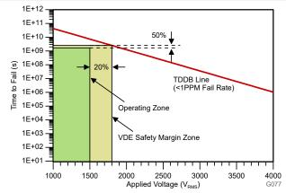
$T_A$  up to 150°C, stress-voltage frequency = 60Hz, isolation working voltage = 1000V<sub>RMS</sub>, operating lifetime > 400 years **Figure 5-5. Basic Isolation Capacitor Lifetime Projection**
