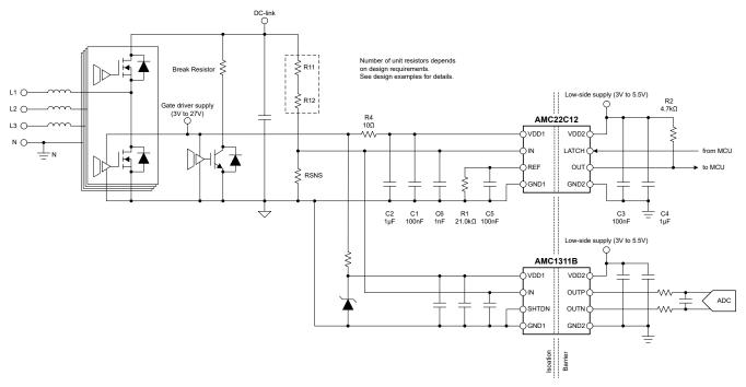
Figure 7-2. Using the AMC22C12 for Overvoltage Detection
