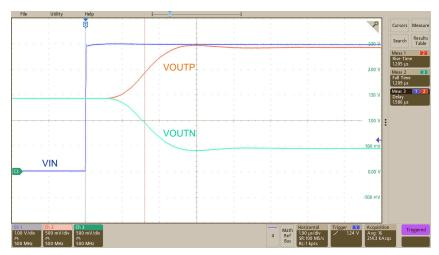
Figure 8-4. Step Response of the AMC1351
