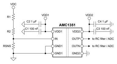
Figure 9-1. Decoupling of the AMC1351
