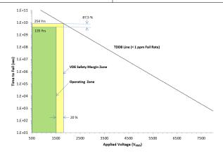
$T_A$  up to 150°C, stress-voltage frequency = 60 Hz, isolation working voltage = 1500  $V_{RMS}$ , operating lifetime = 135 years
