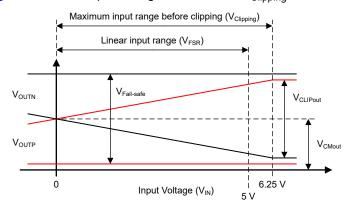
Figure 7-2. Output Behavior of the AMC1351
