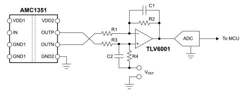
Figure 8-3. Connecting the AMC1351 Output to a Single-Ended Input ADC
