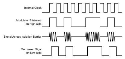
Figure 7-1. OOK-Based Modulation Scheme
