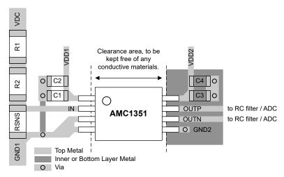
Figure 10-1. Recommended Layout of the AMC1351
