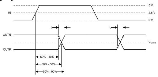
Figure 6-1. Rise, Fall, and Delay Time Definition
