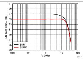
Figure 22. Signal-to-Noise Ratio and Signal-to-Noise + Distortion vs Input Signal Frequency
