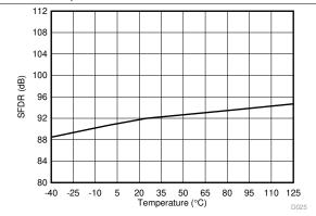
Figure 30. Spurious-Free Dynamic Range vs Temperature
