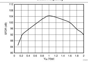
Figure 33. Spurious-Free Dynamic Range vs Input Signal Amplitude
