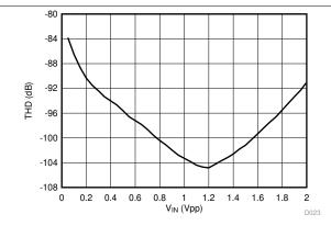
Figure 28. Total Harmonic Distortion vs Input Signal Amplitude
