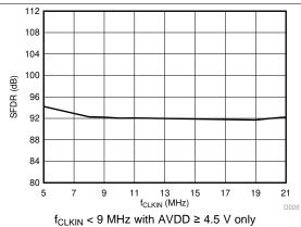
Figure 31. Spurious-Free Dynamic Range vs Clock Frequency
