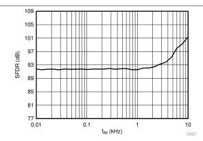
Figure 32. Spurious-Free Dynamic Range vs Input Signal Frequency
