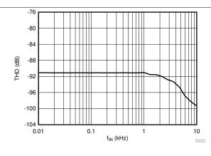
Figure 27. Total Harmonic Distortion vs Input Signal Frequency
