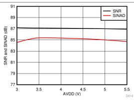
Figure 19. Signal-to-Noise Ratio and Signal-to-Noise +
