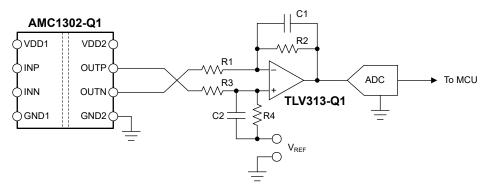
Figure 8-3. Connecting the AMC1302-Q1 Output to a Single-Ended Input ADC
