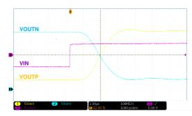
Figure 8-4. Step Response of the AMC1302-Q1
