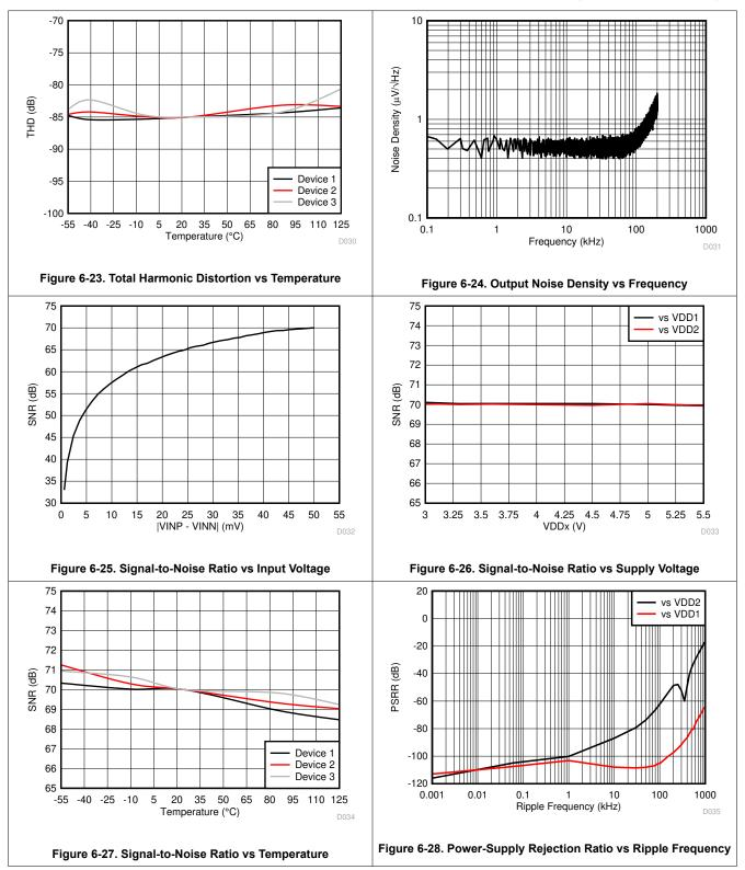
at  $T_A = 25$ °C, VDD1 = 5 V, VDD2 = 3.3 V, INP = -50 mV to 50 mV, INN = GND1, and  $f_{IN} = 10$  kHz (unless otherwise noted)
