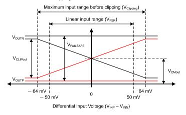
Figure 7-2. Output Behavior of the AMC1302-Q1
