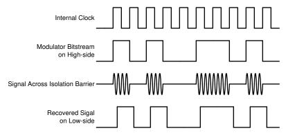
Figure 7-1. OOK-Based Modulation Scheme
