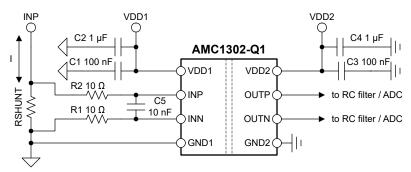
Figure 9-1. Decoupling of the AMC1302-Q1
