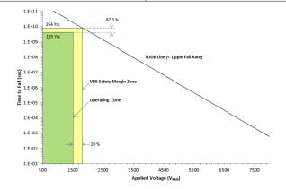
$T_{A} \ up \ to \ 150 ^{\circ}C, \ stress-voltage \ frequency = 60 \ Hz, \ isolation \ working \ voltage = 1500 \ V_{RMS}, \ operating \ lifetime = 135 \ years$
