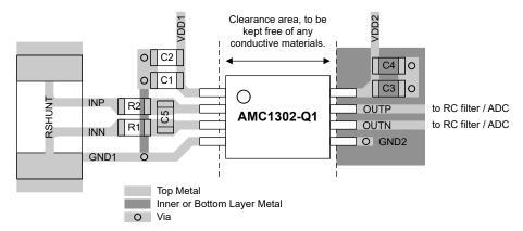
Figure 10-1. Recommended Layout of the AMC1302-Q1
