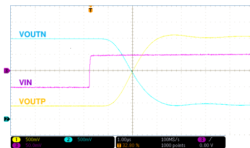
Figure 8-4. Step Response of the AMC1302
