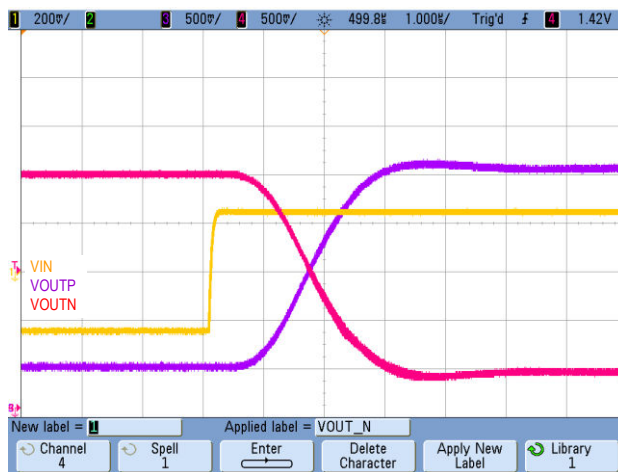
Figure 8-4. Step Response of the AMC1301
