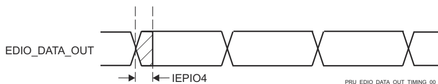
Figure 7-111. PRUSS IEP Digital IOs Timing Requirements
