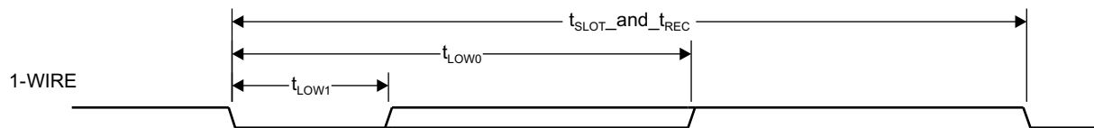
Figure 5-118. 1-Wire Write Bit Timing (Command/Address or Data)
