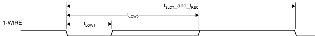
Figure 5-118. 1-Wire Write Bit Timing (Command/Address or Data)
