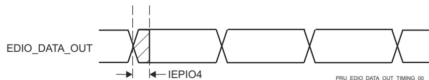
Figure 6-54. PRU-ICSS IEP Digital IOs Timing Requirements
