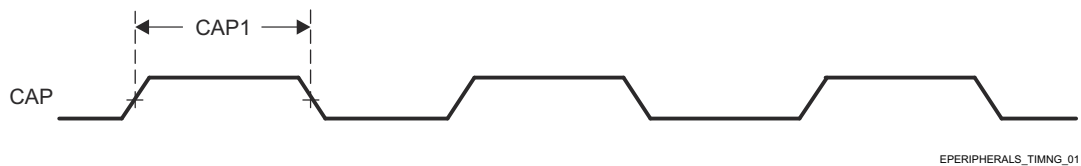
Figure 6-16. ECAP Timings Requirements
