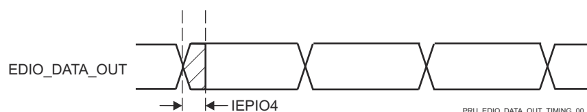
Figure 6-76. PRU-ICSS IEP Digital IOs Timing Requirements
