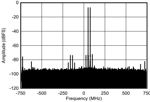
Figure 4-444. RX Dual Tone Output FFT at 8.11GHz
