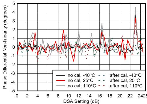
Figure 4-452. RX Phase Differential Non-linearity at 9.6 GHz
