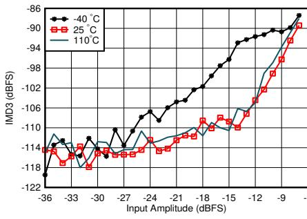
With 0.8 GHz matching, tone spacing = 20 MHz, DSA = 4 dB
