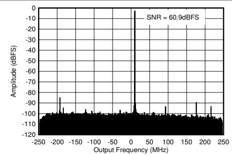
With 1.8 GHz matching,  $f_{\text{IN}} = 2610 \text{ MHz}$ ,  $A_{\text{IN}} = -3 \text{ dBFS}$
