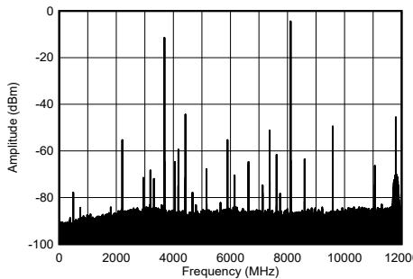
**Figure 4-203. TX Single Tone Output Spectrum at 8.11 GHz**
