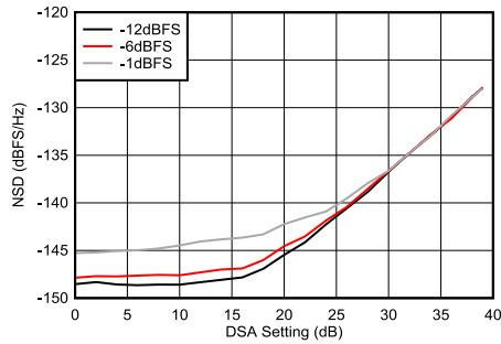
Figure 4-261. TX NSD vs DSA Setting at 9.61 GHz
