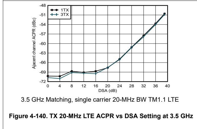
Figure 4-140. TX 20-MHz LTE ACPR vs DSA Setting at 3.5 GHz
