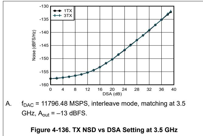
Figure 4-136. TX NSD vs DSA Setting at 3.5 GHz
