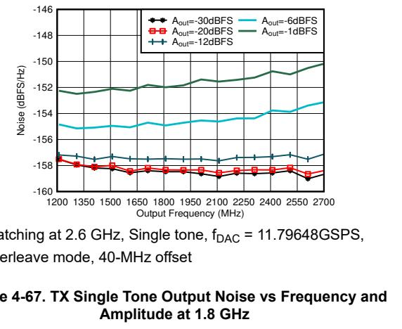
Figure 4-67. TX Single Tone Output Noise vs Frequency and Amplitude at 1.8 GHz
