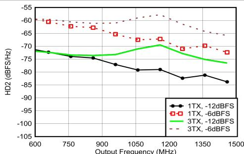
Matching at 0.8 GHz,  $f_{\text{DAC}} = 8847.36$  GSPS, straight mode
