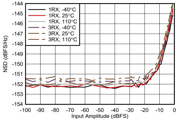
Figure 4-431. RX NSD vs Digital Amplitude at 8.11GHz
