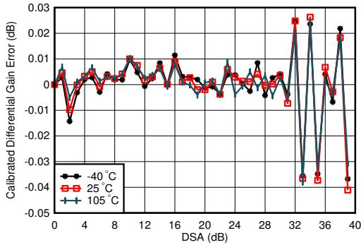
$f_{\text{DAC}} = 5898.24$  MSPS, interleave mode, matching at 0.8 GHz
