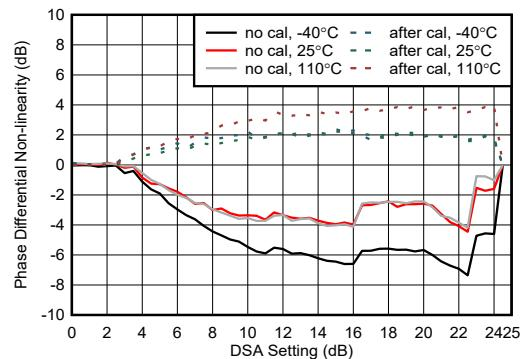
Figure 4-427. RX Phase Differential Nonlinearity at 8.1GHz
