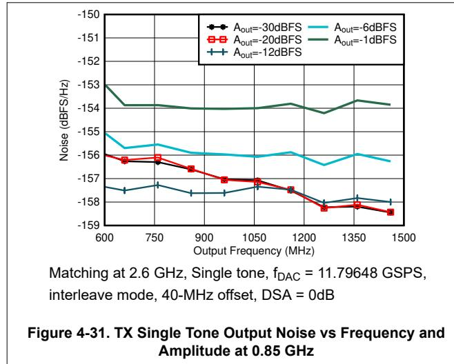
Figure 4-31. TX Single Tone Output Noise vs Frequency and Amplitude at 0.85 GHz
