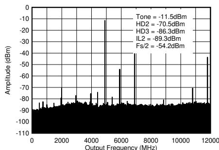
$f_{\text{DAC}} = 11796.48$  MSPS, interleave mode, 4.9 GHz matching, includes PCB and cable losses.  $\text{ILn} = f_s/n \pm f_{\text{OUT}}$ .
