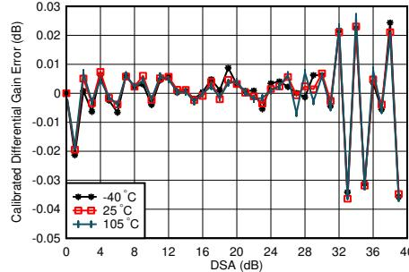
$f_{\text{DAC}} = 5898.24$  MSPS, interleave mode, matching at 1.8 GHz
