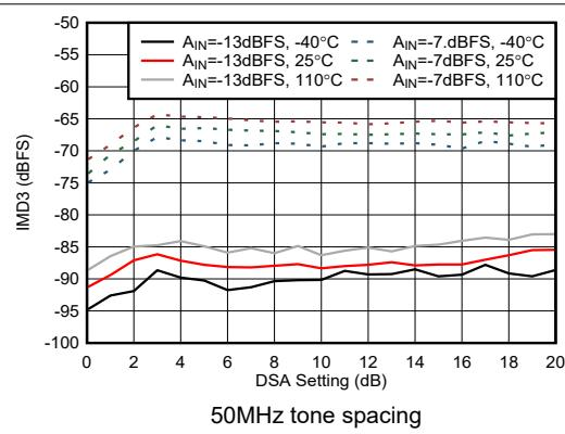
Figure 4-429. RX IMD3 vs DSA Setting at 8.11GHz
