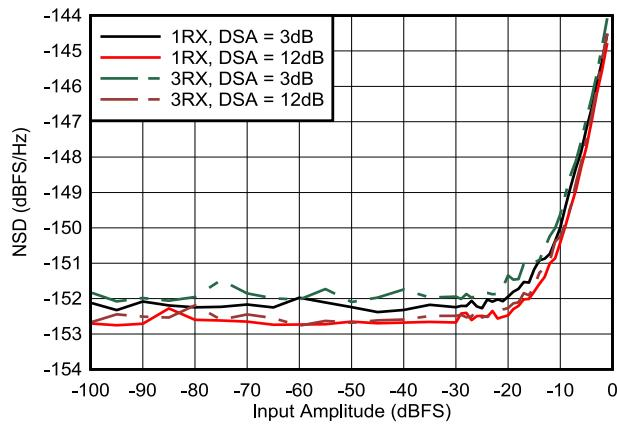
Figure 4-432. RX NSD vs Digital Amplitude at 8.11GHz
