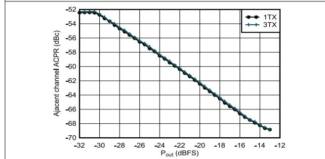
Figure 4-33. TX 20-MHz LTE ACPR vs Digital Level at 0.85 GHz
