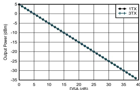
$f_{\text{DAC}} = 11796.48$  MSPS, interleave mode,  $A_{\text{out}} = -0.5$  dBFS, matching 0.8 GHz
