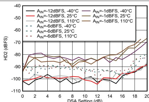
Figure 4-462. RX HD2 vs DSA Setting at 9.6 GHz
