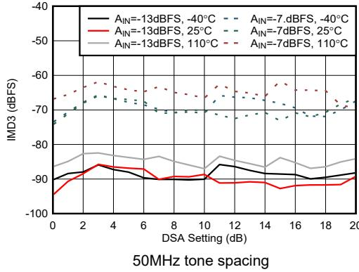
Figure 4-456. RX IMD3 vs DSA Setting at 9.6 GHz
