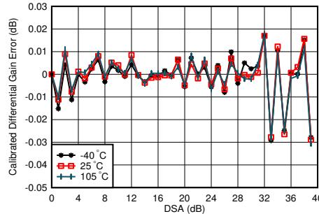
$f_{\text{DAC}} = 8847.36$  MSPS, straight mode, matching at 2.6 GHz, channel with the median variation over DSA setting at 25°C
