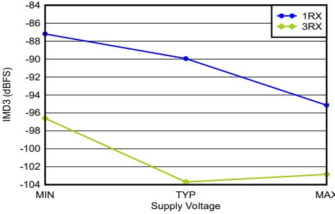
With 1.8 GHz matching, -7 dBFS each tone, 20-MHz tone spacing, all supplies at MIN, TYP, or MAX recommended operating voltages
