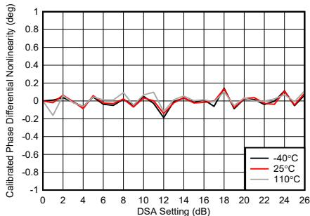
Figure 4-247. TX DSA Calibrated Phase Differential Nonlinearity
