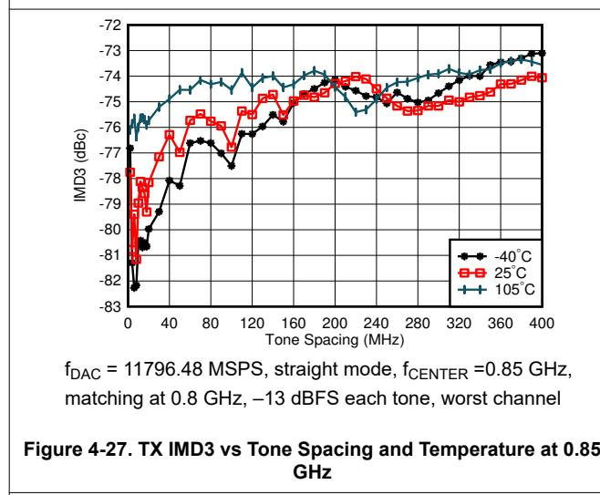
$f_{\text{DAC}} = 11796.48$  MSPS, straight mode,  $f_{\text{CENTER}} = 0.85$  GHz, matching at 0.8 GHz, -13 dBFS each tone, worst channel
