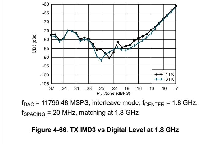
Figure 4-66. TX IMD3 vs Digital Level at 1.8 GHz
