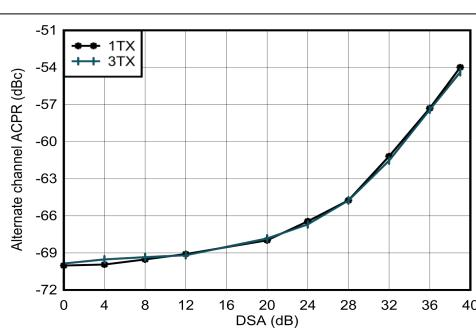
Figure 4-36. TX 20-MHz LTE alt-ACPR vs DSA at 0.85 GHz
