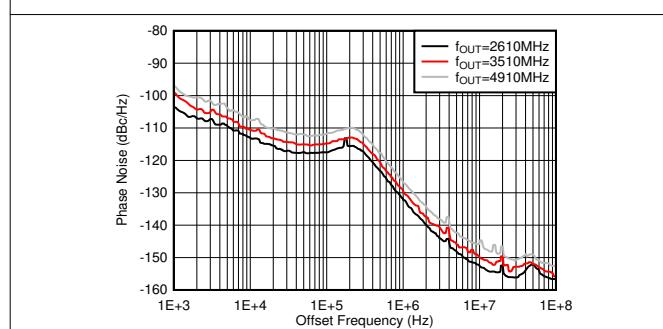
PLL enabled,  $f_{\text{VCO}} = 11796.48 \text{ MHz}$ ,  $f_{\text{REF}} = 491.52 \text{ MSPS}$ , measured at TX output
