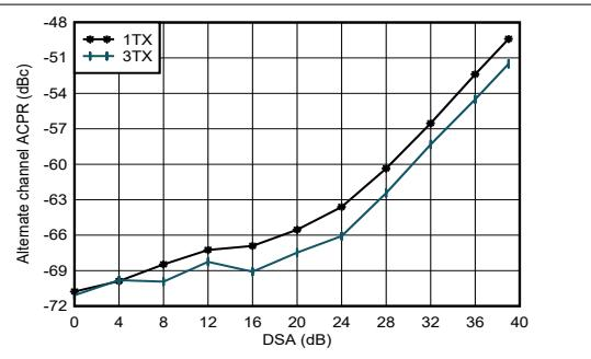
Figure 4-178. TX 20-MHz LTE alt-ACPR vs DSA at 4.9 GHz
