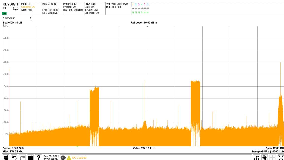
Figure 4-232. TX 4x100 MHz NR Output Spectrum 8.11 GHz
