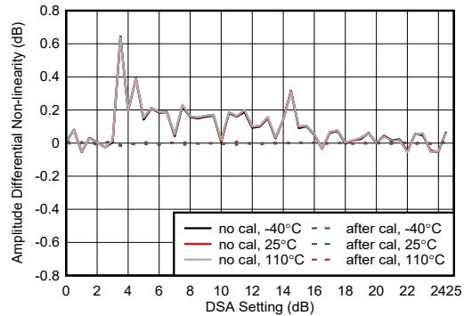
Figure 4-450. RX Amplitude Differential Non-Linearity at 9.6 GHz
