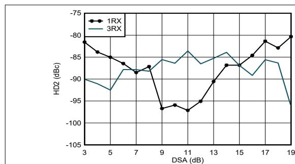
With 1.8 GHz matching,  $f_{\text{in}} = 1900 \text{ MHz}$ , measured after HD2 trim, DDC bypass mode (TI only mode for characterization)
