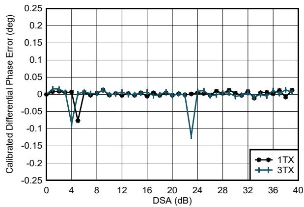
$f_{\text{DAC}} = 5898.24$  MSPS, interleave mode, matching at 0.8 GHz, channel with the median variation over DSA setting at  $25^\circ\text{C}$
