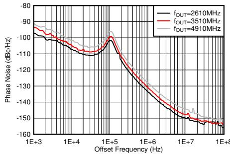
PLL enabled, f<sub>VCO</sub> = 8847.36 MHz, f<sub>REF</sub> = 491.52 MSPS, measured at TX output
