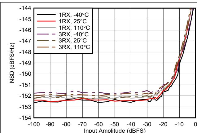
Figure 4-458. RX NSD vs Digital Amplitude at 9.6 GHz
