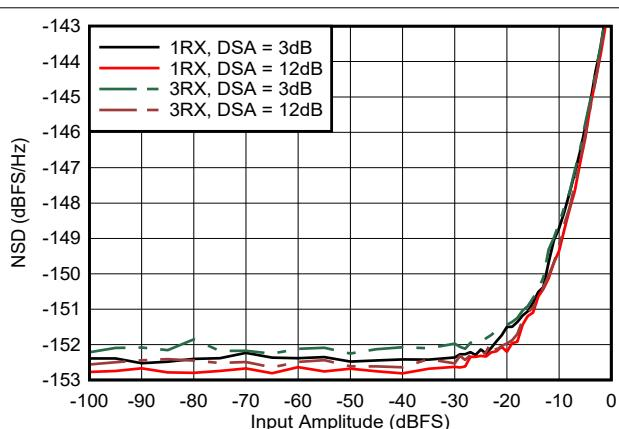
Figure 4-459. RX NSD vs Digital Amplitude at 9.6 GHz
