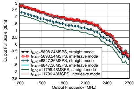
including PCB and cable losses,  $A_{\text{out}} = -0.5$  dFBS, DSA = 0, 1.8 GHz matching
