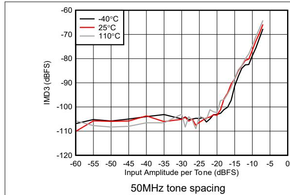
Figure 4-428. RX IMD3 vs Input Amplitude at 8.11GHz
