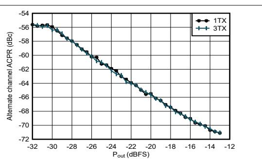
Figure 4-176. TX 20-MHz LTE alt-ACPR vs Digital Level at 4.9 GHz
