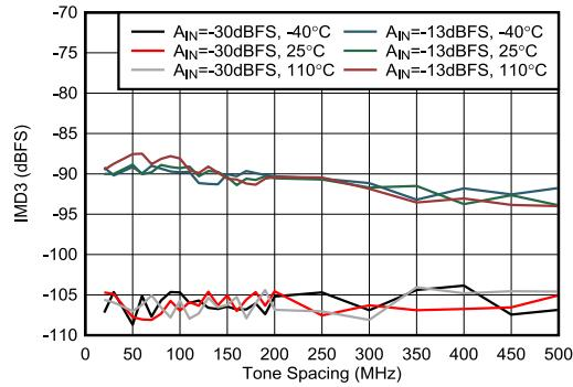
Figure 4-430. RX IMD3 vs Tone Spacing at 8.11GHz
