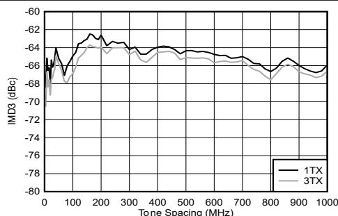
Figure 4-256. TX IMD3 vs Tone Spacing at 9.61 GHz
