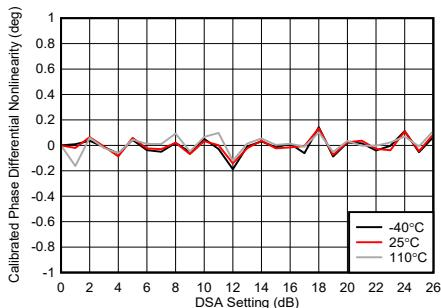
Figure 4-249. TX DSA Calibrated Phase Integrated Nonlinearity
