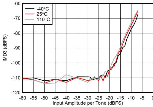
Figure 4-454. RX IMD3 vs Digital Amplitude at 9.6 GHz
