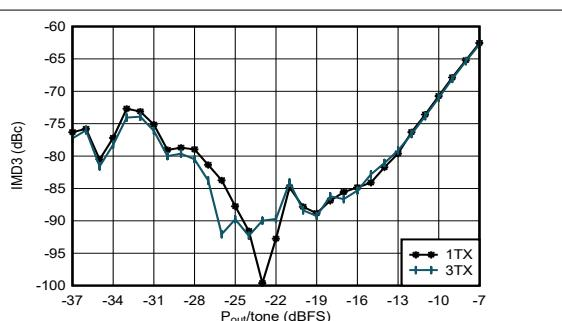
$f_{\text{DAC}} = 5898.24$  MSPS, straight mode,  $f_{\text{CENTER}} = 0.85$  GHz,  $f_{\text{SPACING}} = 20$  MHz, matching at 0.8 GHz
