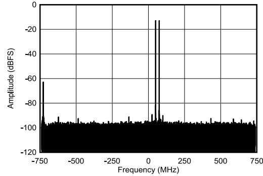
Figure 4-445. RX Dual Tone Output FFT at 8.11GHz
