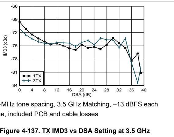
Figure 4-137. TX IMD3 vs DSA Setting at 3.5 GHz
