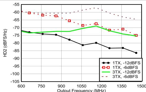
Matching at 0.8 GHz,  $f_{\text{DAC}} = 5898.24$  G SPS, straight mode
