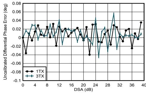
$f_{\text{DAC}} = 11796.48$  MSPS, interleaved mode, matching at 4.9 GHz
