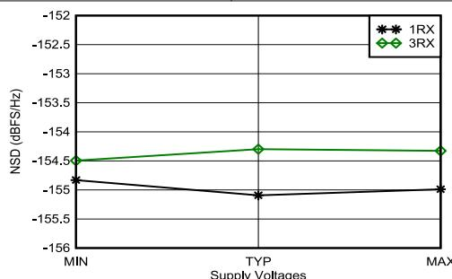
With 3.6 GHz matching, tone at -20 dBFS, 12.5-MHz offset frequency, all supplies at MIN, TYP, or MAX recommended operating voltages
