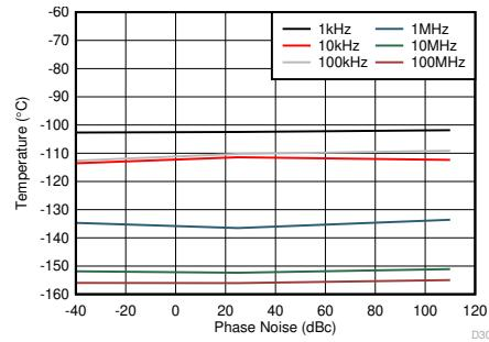
PLL enabled, f<sub>VCO</sub> = 8847.36 MHz, f<sub>REF</sub> = 491.52 MSPS, minimum LPF BW, measured at TX output
