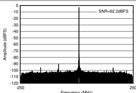
With 3.6 GHz matching,  $f_{\text{IN}} = 3610 \text{ MHz}$ ,  $A_{\text{IN}} = -3 \text{ dBFS}$
