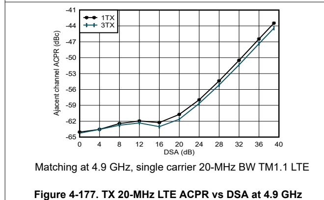
Figure 4-177. TX 20-MHz LTE ACPR vs DSA at 4.9 GHz
