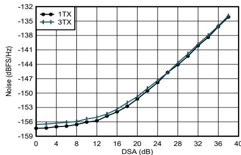
$f_{\text{DAC}} = 8847.36$  MSPS, straight mode, matching at 2.6 GHz,  $A_{\text{OUT}} = -13$  dBFS
