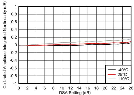
**Figure 4-243. TX DSA Calibrated Amplitude Integrated Nonlinearity**
