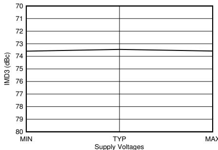
$f_{\text{DAC}} = 11796.48$  MSPS, interleave mode, 2.6 GHz matching, 40-MHz offset from tone. Output Power = -13 dBFS. All supplies simultaneously at MIN, TYP, or MAX voltages.
