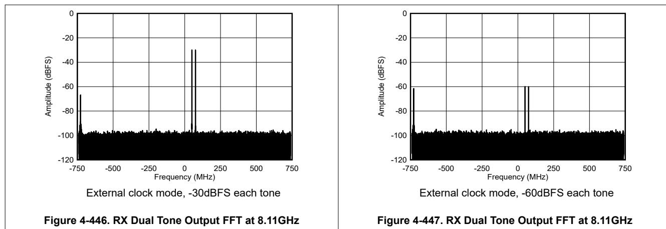
Figure 4-446. RX Dual Tone Output FFT at 8.11GHz
