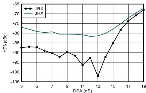
With 1.8 GHz matching,  $f_{\text{in}} = 1900 \text{ MHz}$ , DDC bypass mode (TI only mode for characterization)
