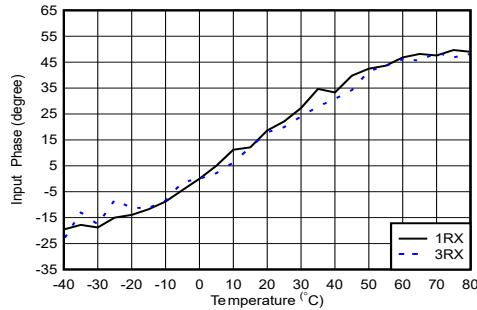
With 4.9 GHz matching, normalized to phase at  $25^\circ\text{C}$
