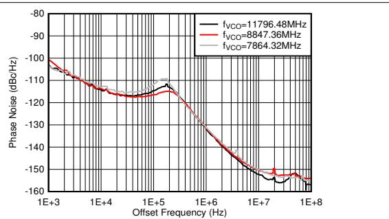
PLL enabled,  $f_{\text{REF}} = 491.52 \text{ MSPS}$ , measured at TX output
