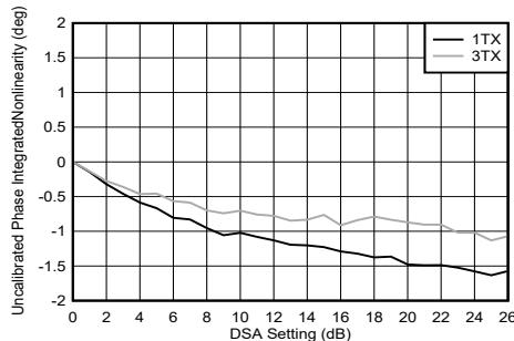
Figure 4-248. TX DSA Uncalibrated Phase Integrated Nonlinearity
