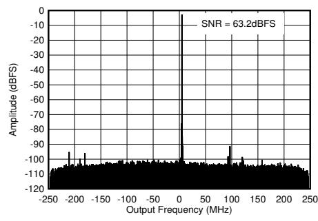
With 0.8 GHz matching,  $f_{\text{IN}} = 840$  MHz,  $A_{\text{IN}} = -3$  dBFS
