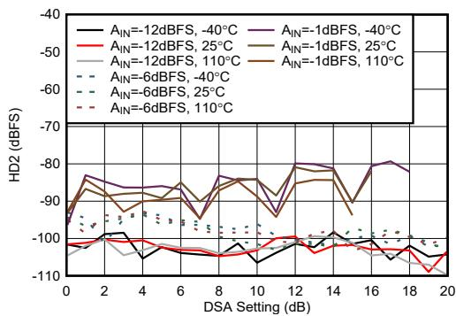
Figure 4-436. RX HD2 vs DSA Setting at 8.11GHz
