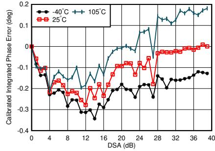
$f_{\text{DAC}} = 11796.48$  MSPS, interleaved mode, matching at 4.9 GHz, channel with the median variation over DSA setting at  $25^\circ\text{C}$
