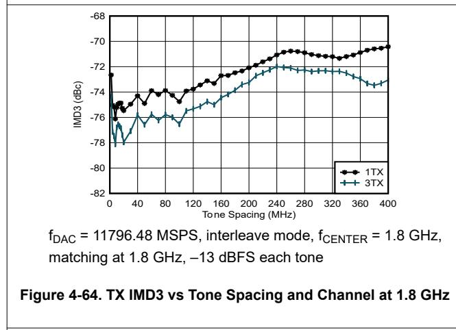
Figure 4-64. TX IMD3 vs Tone Spacing and Channel at 1.8 GHz
