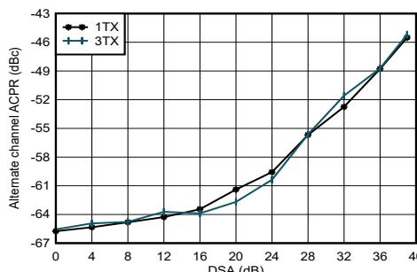
Figure 4-227. TX NR100 MHz alt-ACPR vs DSA Setting 8.11 GHz
