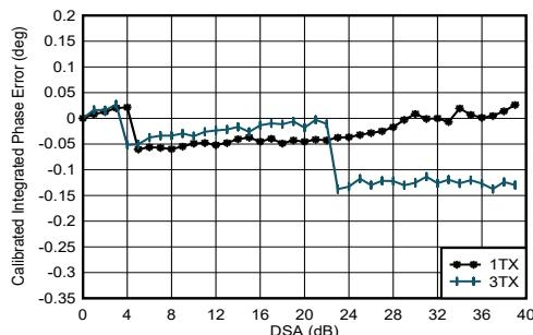
$f_{\text{DAC}} = 5898.24$  MSPS, interleave mode, matching at 0.8 GHz
