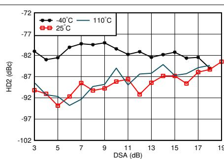
With 1.8 GHz matching,  $f_{\text{in}} = 1900 \text{ MHz}$ , measured after HD2 trim, DDC bypass mode (TI only mode for characterization)
