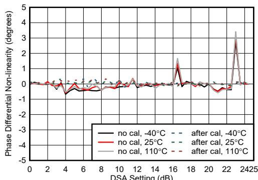
Figure 4-426. RX Phase Differential Nonlinearity at 8.11GHz
