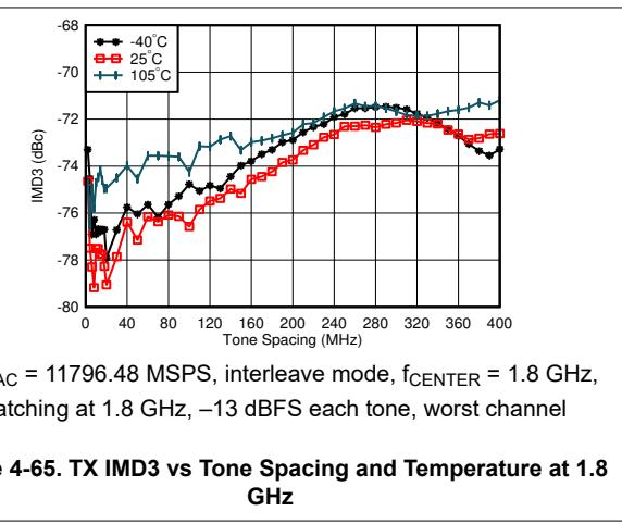
Figure 4-65. TX IMD3 vs Tone Spacing and Temperature at 1.8 GHz
