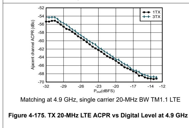
Figure 4-175. TX 20-MHz LTE ACPR vs Digital Level at 4.9 GHz
