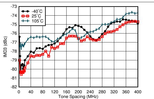
$f_{\text{DAC}} = 8847.36$  MSPS, straight mode,  $f_{\text{CENTER}} = 0.85$  GHz, matching at 0.8 GHz, -13 dBFS each tone, worst channel
