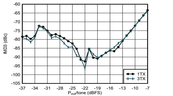
$f_{\text{DAC}} = 11796.48$  MSPS, interleave mode,  $f_{\text{CENTER}} = 0.85$  GHz,  $f_{\text{SPACING}} = 20$  MHz, matching at 0.8 GHz
