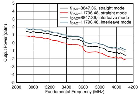
$A_{\text{out}} = -0.5$  dFBS, 3.5 GHz Matching, included PCB and cable losses
