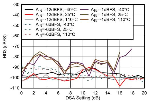
Figure 4-438. RX HD3 vs DSA Setting at 8.11GHz
