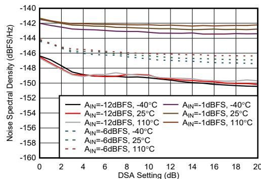
Figure 4-460. RX NSD vs DSA Setting at 9.6 GHz
