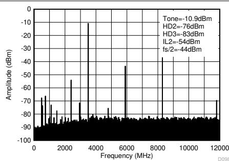
Matching at 3.5 GHz,  $f_{\text{DAC}} = 11.79648$  GSPS, interleave mode.
