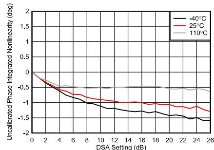
Figure 4-250. TX DSA Uncalibrated Phase Integrated Nonlinearity
