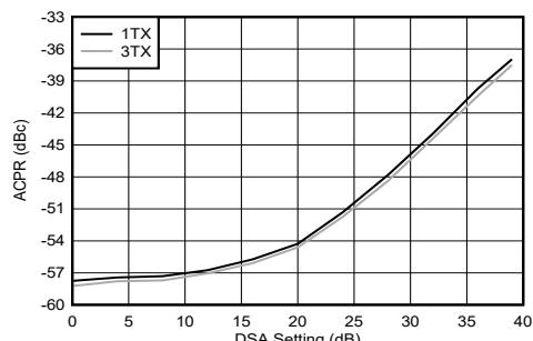
Figure 4-226. TX NR100MHz ACPR vs DSA Setting 8.11 GHz
