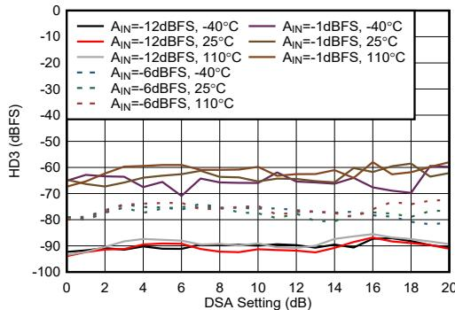
Figure 4-464. RX HD3 vs DSA Setting at 9.6 GHz
