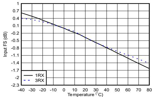
With 4.9 GHz matching, normalized to fullscale at  $25^\circ\text{C}$  for each channel
