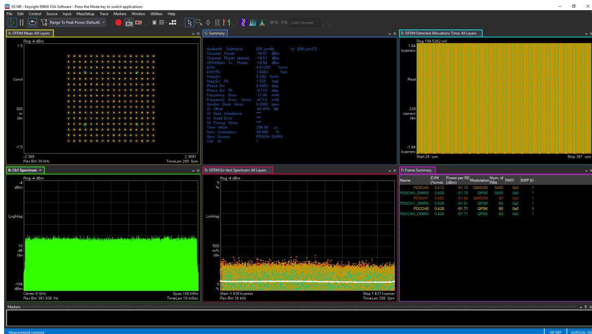
Figure 4-230. TX 100 MHz NR EVM at 8.11 GHz
