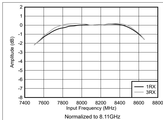
Figure 4-422. RX Amplitude vs Frequency and Channel
