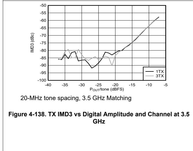
Figure 4-138. TX IMD3 vs Digital Amplitude and Channel at 3.5 GHz
