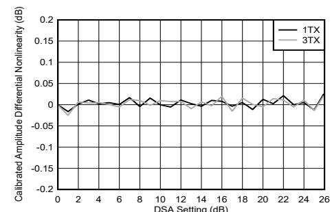
Figure 4-237. TX DSA Calibrated Amplitude Differential Nonlinearity
