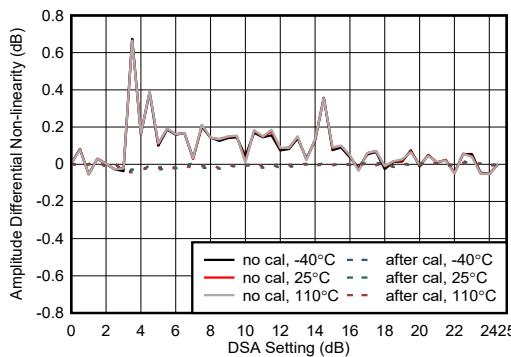
Figure 4-424. RX Amplitude Differential Nonlinearity at 8.11GHz
