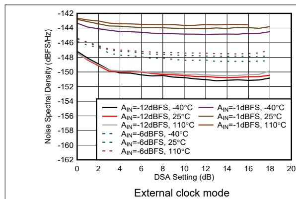
Figure 4-434. RX NSD vs DSA Setting at 8.11GHz
