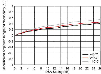
**Figure 4-242. TX DSA Uncalibrated Amplitude Integrated Nonlinearity**
