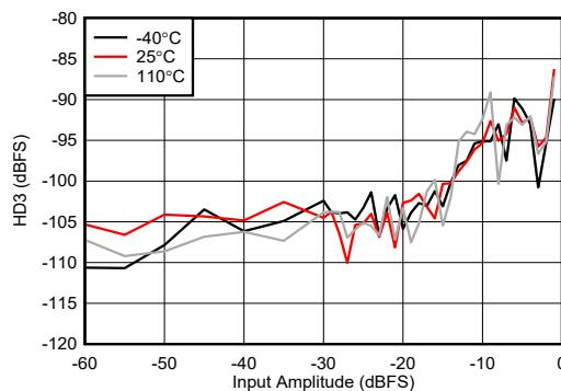
Figure 4-437. RX HD3 vs Digital Amplitude at 8.11GHz
