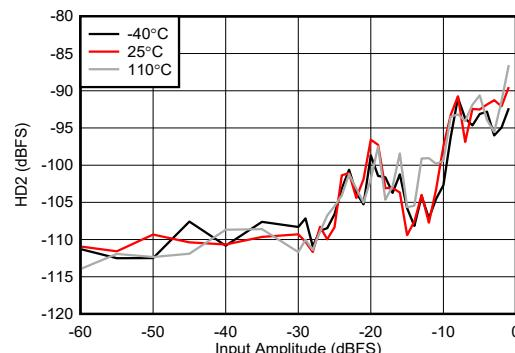
Figure 4-461. RX HD2 vs Digital Level at 9.6 GHz
