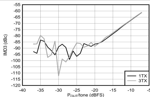
$f_{\text{DAC}} = 8847.36$  MSPS, straight mode,  $f_{\text{CENTER}} = 2.6$  GHz,
