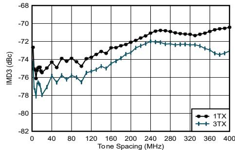
$f_{\text{DAC}} = 5898.24$  MSPS, straight mode,  $f_{\text{CENTER}} = 0.85$  GHz,
