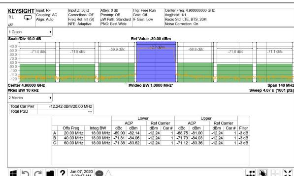
Figure 4-174. TX 20-MHz LTE Output Spectrum at 4.9 GHz
