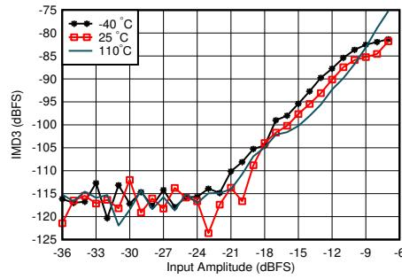
With 4.9 GHz matching, tone spacing = 20 MHz, DSA = 12 dB
