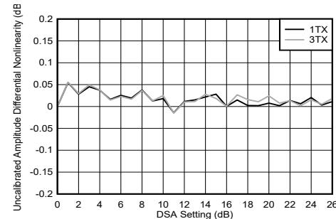
Figure 4-236. TX DSA Uncalibrated Amplitude Differential Nonlinearity
