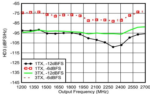
Matching at 1.8 GHz,  $f_{\text{DAC}} = 11.79648$  GSPS, interleave mode, normalized to output power at harmonic frequency
