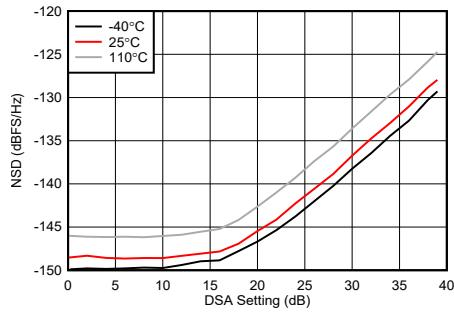
Figure 4-263. TX NSD vs DSA Setting at 9.61 GHz
