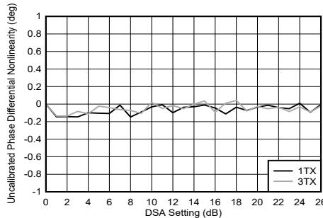
**Figure 4-244. TX DSA Uncalibrated Phase Differential Nonlinearity**
