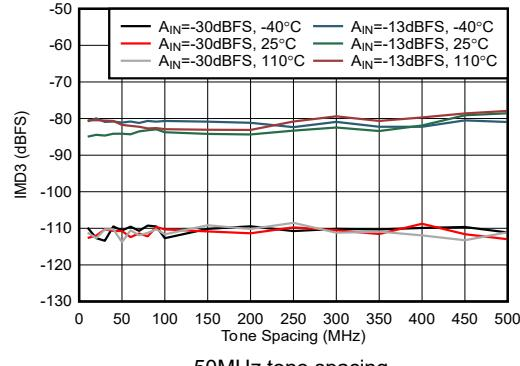
Figure 4-457. RX IMD3 vs Tone Spacing at 9.6 GHz
