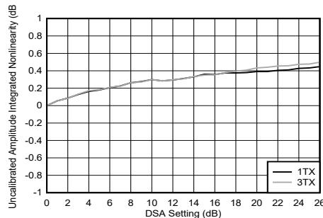
**Figure 4-240. TX DSA Uncalibrated Amplitude Integrated Nonlinearity**
