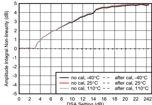
Figure 4-451. RX Amplitude Integrated Non-linearity at 9.6 GHz
