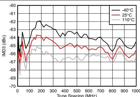
Figure 4-258. TX IMD3 vs Tone Spacing at 9.61 GHz
