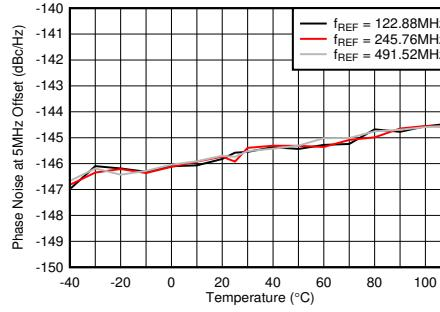
PLL enabled, f<sub>VCO</sub> = 9830.4 MHz, measured at TX output
