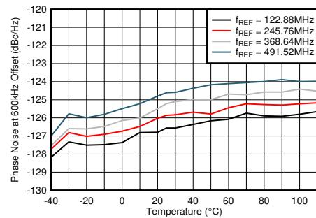
PLL enabled,  $f_{VCO} = 11796.48$  MHz, measured at TX output
