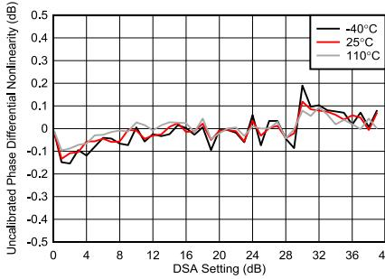
Figure 4-197. TX DSA Uncalibrated Phase Differential Nonlinearity at 8.11 GHz
