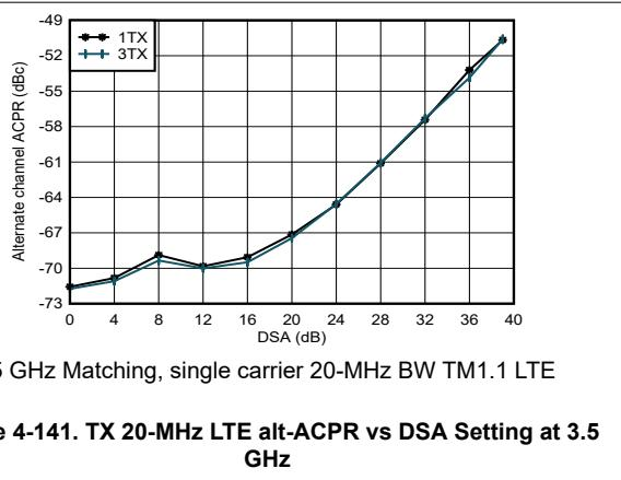
Figure 4-141. TX 20-MHz LTE alt-ACPR vs DSA Setting at 3.5 GHz
