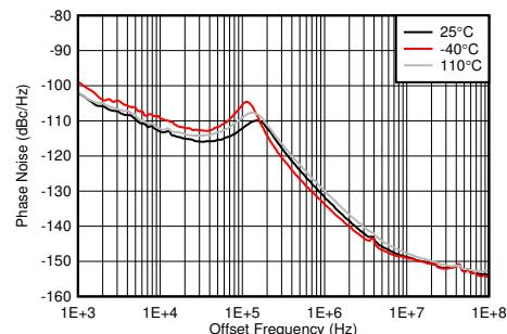
PLL enabled,  $f_{VCO} = 7864.32$  MHz,  $f_{REF} = 491.52$  MSPS, measured at TX output
