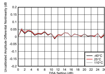
Figure 4-238. TX DSA Uncalibrated Amplitude Differential Nonlinearity
