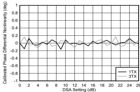
**Figure 4-245. TX DSA Calibrated Phase Differential Nonlinearity**
