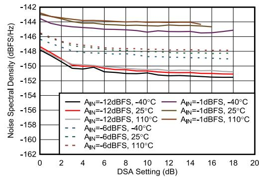
Figure 4-433. RX NSD vs DSA Setting at 8.11GHz
