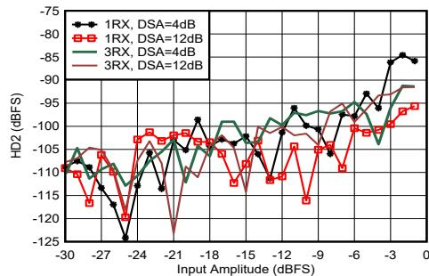
With 1.8 GHz matching,  $f_{\text{in}} = 1900 \text{ MHz}$ , measured after HD2 trim, DDC bypass mode (TI only mode for characterization)
