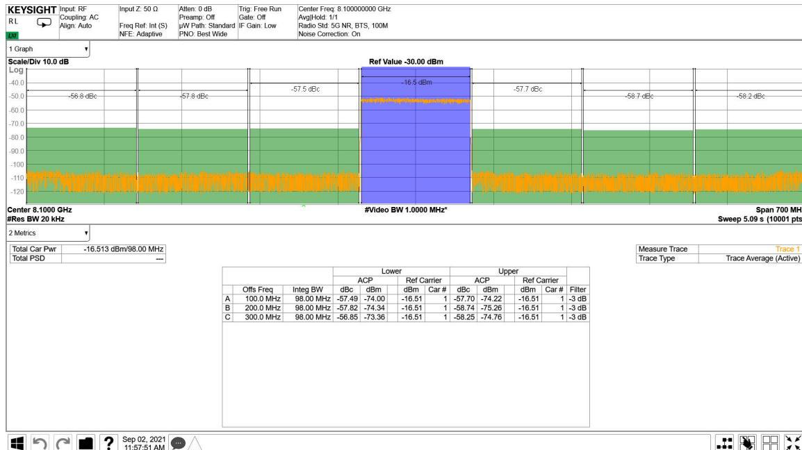
Figure 4-229. TX 100 MHz NR Output Spectrum at 8.11 GHz
