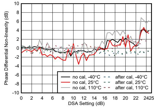
Figure 4-453. RX Phase Integrated Non-linearity at 9.6 GHz
