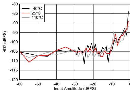
Figure 4-435. RX HD2 vs Digital Amplitude at 8.11GHz
