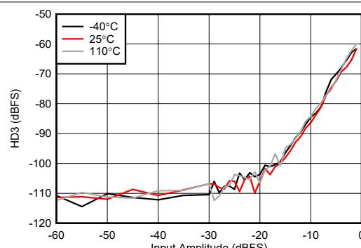
Figure 4-463. RX HD3 vs Digital Level at 9.6 GHz
