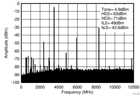
Matching at 3.5 GHz,  $f_{\text{DAC}} = 11.79648$  GSPS, interleave mode.
