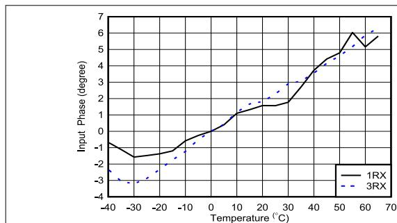
With 0.8 GHz matching, normalized to phase at  $25^\circ\text{C}$
