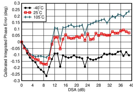
$f_{\text{DAC}} = 8847.36$  MSPS, straight mode, matching at 2.6 GHz, channel with the median variation over DSA setting at 25°C
