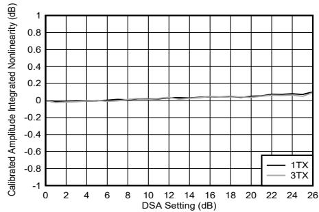
**Figure 4-241. TX DSA Calibrated Amplitude Integrated Nonlinearity**
