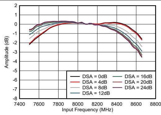
Figure 4-423. RX Amplitude vs Frequency and DSA Setting
