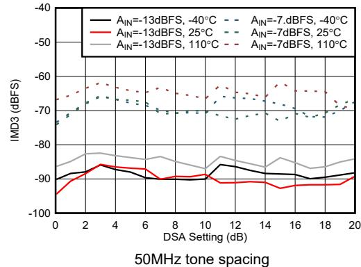
Figure 4-455. RX IMD3 vs DSA Setting at 9.6 GHz
