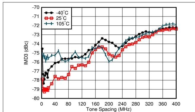
$f_{\text{DAC}} = 5898.24$  MSPS, straight mode,  $f_{\text{CENTER}} = 0.85$  GHz, matching at 0.8 GHz, -13 dBFS each tone, worst channel
