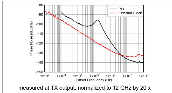
measured at TX output, normalized to 12 GHz by  $20 \times \log_{10}(12\text{GHz}/F_{\text{OUT}})$
