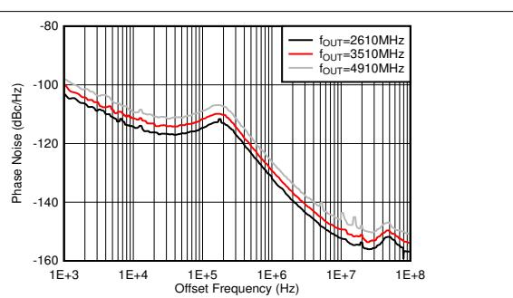
PLL enabled,  $f_{\text{VCO}} = 11796.48 \text{ MHz}$ ,  $f_{\text{REF}} = 491.52 \text{ MSPS}$ , measured at TX output
