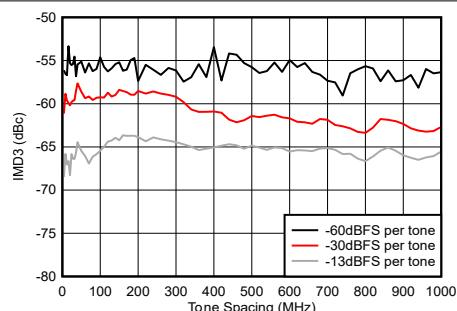
Figure 4-257. TX IMD3 vs Tone Spacing at 9.61 GHz
