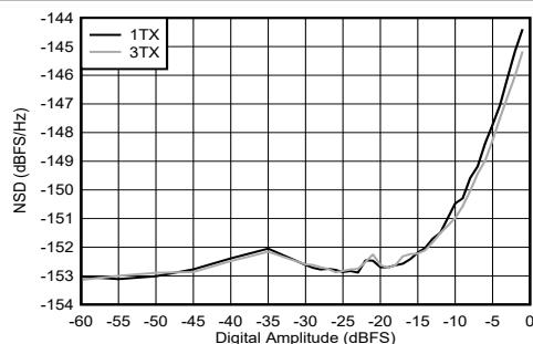
Figure 4-259. TX NSD vs Digital Amplitude at 9.61 GHz
