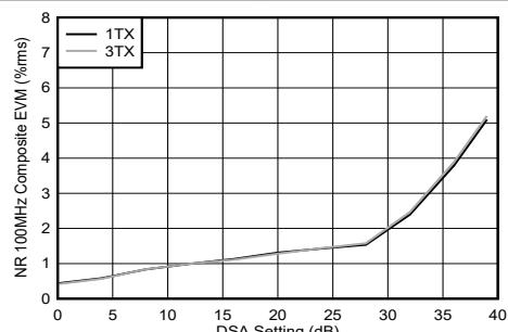
Figure 4-228. TX NR100 MHz EVM vs DSA Setting 8.11 GHz
