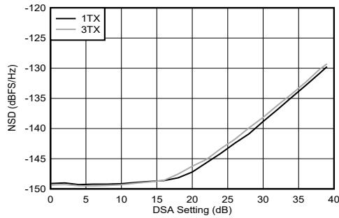
Figure 4-262. TX NSD vs DSA Setting at 9.61 GHz
