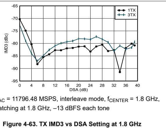
Figure 4-63. TX IMD3 vs DSA Setting at 1.8 GHz
