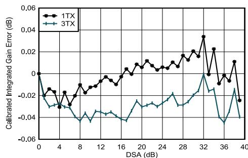
$f_{\text{DAC}} = 5898.24$  MSPS, interleave mode, matching at 1.8 GHz
