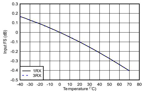
With 1.8 GHz matching, normalized to fullscale at  $25^\circ\text{C}$  for each channel
