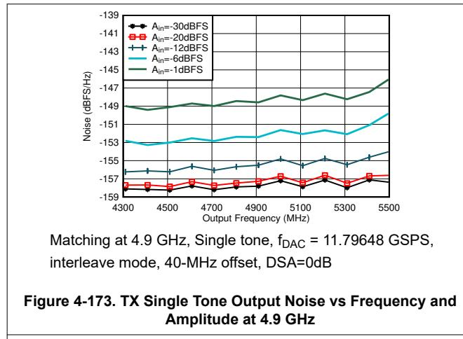
Figure 4-173. TX Single Tone Output Noise vs Frequency and Amplitude at 4.9 GHz
