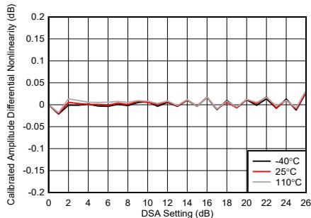
**Figure 4-239. TX DSA Calibrated Amplitude Differential Nonlinearity**
