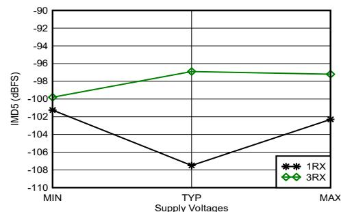
With 3.6 GHz matching, -7 dBFS each tone, 20-MHz tone spacing, all supplies at MIN, TYP, or MAX recommended operating voltages
