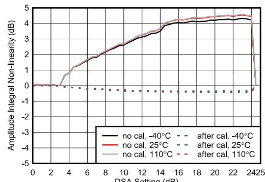
Figure 4-425. RX Amplitude Integrated Nonlinearity at 8.1GHz
