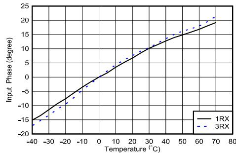
With 2.6 GHz matching, normalized to phase at  $25^\circ\text{C}$
