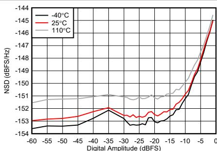
Figure 4-260. TX NSD vs Digital Amplitude at 9.61 GHz
