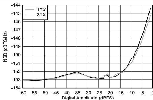
Figure 4-253. TX NSD vs Digital Amplitude at 9.61 GHz
