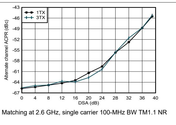
Figure 4-109. TX 100-MHz NR alt-ACPR vs DSA at 2.6 GHz
