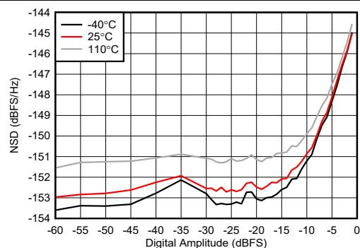
Figure 4-254. TX NSD vs Digital Amplitude at 9.61 GHz
