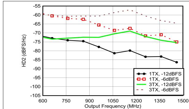
Matching at 0.8 GHz,  $f_{\text{DAC}} = 5898.24$  G SPS, straight mode
