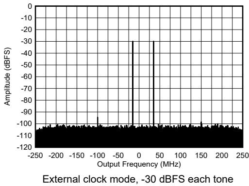
Figure 4-438. RX Dual Tone Output FFT at 8.11 GHz
