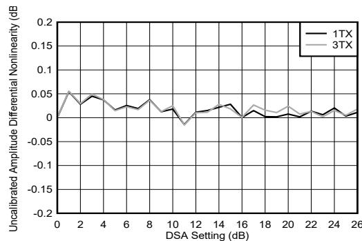
Figure 4-230. TX DSA Uncalibrated Amplitude Differential Nonlinearity
