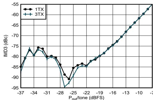
$f_{\text{DAC}} = 11796.48$  MSPS, interleaved mode, matching at 4.9 GHz,  $f_{\text{CENTER}} = 4.9\text{GHz}$ , fSPACING = 20 MHz
