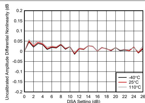
Figure 4-232. TX DSA Uncalibrated Amplitude Differential Nonlinearity
