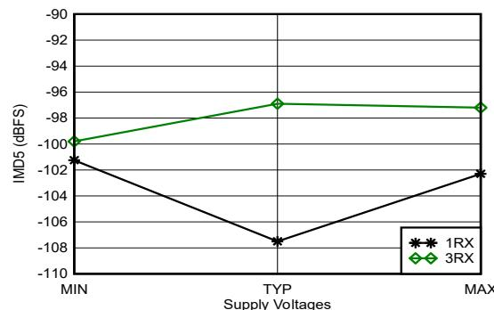
With 3.6 GHz matching,  $-7 \text{ dBFS}$  each tone, 20-MHz tone spacing, all supplies at MIN, TYP, or MAX recommended operating voltages
