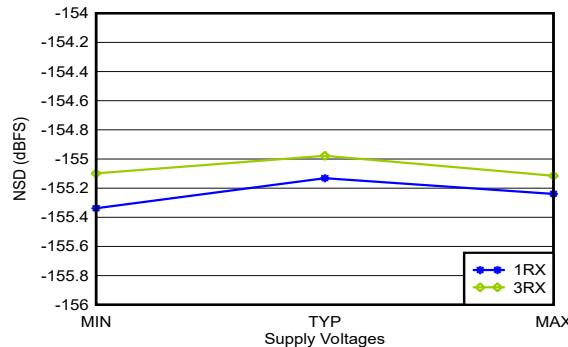
With 0.8 GHz matching, 12.5-MHz offset, all supplies at MIN, TYP, or MAX recommended operating voltages
