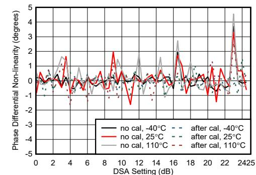
Figure 4-444. RX Phase Differential Non-linearity at 9.6 GHz
