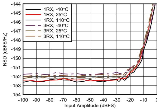
Figure 4-450. RX NSD vs Digital Amplitude at 9.6 GHz
