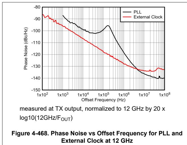
**Figure 4-468. Phase Noise vs Offset Frequency for PLL and External Clock at 12 GHz**
