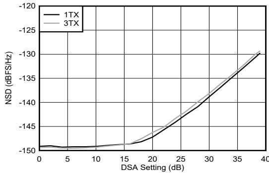
Figure 4-256. TX NSD vs DSA Setting at 9.61 GHz
