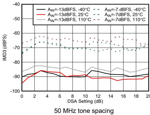
Figure 4-448. RX IMD3 vs DSA Setting at 9.6 GHz
