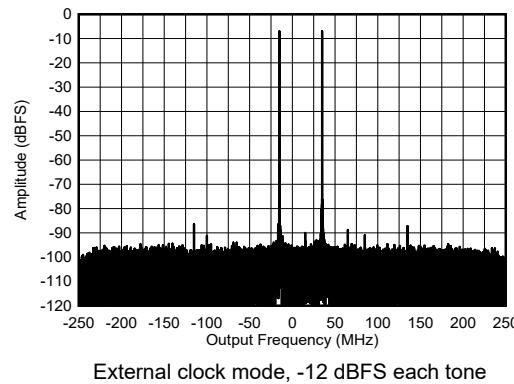
Figure 4-437. RX Dual Tone Output FFT at 8.11 GHz
