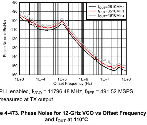
**Figure 4-473. Phase Noise for 12-GHz VCO vs Offset Frequency and f<sub>OUT</sub> at 110°C**
