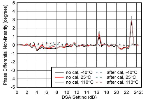
Figure 4-416. RX Phase Differential Nonlinearity at 8.11 GHz
