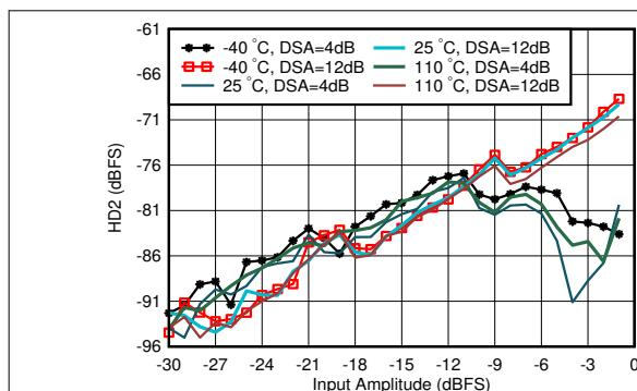
With 0.8 GHz matching, measured after HD2 trim, DDC bypass mode (TI only mode for characterization)
