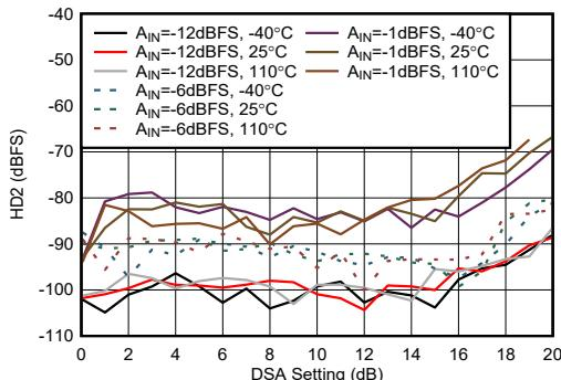
Figure 4-454. RX HD2 vs DSA Setting at 9.6 GHz
