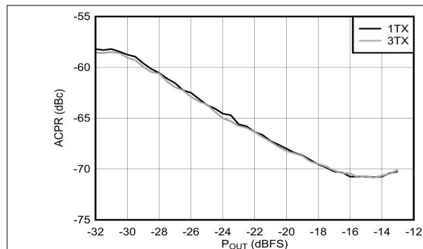
3.5 GHz Matching, single carrier 20-MHz BW TM1.1 LTE
