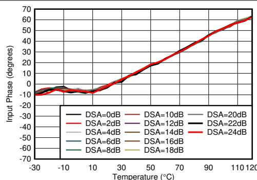
**Figure 4-337. RX Input Phase vs Temperature at 3.6 GHz**
