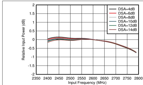
With matching, normalized to power at 2.6 GHz for each DSA setting
