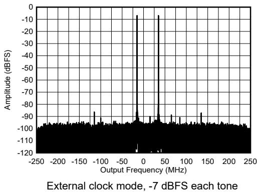
Figure 4-436. RX Dual Tone Output FFT at 8.11 GHz
