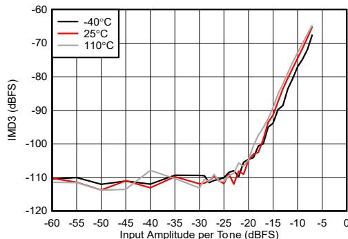
Figure 4-446. RX IMD3 vs Digital Amplitude at 9.6 GHz
