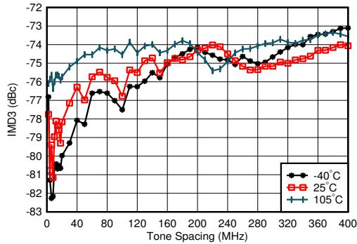
$f_{\text{DAC}} = 11796.48$  MSPS, straight mode,  $f_{\text{CENTER}} = 0.85$  GHz,
