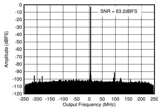
Figure 4-286. RX Output FFT at 0.8 GHz
