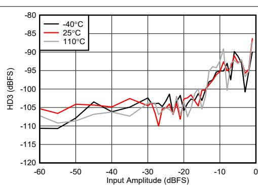
Figure 4-427. RX HD3 vs Digital Amplitude at 8.11 GHz
