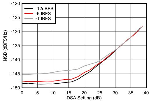
Figure 4-255. TX NSD vs DSA Setting at 9.61 GHz
