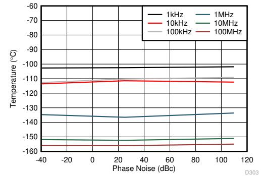
PLL enabled,  $f_{VCO} = 8847.36$  MHz,  $f_{REF} = 491.52$  MSPS, minimum LPF BW, measured at TX output
