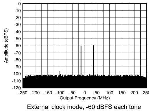
Figure 4-439. RX Dual Tone Output FFT at 8.11 GHz
