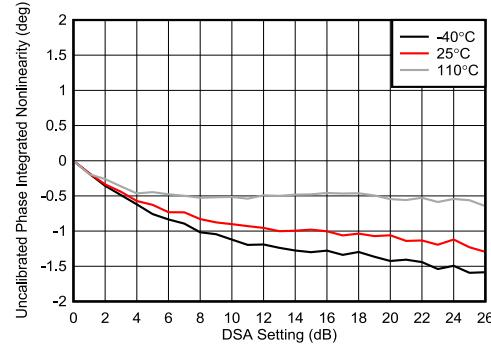
Figure 4-244. TX DSA Uncalibrated Phase Integrated Nonlinearity
