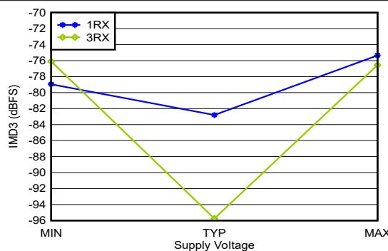
With 4.9 GHz matching, -7 dBFS each tone, 20-MHz tone spacing, all supplies at MIN, TYP, or MAX recommended operating voltages
