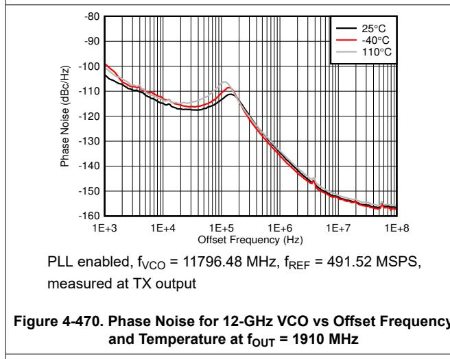
**Figure 4-470. Phase Noise for 12-GHz VCO vs Offset Frequency and Temperature at f<sub>OUT</sub> = 1910 MHz**
