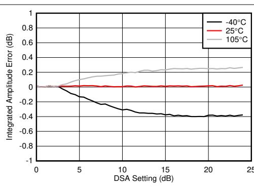
**Figure 4-341. RX Calibrated Integrated Amplitude Error vs DSA Setting at 3.6 GHz**
