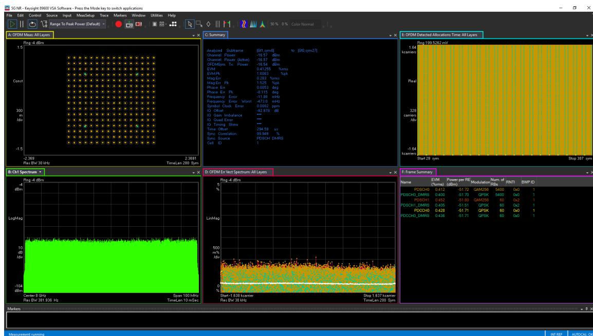
Figure 4-224. TX 100 MHz NR EVM at 8.11 GHz
