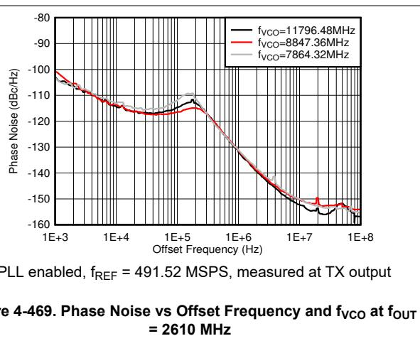
**Figure 4-469. Phase Noise vs Offset Frequency and f<sub>VCO</sub> at f<sub>OUT</sub> = 2610 MHz**
