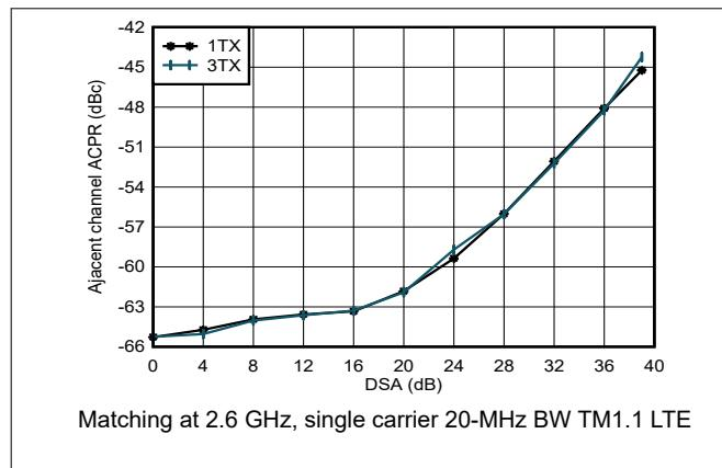
Figure 4-106. TX 20-MHz LTE ACPR vs DSA at 2.6 GHz
