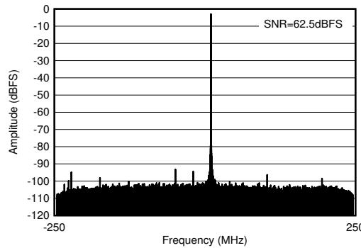
With 2.6 GHz matching,  $f_{\text{IN}} = 2610 \text{ MHz}$ ,  $A_{\text{IN}} = -3 \text{ dBFS}$
