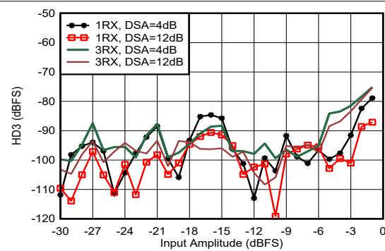
With 1.8 GHz matching,  $f_{\text{in}} = 1900$  MHz, DDC bypass mode (TI only mode for characterization)
