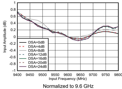
Figure 4-441. RX Input Amplitude vs Frequency at 9.6 GHz
