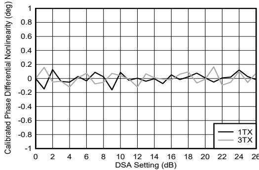
Figure 4-239. TX DSA Calibrated Phase Differential Nonlinearity
