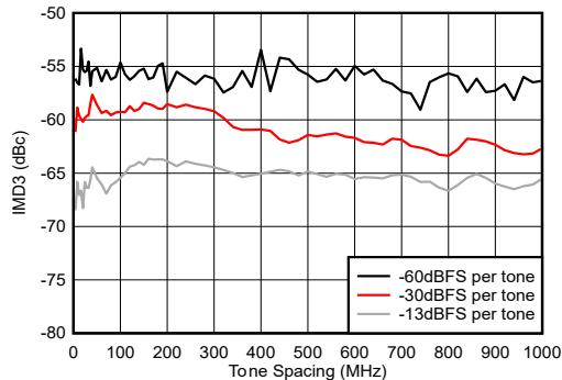
Figure 4-251. TX IMD3 vs Tone Spacing at 9.61 GHz
