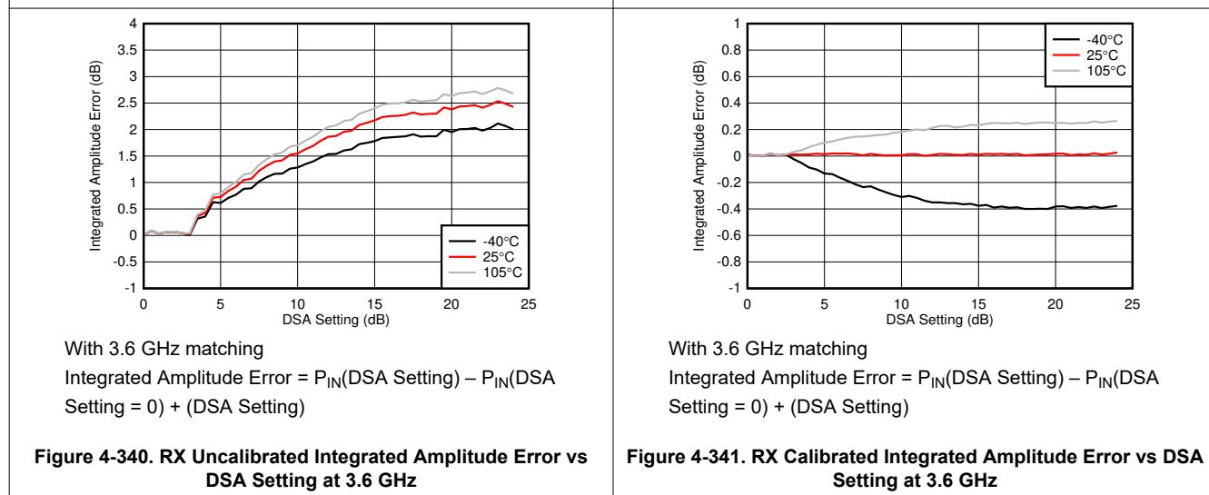
**Figure 4-340. RX Uncalibrated Integrated Amplitude Error vs DSA Setting at 3.6 GHz**
