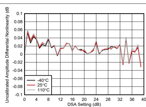
Figure 4-187. TX DSA Uncalibrated Amplitude Differential Nonlinearity at 8.11 GHz
