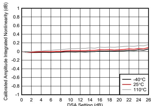
Figure 4-237. TX DSA Calibrated Amplitude Integrated Nonlinearity
