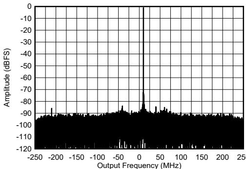
Figure 4-457. RX Single Tone Output FFT at 9.61 GHz
