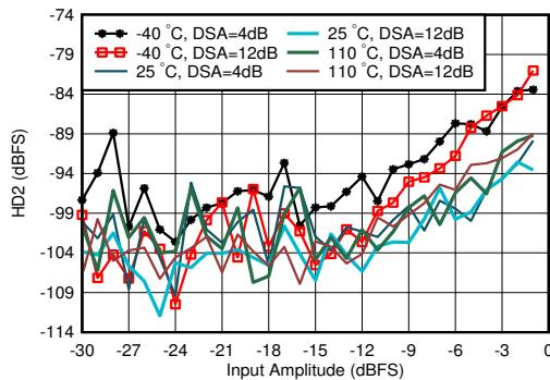
With 1.8 GHz matching,  $f_{\text{in}} = 1900$  MHz, measured after HD2 trim, DDC bypass mode (TI only mode for characterization)
