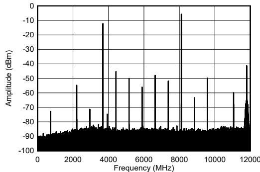
Figure 4-201. TX Single Tone Output Spectrum at 8.11 GHz
