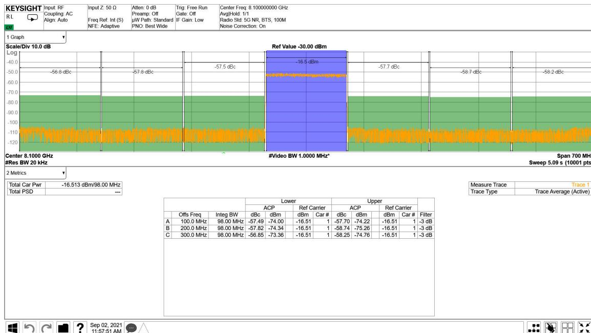
Figure 4-223. TX 100 MHz NR Output Spectrum at 8.11 GHz
