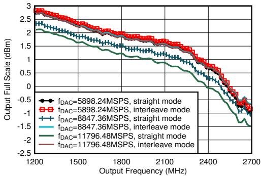
including PCB and cable losses,  $A_{\text{out}} = -0.5$  dBFS, DSA = 0, 1.8 GHz matching
