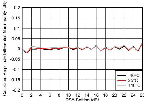
Figure 4-233. TX DSA Calibrated Amplitude Differential Nonlinearity
