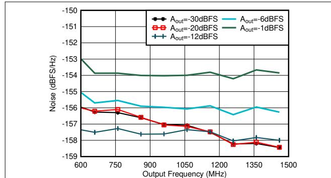
Matching at 2.6 GHz, Single tone,  $f_{\text{DAC}} = 11.79648$  GSPS, interleave mode, 40-MHz offset, DSA = 0dB
