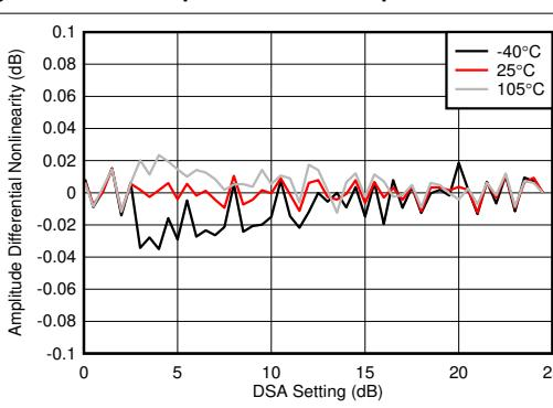
**Figure 4-339. RX Calibrated Differential Amplitude Error vs DSA Setting at 3.6 GHz**
