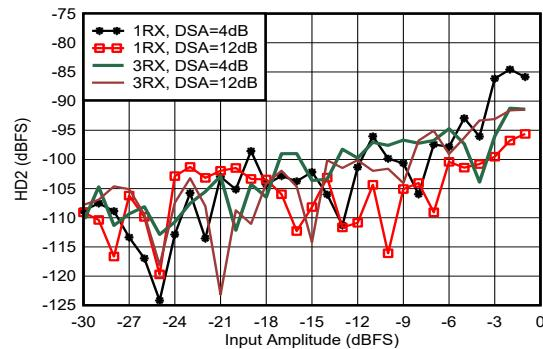
With 1.8 GHz matching,  $f_{\text{in}} = 1900$  MHz, measured after HD2 trim, DDC bypass mode (TI only mode for characterization)
