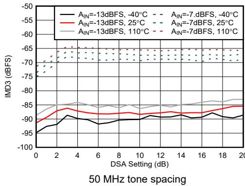
Figure 4-419. RX IMD3 vs DSA Setting at 8.11 GHz
