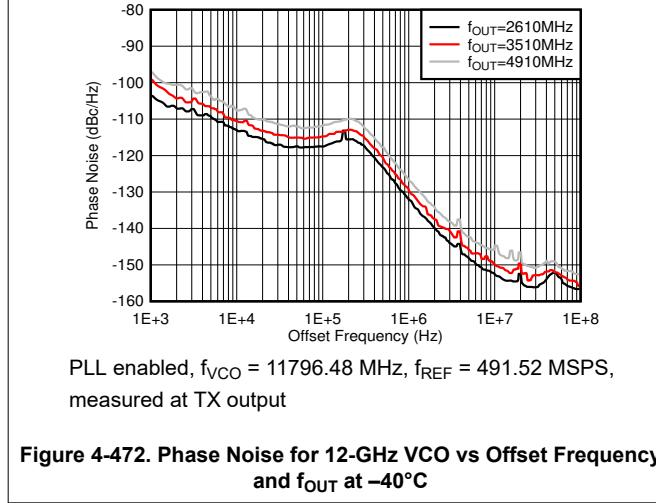
**Figure 4-472. Phase Noise for 12-GHz VCO vs Offset Frequency and f<sub>OUT</sub> at -40°C**
