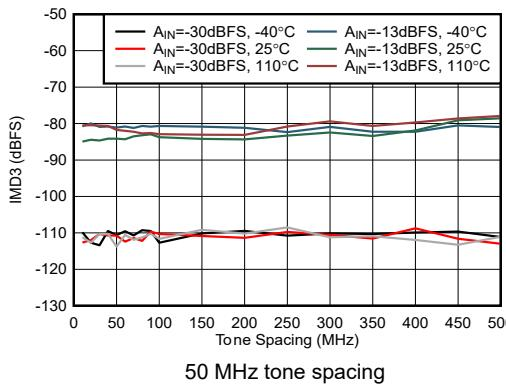
Figure 4-449. RX IMD3 vs Tone Spacing at 9.6 GHz
