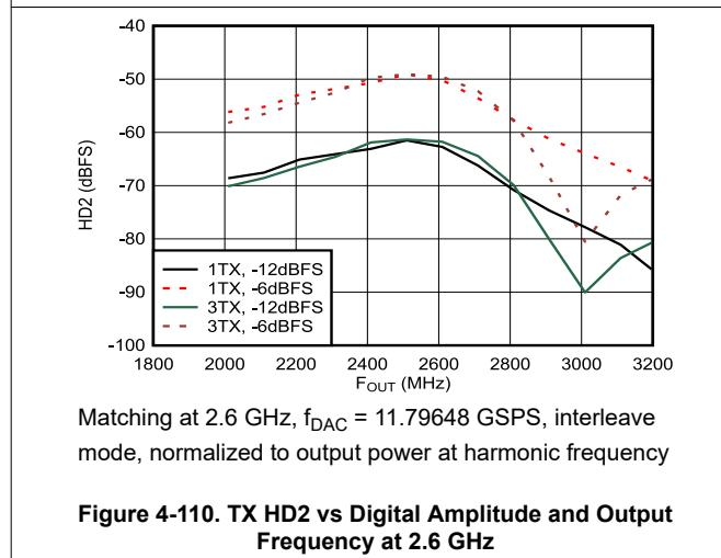
Figure 4-110. TX HD2 vs Digital Amplitude and Output Frequency at 2.6 GHz
