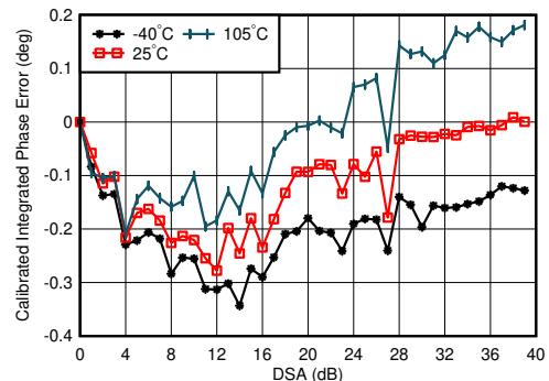
$f_{\text{DAC}} = 11796.48$  MSPS, interleaved mode, matching at 4.9 GHz, channel with the median variation over DSA setting at 25°C
