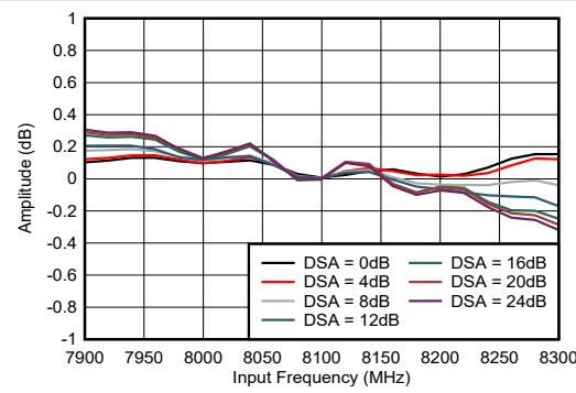
Figure 4-413. RX Amplitude vs Frequency and DSA Setting
