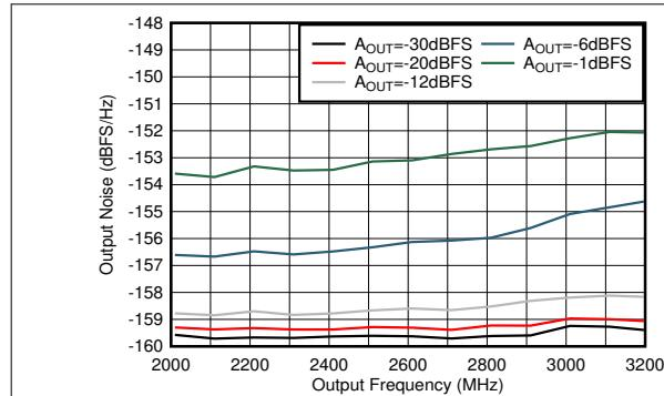
Matching at 2.6 GHz, Single tone,  $f_{\text{DAC}} = 11.79648$  GSPS, interleave mode, 40-MHz offset
