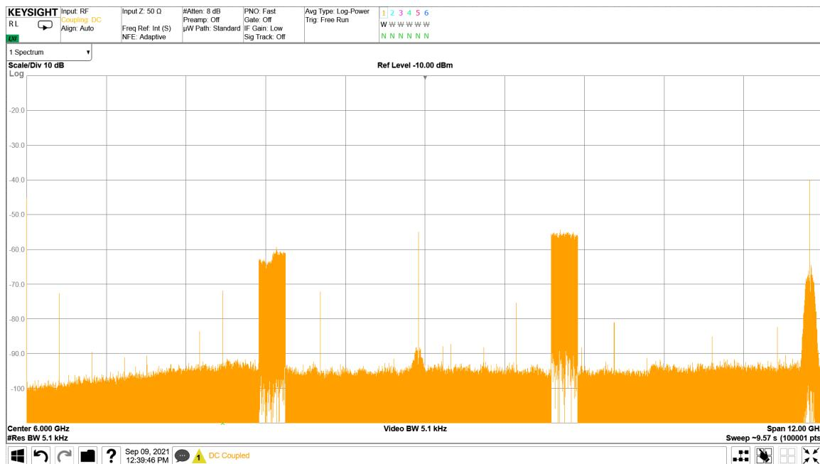
Figure 4-226. TX 4x100 MHz NR Output Spectrum 8.11 GHz
