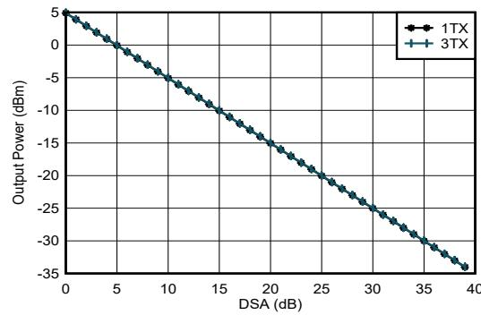
$f_{\text{DAC}} = 11796.48$  MSPS, interleave mode,  $A_{\text{out}} = -0.5$  dBFS, matching 0.8 GHz
