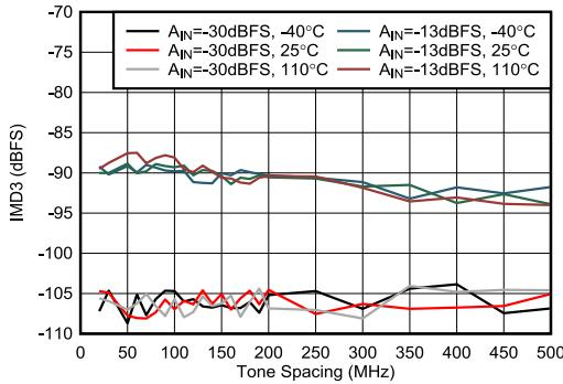
Figure 4-420. RX IMD3 vs Tone Spacing at 8.11 GHz
