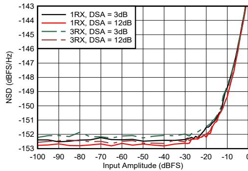
Figure 4-451. RX NSD vs Digital Amplitude at 9.6 GHz
