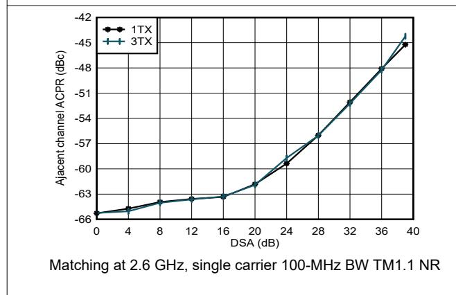
Figure 4-108. TX 100-MHz NR ACPR vs DSA at 2.6 GHz
