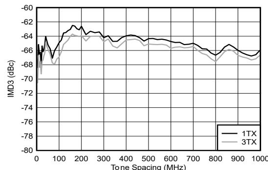
Figure 4-250. TX IMD3 vs Tone Spacing at 9.61 GHz
