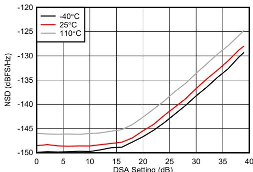
Figure 4-257. TX NSD vs DSA Setting at 9.61 GHz
