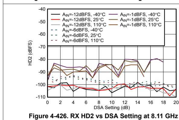
Figure 4-426. RX HD2 vs DSA Setting at 8.11 GHz
