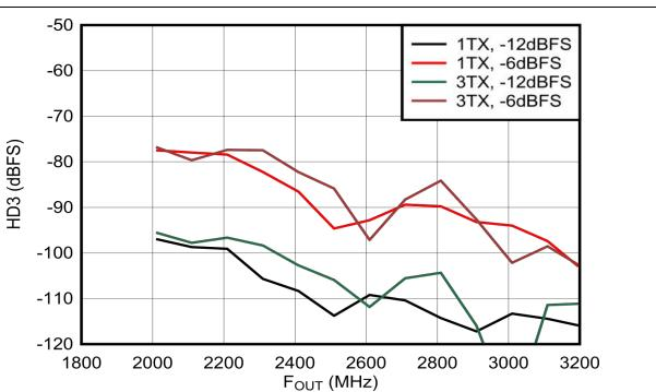
Figure 4-111. TX HD3 vs Digital Amplitude and Output Frequency at 2.6 GHz
