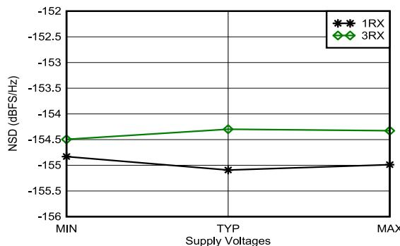
With 3.6 GHz matching, tone at  $-20 \text{ dBFS}$ , 12.5-MHz offset frequency, all supplies at MIN, TYP, or MAX recommended operating voltages
