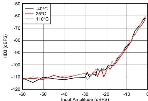
Figure 4-455. RX HD3 vs Digital Level at 9.6 GHz
