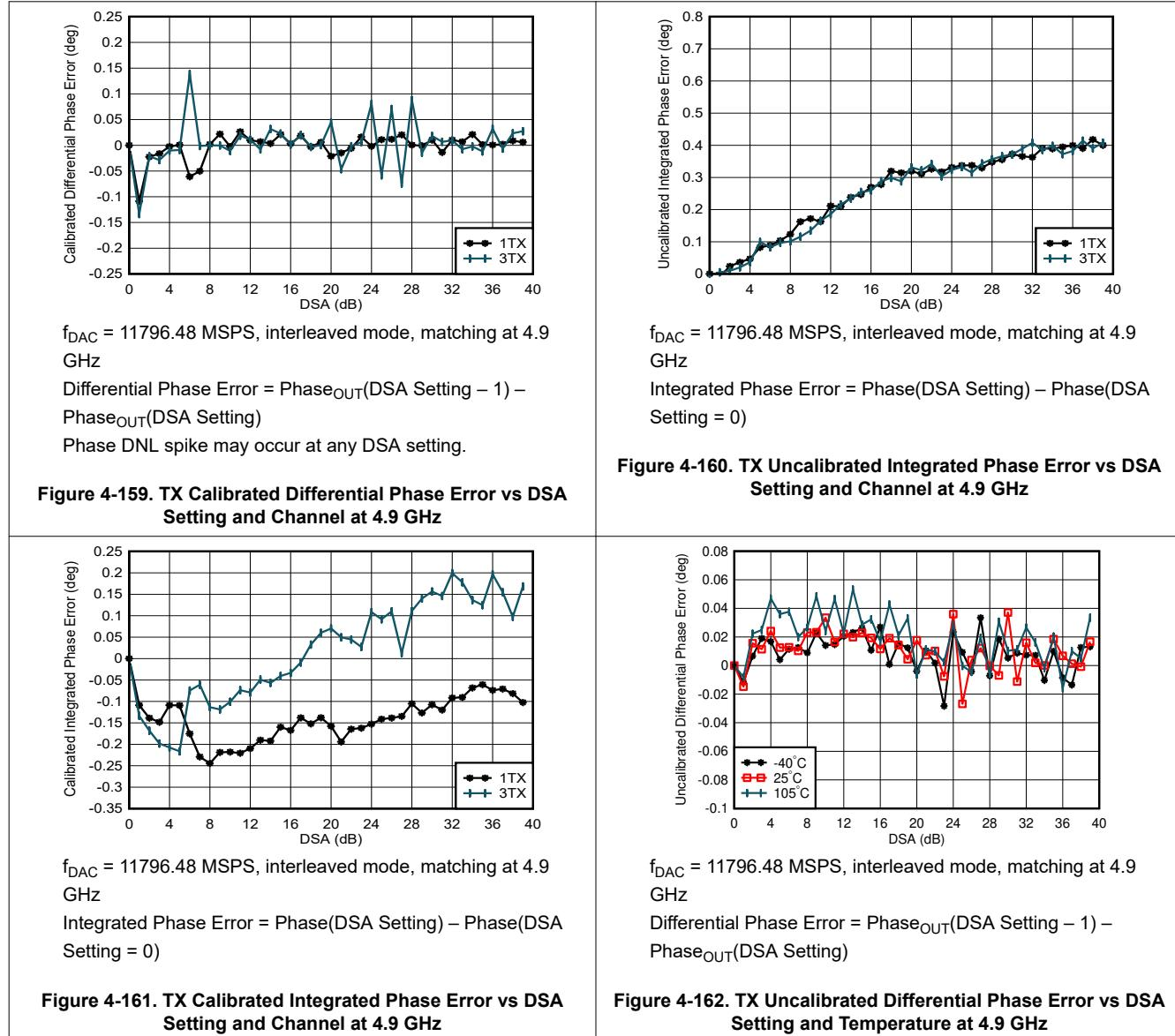
Figure 4-159. TX Calibrated Differential Phase Error vs DSA Setting and Channel at 4.9 GHz
