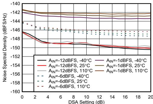
Figure 4-452. RX NSD vs DSA Setting at 9.6 GHz
