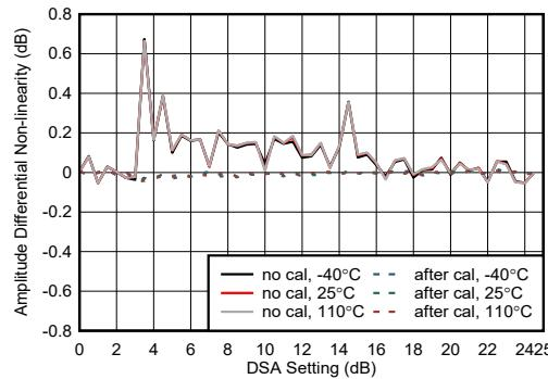
Figure 4-414. RX Amplitude Differential Nonlinearity at 8.11 GHz
