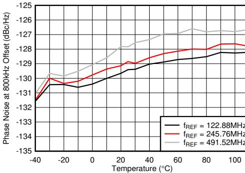
PLL enabled,  $f_{VCO} = 9830.4$  MHz, measured at TX output
