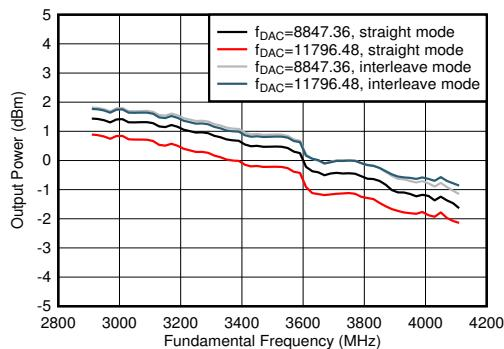
$A_{\text{out}} = -0.5$  dFBS, 3.5 GHz Matching, included PCB and cable losses
