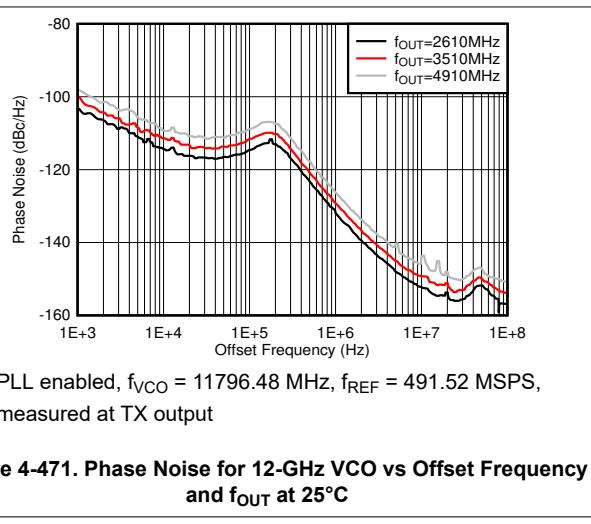
**Figure 4-471. Phase Noise for 12-GHz VCO vs Offset Frequency and f<sub>OUT</sub> at 25°C**
