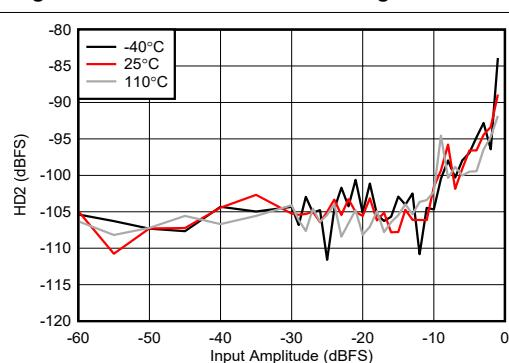
Figure 4-425. RX HD2 vs Digital Amplitude at 8.11 GHz
