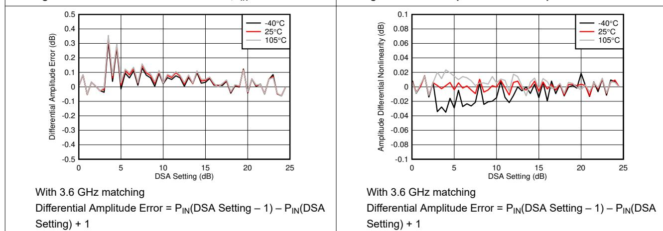
**Figure 4-338. RX Uncalibrated Differential Amplitude Error vs DSA Setting at 3.6 GHz**
