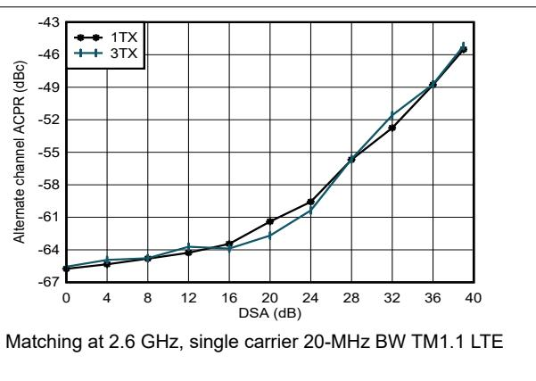
Figure 4-107. TX 20-MHz LTE alt-ACPR vs DSA at 2.6 GHz
