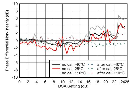
Figure 4-445. RX Phase Integrated Non-linearity at 9.6 GHz
