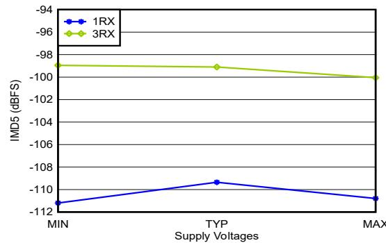
With 0.8 GHz matching,  $-7 \text{ dBFS}$  each tone, 20-MHz tone spacing, all supplies at MIN, TYP, or MAX recommended operating voltages
