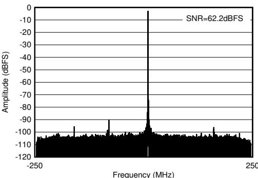
With 3.6 GHz matching,  $f_{\text{IN}} = 3610 \text{ MHz}$ ,  $A_{\text{IN}} = -3 \text{ dBFS}$
