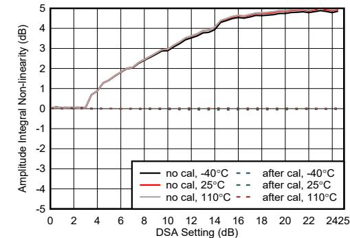
Figure 4-443. RX Amplitude Integrated Non-linearity at 9.6 GHz
