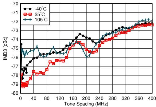
$f_{\text{DAC}} = 5898.24$  MSPS, straight mode,  $f_{\text{CENTER}} = 0.85$  GHz,
