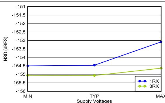
With 4.9 GHz matching, 12.5-MHz offset, all supplies at MIN, TYP, or MAX recommended operating voltages
