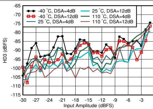
With 1.8 GHz matching,  $f_{\text{in}} = 1900$  MHz, DDC bypass mode (TI only mode for characterization)
