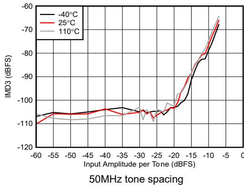
Figure 4-418. RX IMD3 vs Input Amplitude at 8.11 GHz
