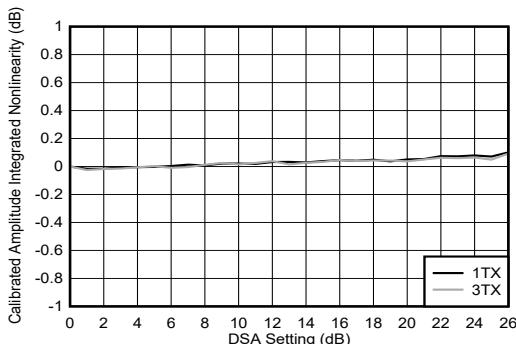
Figure 4-235. TX DSA Calibrated Amplitude Integrated Nonlinearity
