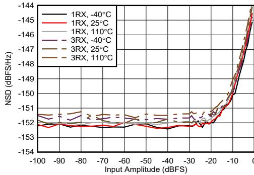
Figure 4-421. RX NSD vs Digital Amplitude at 8.11 GHz
