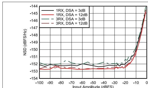
Figure 4-422. RX NSD vs Digital Amplitude at 8.11 GHz
