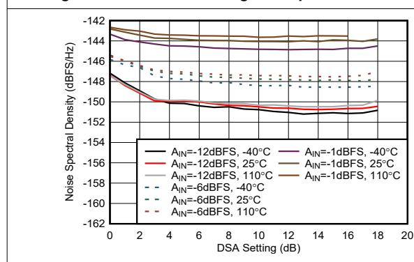
Figure 4-424. RX NSD vs DSA Setting at 8.11 GHz
