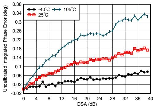
$f_{\text{DAC}} = 5898.24$  MSPS, interleave mode, matching at 1.8 GHz, channel with the median variation over DSA setting at 25°C
