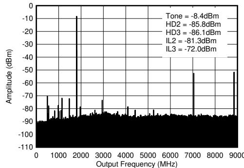
$f_{\text{DAC}} = 8847.36$  MSPS, straight mode, 1.8 GHz matching, includes PCB and cable losses.  $\text{IL}_n = f_s/n \pm f_{\text{OUT}}$  and is due to mixing with digital clocks.
