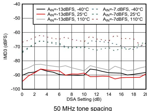
Figure 4-447. RX IMD3 vs DSA Setting at 9.6 GHz
