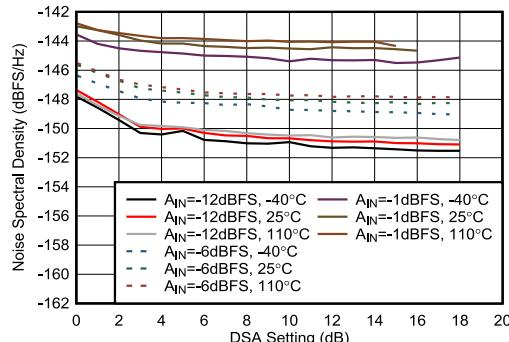
Figure 4-423. RX NSD vs DSA Setting at 8.11 GHz
