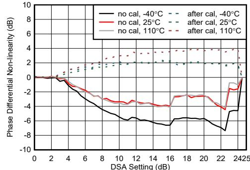
Figure 4-417. RX Phase Differential Nonlinearity at 8.11 GHz
