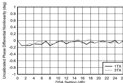
Figure 4-238. TX DSA Uncalibrated Phase Differential Nonlinearity
