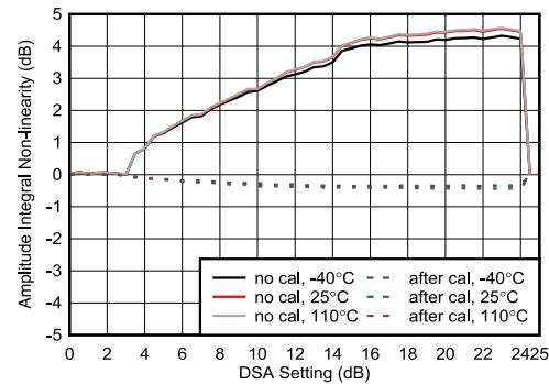
Figure 4-415. RX Amplitude Integrated Nonlinearity at 8.11 GHz
