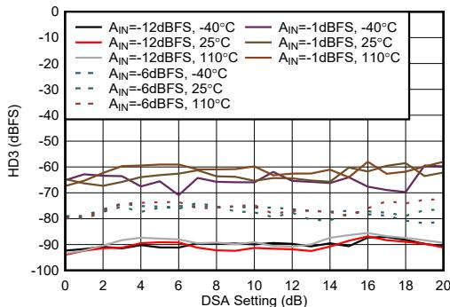
Figure 4-456. RX HD3 vs DSA Setting at 9.6 GHz
