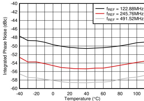
PLL enabled,  $f_{VCO} = 9830.4$  MHz, 1-kHz to 100-MHz, single-sided integration bandwidth, measured at TX output
