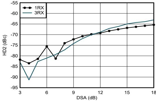
With 0.8 GHz matching, measured after HD2 trim, DDC bypass mode (TI only mode for characterization)
