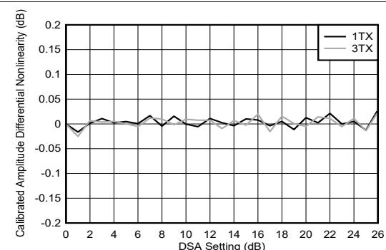
Figure 4-231. TX DSA Calibrated Amplitude Differential Nonlinearity
