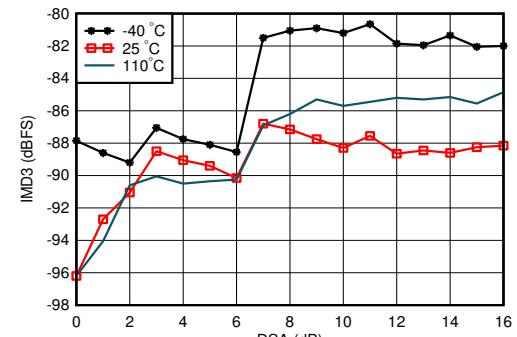
Figure 4-290. RX IMD3 vs DSA Setting and Temperature at 0.8 GHz
