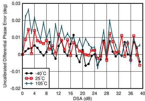
$f_{\text{DAC}} = 5898.24$  MSPS, interleave mode, matching at 1.8 GHz
