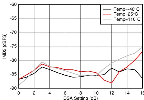
With 3.5 GHz matching, each tone at  $-7 \text{ dBFS}$ , 20-MHz tone spacing
