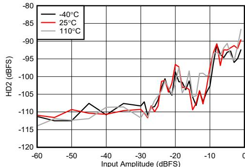
Figure 4-453. RX HD2 vs Digital Level at 9.6 GHz
