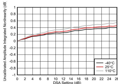
Figure 4-236. TX DSA Uncalibrated Amplitude Integrated Nonlinearity
