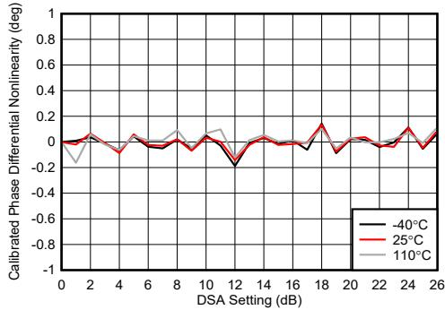
Figure 4-241. TX DSA Calibrated Phase Differential Nonlinearity
