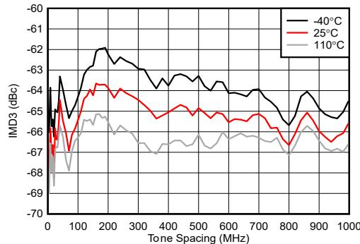
Figure 4-252. TX IMD3 vs Tone Spacing at 9.6 GHz
