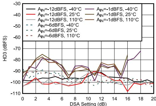
Figure 4-428. RX HD3 vs DSA Setting at 8.11 GHz
