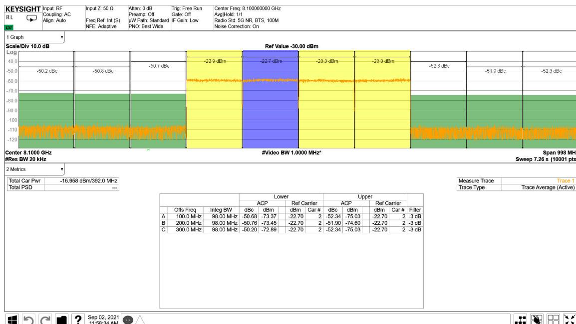
Figure 4-225. TX 4x100 MHz NR Output Spectrum 8.11 GHz
