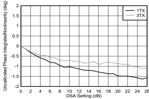
Figure 4-242. TX DSA Uncalibrated Phase Integrated Nonlinearity
