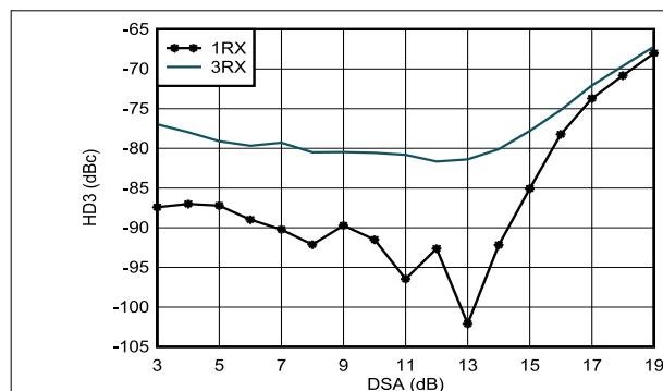
With 1.8 GHz matching,  $f_{\text{in}} = 1900$  MHz, DDC bypass mode (TI only mode for characterization)
