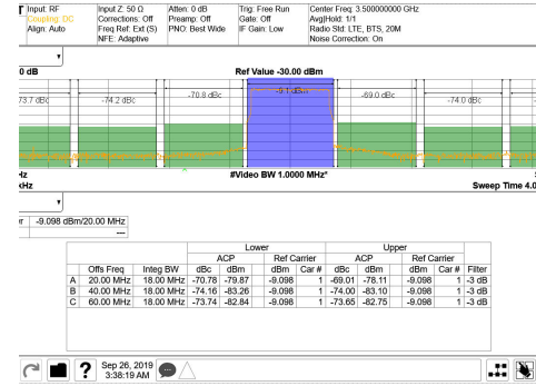
Figure 5-480. TX 20-MHz LTE Output Spectrum at 3.5 GHz (Band 42)
