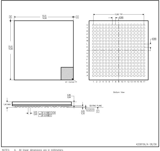
Α. All linear dimensions are in millimeters.
