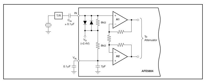
Figure 101. LNA Channel (Simplified Schematic)
