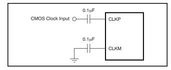
Figure 108. Single-Ended Clock Driving Circuit
