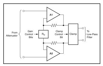
Figure 99. Post-Gain Amplifier (Simplified Schematic)
