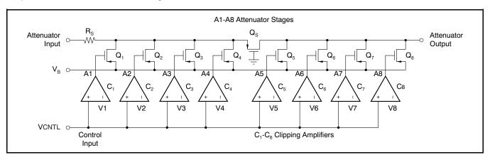
Figure 98. Voltage-Controlled Attenuator Simplified Schematic
