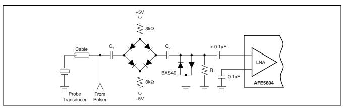
Figure 102. Typical Input Overload Protection Circuit of an Ultrasound System
