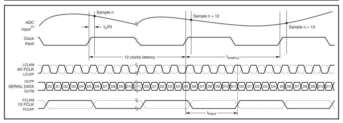
(1) Referenced to ADC Input (internal node) for illustration purposes only.
