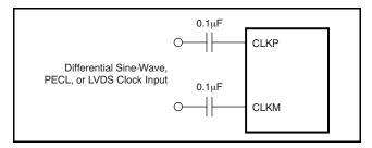
Figure 107. Differential Clock Driving Circuit (DIFF\_CLK = 1)
