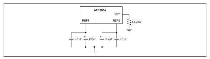
Figure 109. Suggested Decoupling on the Reference Pins
