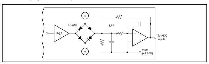
Figure 100. Clamping Stage and Low-Pass Filter (Simplified Schematic)
