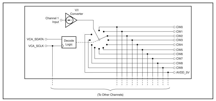
Figure 93. Basic CW Cross-Point Switch Matrix Configuration
