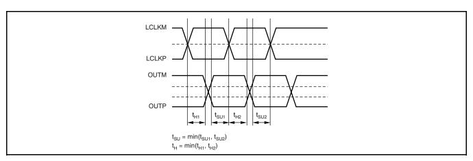
Figure 2. Definition of Setup and Hold Times
