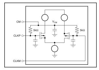
Figure 106. Internal Clock Buffer
