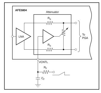
Figure 103. External Filtering of the V<sub>CNTL</sub> Input
