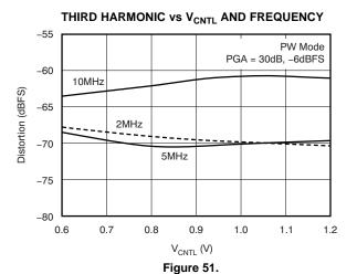
THIRD HARMONIC vs  $V_{CNTL}$  AND FREQUENCY
