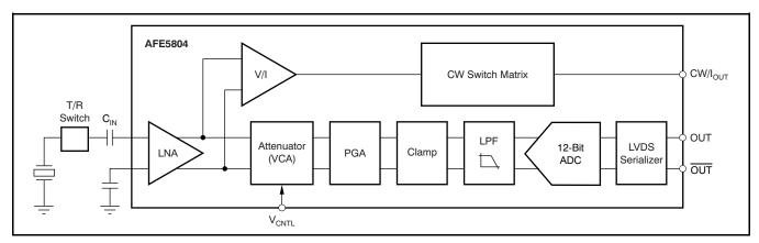
Figure 97. Functional Block Diagram
