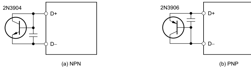
Figure 7-6. Remote Temperature Sensor Using Transistor
