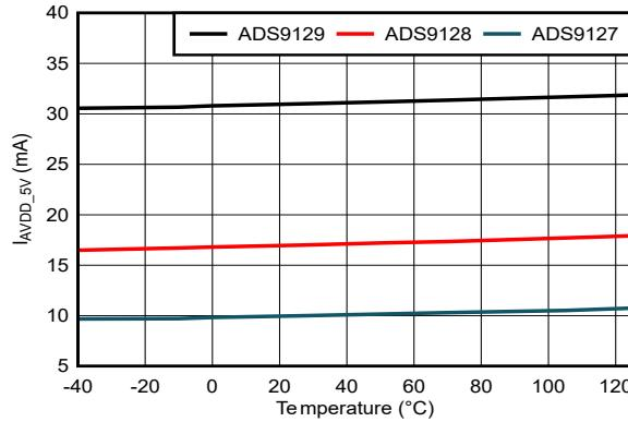
Figure 5-15. AVDD\_5V Current vs Temperature
