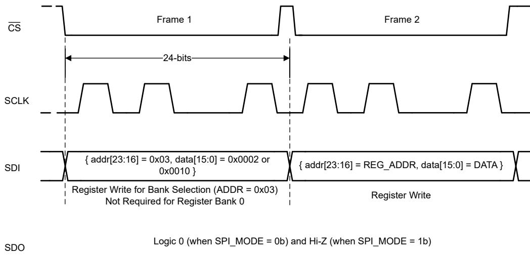
**Figure 6-10. Register Write**
