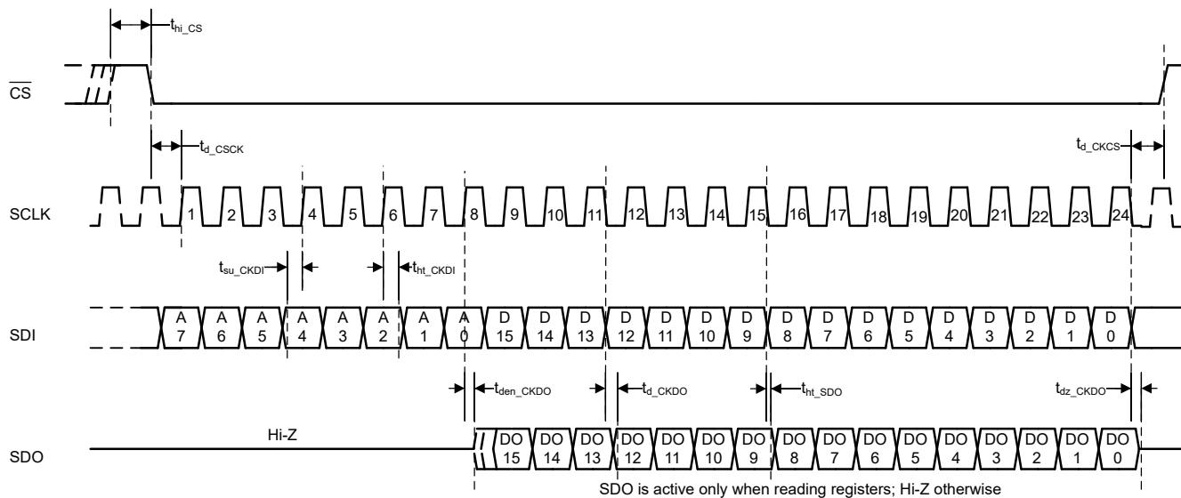
**Figure 5-4. Configuration SPI**
