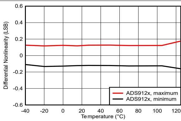
Figure 5-11. DNL vs Temperature
