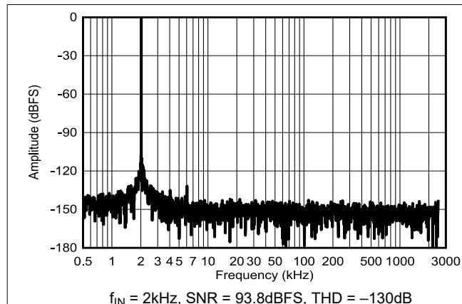
**Figure 8-2. Typical FFT at 5MSPS: ADS9127**
