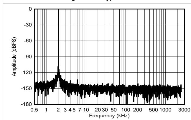
**Figure 5-29. Typical FFT for  $f_{\text{IN}} = 2\text{kHz}$**
