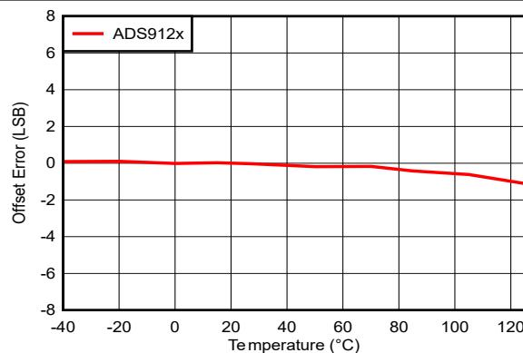
Figure 5-9. Offset Error vs Temperature
