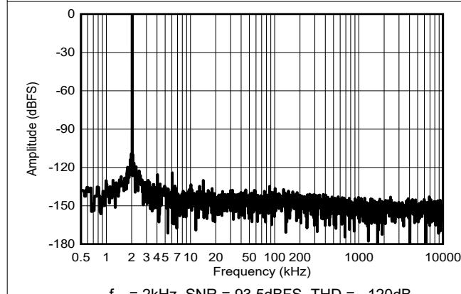
**Figure 5-19. Typical FFT for  $f_{\text{IN}} = 2\text{kHz}$**
