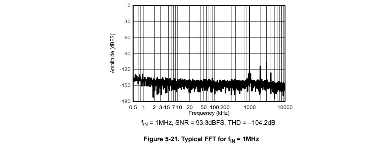
**Figure 5-21. Typical FFT for  $f_{\text{IN}} = 1\text{MHz}$**
