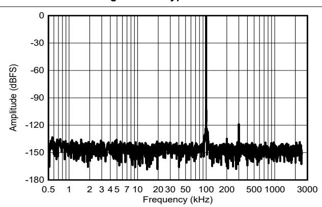
**Figure 5-30. Typical FFT for  $f_{\text{IN}} = 100\text{kHz}$**
