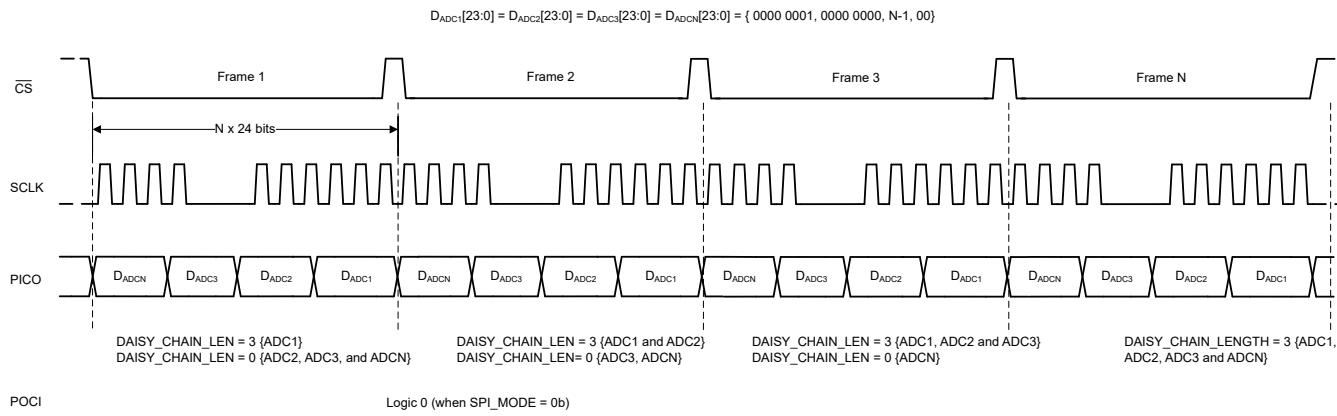
**Figure 6-14. Register Write to Configure Daisy-Chain Length**
