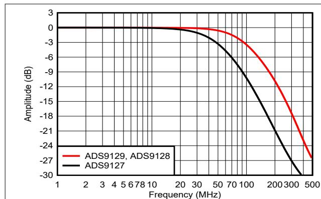
Figure 5-7. Typical Analog Input Bandwidth
