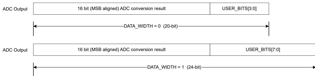
**Figure 6-6. Data Frame Width Composition**
