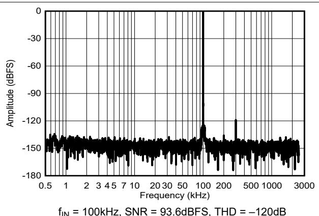
Figure 8-6. Typical FFT at 5MSPS: ADS9127
