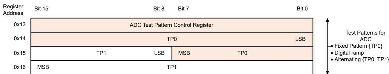
**Figure 6-7. Register Bank for Test Patterns**
