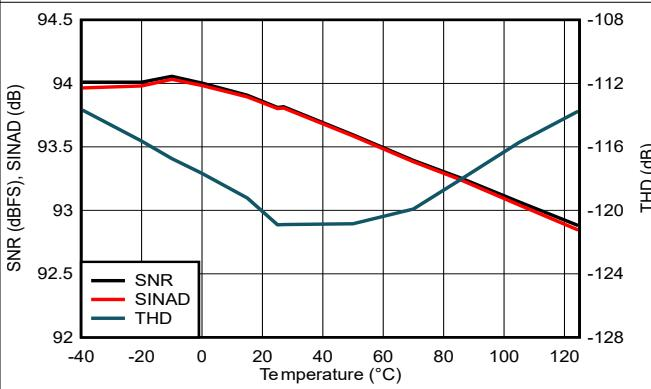
Figure 5-12. SNR, SINAD, and THD vs Temperature
