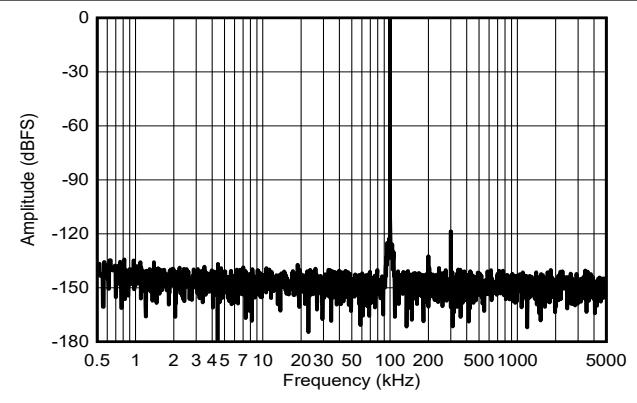
**Figure 5-25. Typical FFT for  $f_{\text{IN}} = 100\text{kHz}$**
