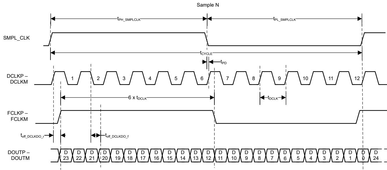
**Figure 5-1. LVDS Data Interface: DDR**
