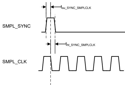
**Figure 5-5. SMPL\_SYNC Timing**
