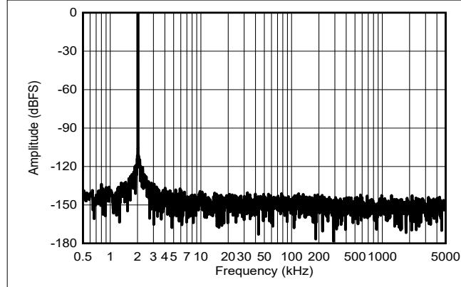
**Figure 5-24. Typical FFT for  $f_{\text{IN}} = 2\text{kHz}$**
