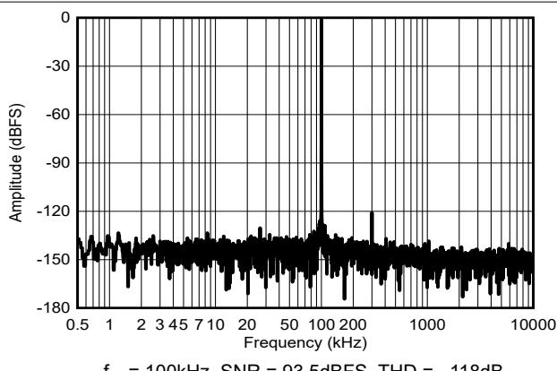
**Figure 5-20. Typical FFT for  $f_{\text{IN}} = 100\text{kHz}$**
