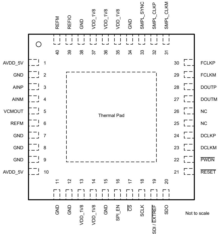
Figure 4-1. RHA Package, 6mm × 6mm, 40-Pin VQFN (Top View)
