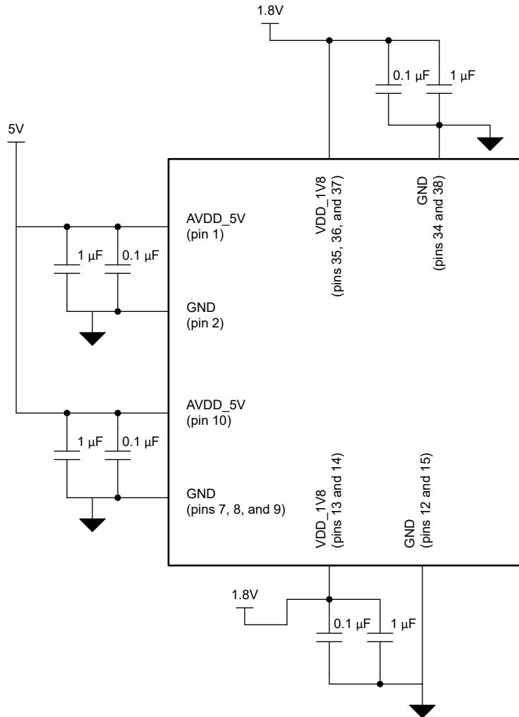
**Figure 8-10. Power-Supply Decoupling**
