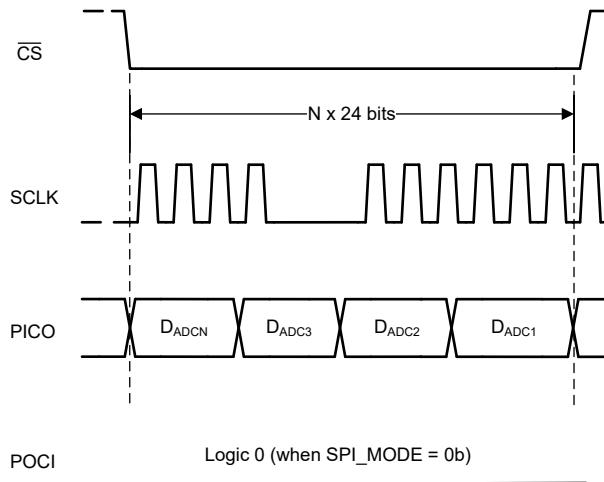
**Figure 6-13. Register Write With Daisy-Chain**
