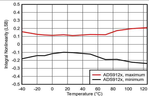
Figure 5-10. INL vs Temperature
