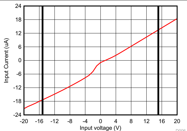
Figure 7-4. I-V Curve for the Input OVP Circuit (AVDD = Floating)
