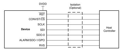
Figure 6-20. All multiSPI Protocols Pin Configuration
