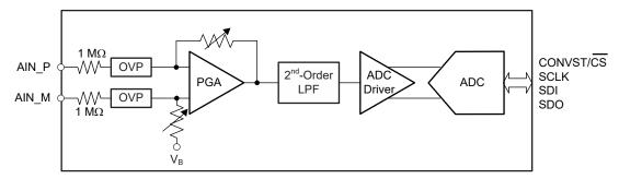
Figure 6-1. Simplified Analog Front-End Circuit Schematic
