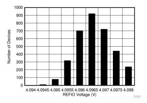
Figure 6-8. Internal Reference Accuracy Histogram at Room Temperature
