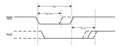
Figure 5-2. Asynchronous Reset Timing Diagram
