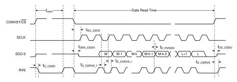
Figure 5-7. multiSPI Source-Synchronous External Clock Serial Interface Timing Diagram
