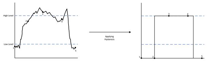
Figure 8-4. Alarm Functionality With Hysteresis
