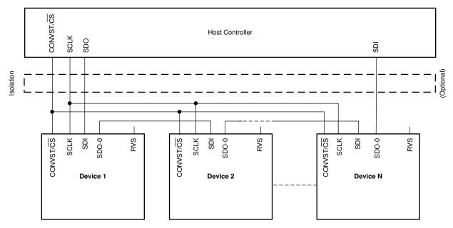
Figure 6-22. Daisy-Chain Connection Schematic
