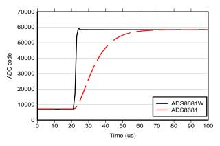
Figure 8-2. Step Settling Response Time
