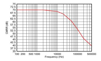
Figure 8-5. Common-Mode Rejection Ratio vs Frequency
