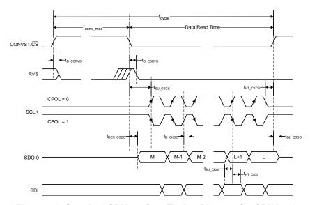
Figure 5-3. Standard SPI Interface Timing Diagram for CPHA = 0
