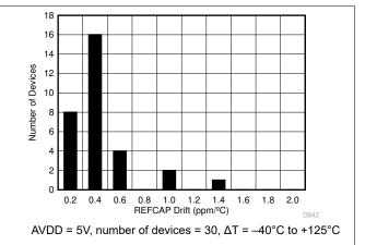
Figure 6-14. Reference Buffer Temperature Drift Histogram
