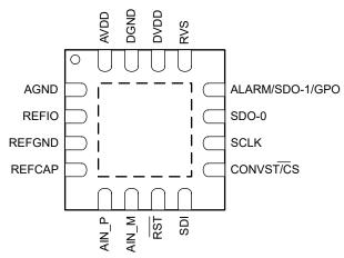
Figure 4-1. RUM Package, 16-Pin WQFN (Top View)
