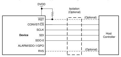
Figure 6-21. Standard SPI Protocol Pin Configuration
