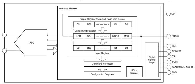
Figure 6-19. Device Interface Module
