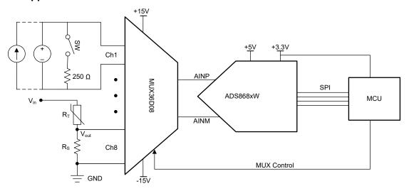
Figure 8-1. 16-Bit, 8-Channel, Analog Input Module for Programmable Logic Controllers (PLCs)
