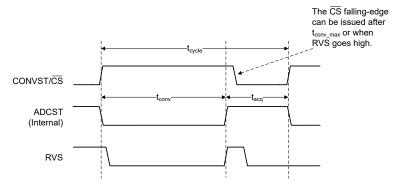
Figure 5-1. Conversion Cycle Timing Diagram
