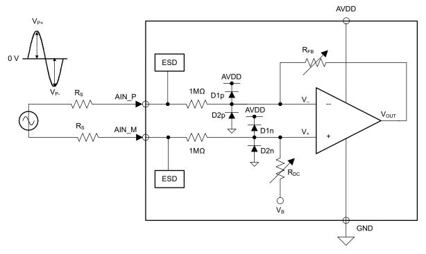
Figure 6-2. Input Overvoltage Protection Circuit Schematic
