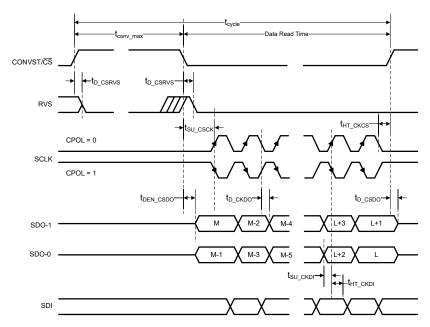
Figure 5-5. multiSPI Interface Timing Diagram for Dual SDO-x and CPHA = 0
