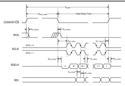
Figure 5-4. Standard SPI Interface Timing Diagram for CPHA = 1
