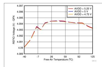
Figure 6-10. REFIO Voltage Variation Across AVDD and Temperature
