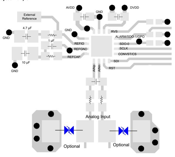
Figure 8-8. Board Layout for the ADS868xW
