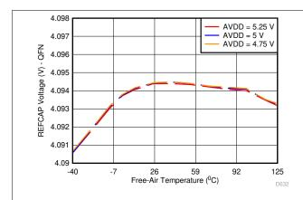
Figure 6-13. Reference Buffer Output (REFCAP)
