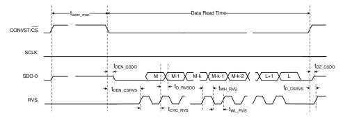
Figure 5-8. multiSPI Source-Synchronous Internal Clock Serial Interface Timing Diagram
