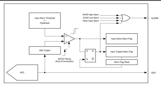
Figure 6-16. Alarm Functionality Schematic
