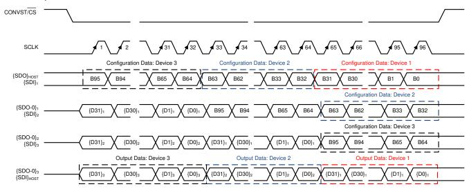
Figure 6-23. Three Devices in Daisy-Chain Mode Timing Diagram
