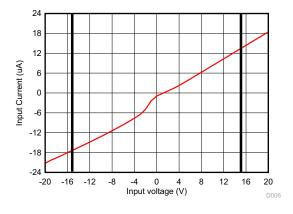
Figure 6-4. I-V Curve for the Input OVP Circuit (AVDD = Floating)
