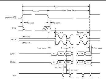
Figure 5-6. multiSPI Interface Timing Diagram for Dual SDO-x and CPHA = 1
