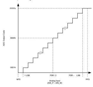
Figure 6-15. Device Transfer Function (Straight-Binary Format)
