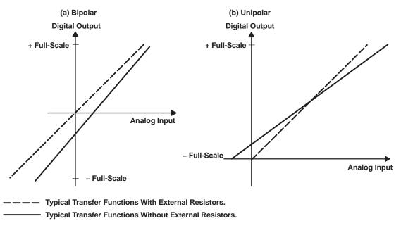
Figure 44. Typical Transfer Functions With and Without External Resistors
