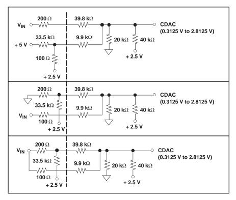
Figure 45. Circuit Diagrams Showing External and Internal Resistors
