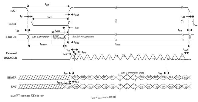
Figure 38. Read After Conversion (Discontinuous External DATACLK)
