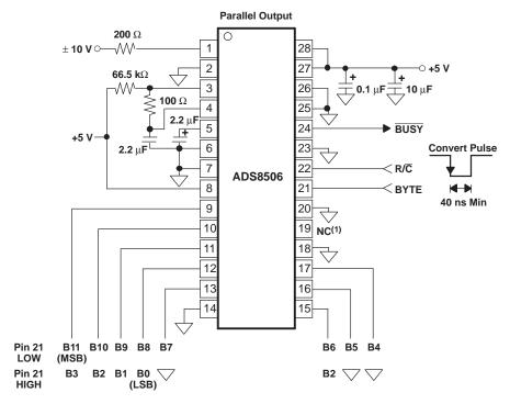
Figure 31. Basic ±10-V Operation, Both Parallel and Serial Output
