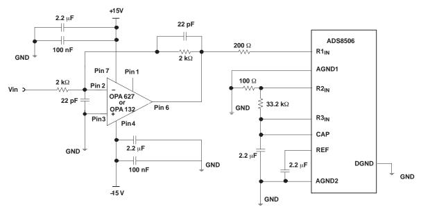
Figure 41. Typical Driving Circuit (±10 V, No Trim)
