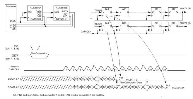
Figure 40. Timing of TAG Feature With Single Conversion (Using External DATACLK)
