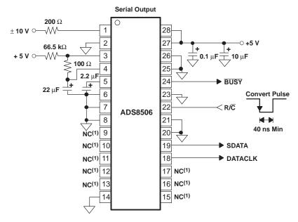
Figure 32. Basic ±10-V Operation With Serial Output
