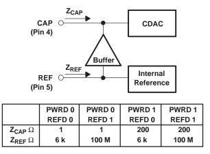
Figure 46. Characteristic Impedances of the Internal Buffer
