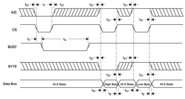
Figure 34. CS to Control Conversion and Read Timing With Parallel Outputs
