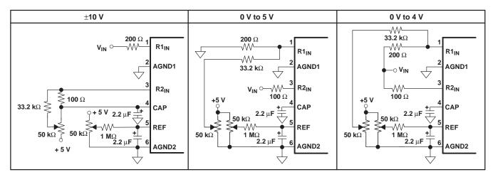
Figure 42. Circuit Diagrams (With Hardware Trim)
