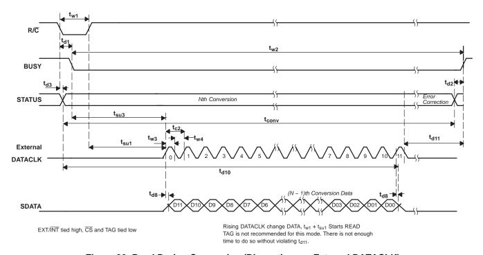
Figure 39. Read During Conversion (Discontinuous External DATACLK)
