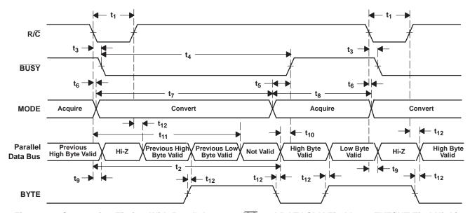
Figure 33. Conversion Timing With Parallel Output (CS and DATACLK Tied Low, EXT/INT Tied High)
