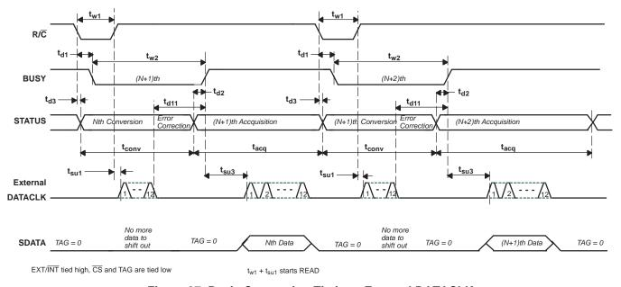
Figure 37. Basic Conversion Timing - External DATACLK
