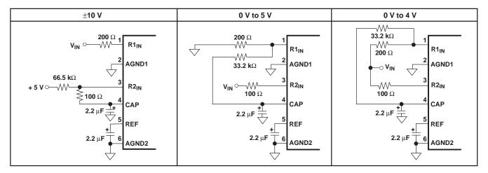
Figure 43. Circuit Diagrams (Without Hardware Trim)
