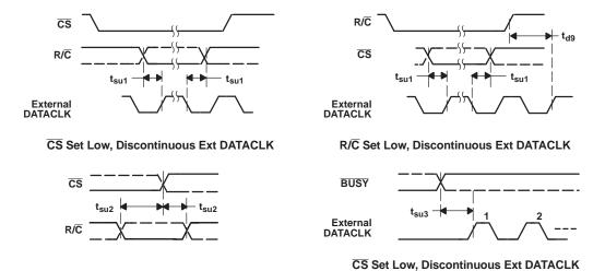
Figure 35. Critical Timing
