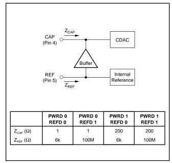
FIGURE 10. Characteristic Impedances of Internal Buffer.
