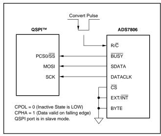
FIGURE 12. QSPI Interface to the ADS7806.
