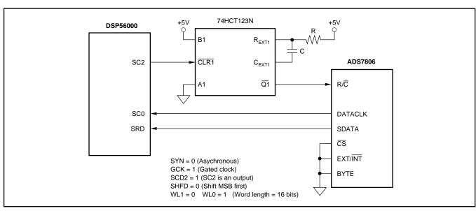
FIGURE 15. DSP56000 Interface to the ADS7806. Processor initiates conversions.
