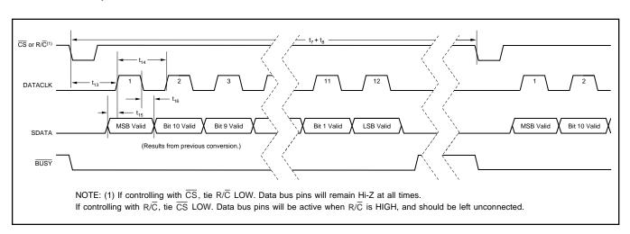
FIGURE 4. Serial Data Timing Using Internal Data Clock (TAG tied LOW).
