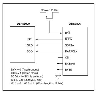
FIGURE 14. DSP56000 Interface to the ADS7806.
