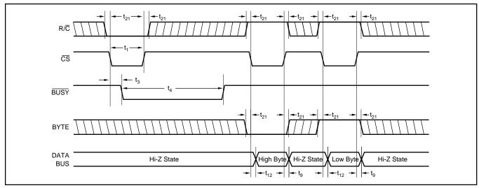
FIGURE 3. Using  $\overline{CS}$  to Control Conversion and Read Timing with Parallel Outputs.
