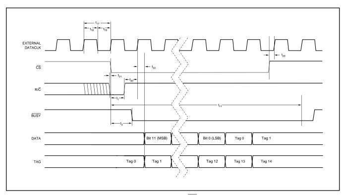
FIGURE 6. Conversion and Read Timing with External Clock (EXT/INT tied HIGH) Read During a Conversion.
