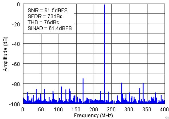
Figure 5. FFT for 230-MHz Input Signal (Auto On)
