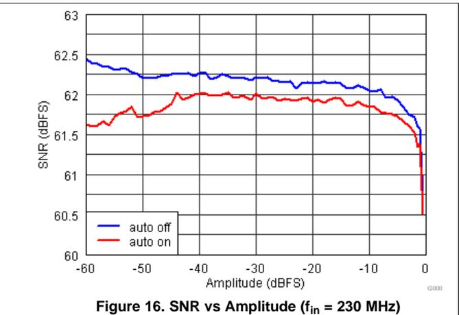
Figure 16. SNR vs Amplitude (f<sub>in</sub> = 230 MHz)
