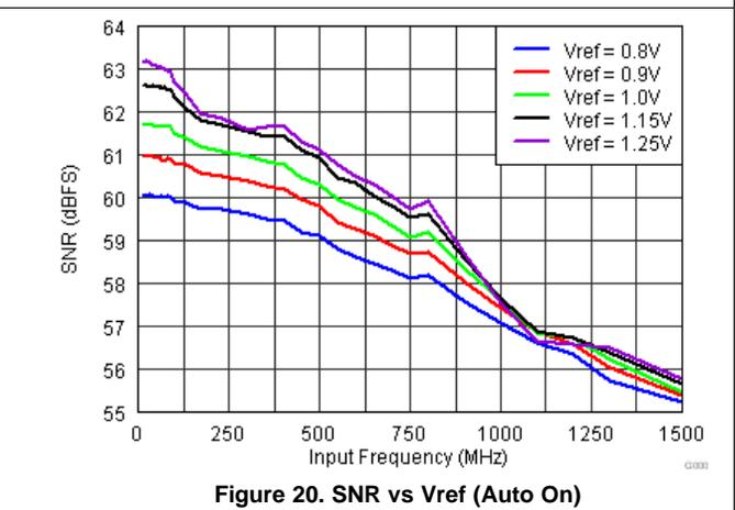
Figure 20. SNR vs Vref (Auto On)
