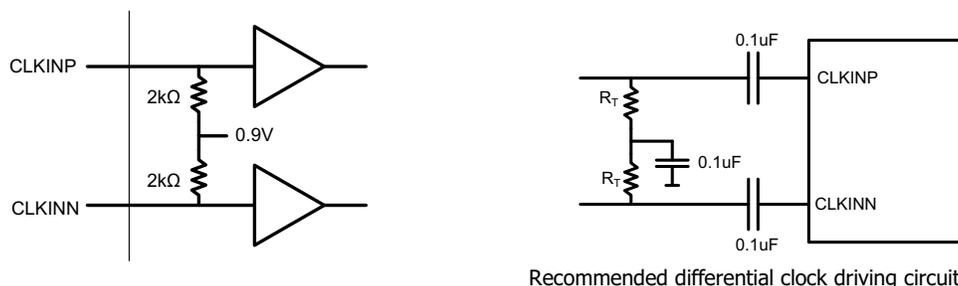
Recommended differential clock driving circuit
