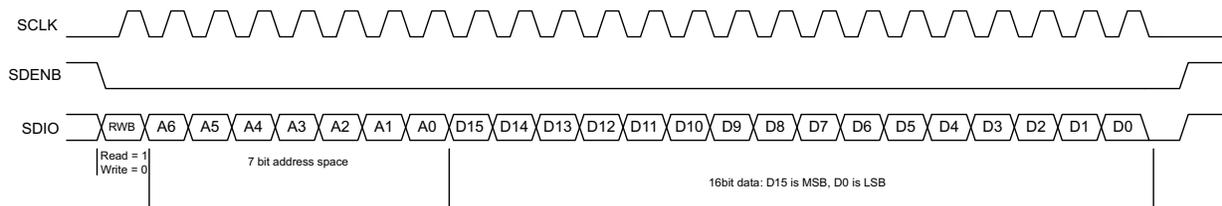
**Figure 46. Serial Register Write Timing Diagram**
