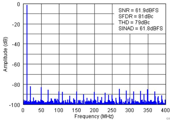
Figure 3. FFT for 10-MHz Input Signal (Auto On)
