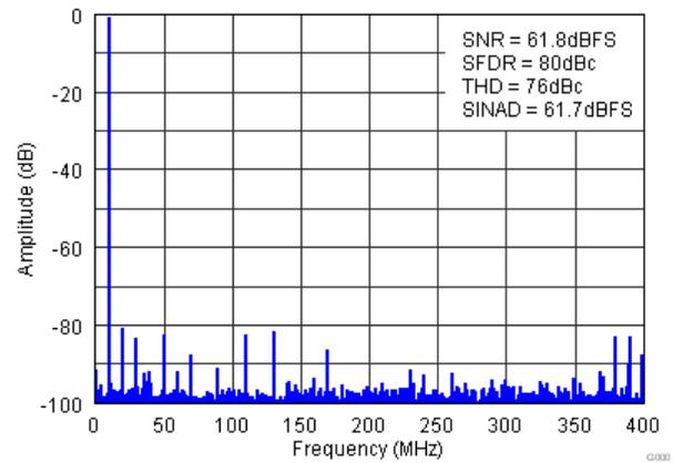
Figure 4. FFT for 10-MHz Input Signal (Auto Off)
