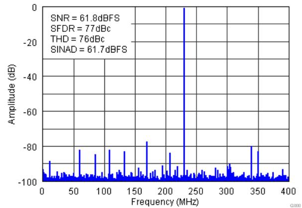
Figure 6. FFT for 230-MHz Input Signal (Auto Off)
