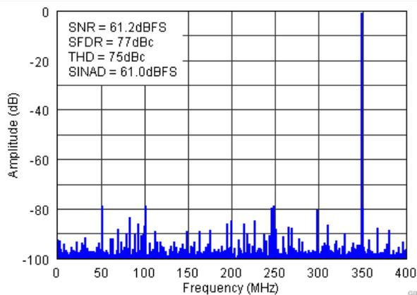
Figure 7. FFT for 450-MHz Input Signal (Auto On)
