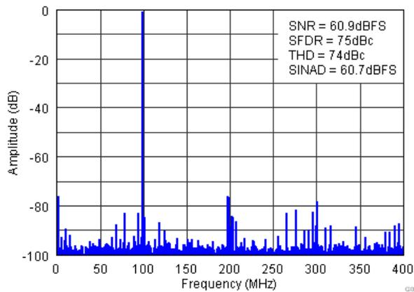
Figure 9. FFT for 700-MHz Input Signal (Auto On)
