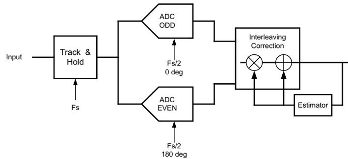
Figure 39. Interleaving Correction Circuit
