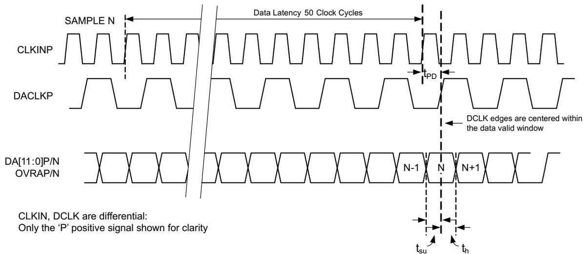
**Figure 1. Timing Diagram for 12-Bit DDR Output**
