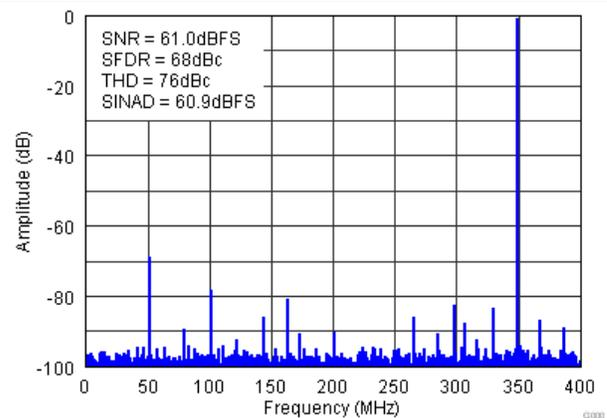
Figure 8. FFT for 450-MHz Input Signal (Auto Off)
