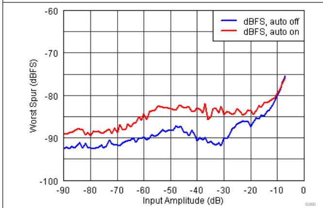
Figure 17. Tow Tone Performance Across Input Amplitude (f<sub>in</sub> = 170 MHz)
