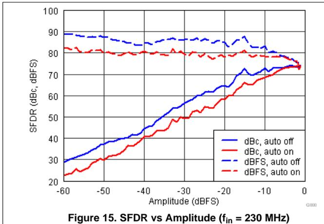
Figure 15. SFDR vs Amplitude (f<sub>in</sub> = 230 MHz)
