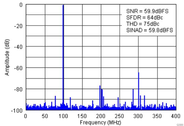
Figure 10. FFT for 700-MHz Input Signal (Auto Off)
