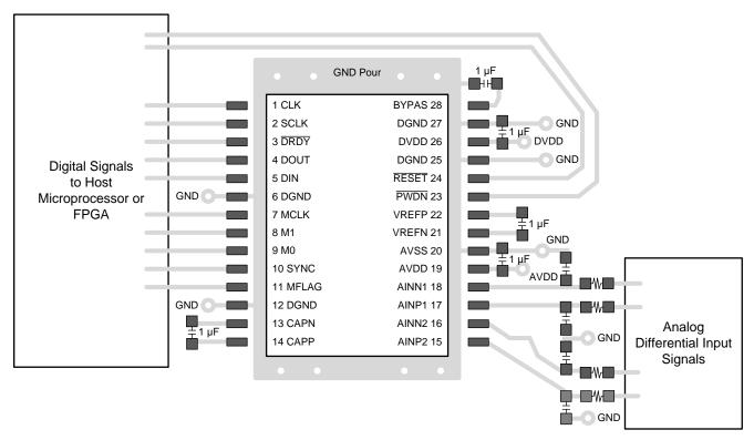
Figure 82. Unipolar Layout Example
