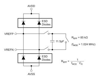
Figure 35. Simplified Reference Input Circuit
