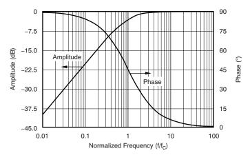
Figure 45. HPF Amplitude and Phase Response
