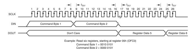
Figure 59. Read Register Data (Equation 11 Shows t<sub>DLY</sub>)
