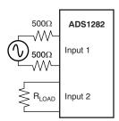
Figure 28. Driving an External Load Through the MUX
