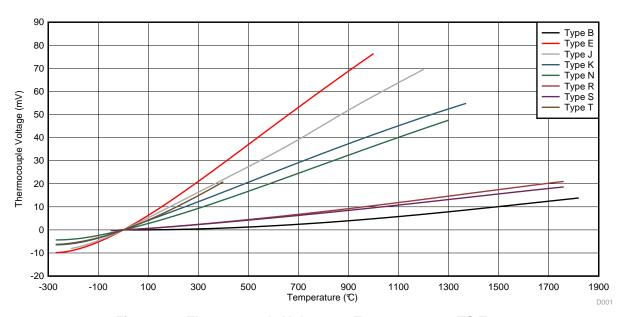
Figure 76. Thermocouple Voltage vs Temperature vs TC Type
