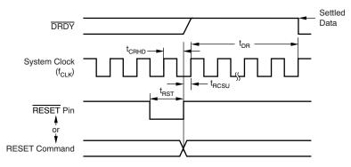
Figure 48. Reset Timing
