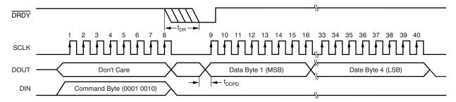
Figure 55. Read Data By Command, Rdata (T<sub>DDPD</sub> Timing Is Given In Read Data Timing Requirements)
