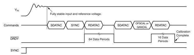
Figure 61. Offset/Gain Calibration Timing
