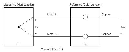
Figure 75. Basic Thermocouple Configuration
