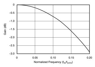
Figure 38. Sinc Filter Roll-Off
