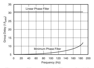
Figure 43. FIR Group Delay ( $F_{DATA} = 500 \text{ Hz}$ )
