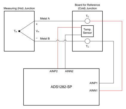
Figure 77. ADS1282-SP as Thermocouple DAQ
