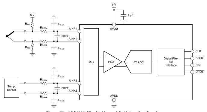
Figure 79. ADS1282-SP with Hot and Cold Junction Sensing
