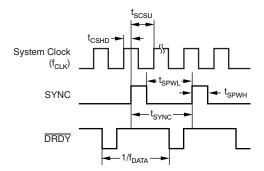
Figure 47. Continuous-Sync Timing With Sync Clock
