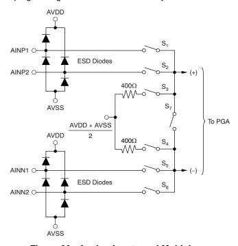
Figure 26. Analog Inputs and Multiplexer
