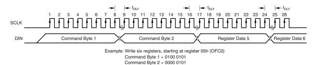
Figure 60. Write Register Data (Equation 11 Shows t<sub>DLY</sub>)
