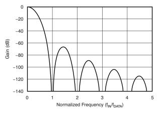
Figure 37. Sinc Filter Frequency Response
