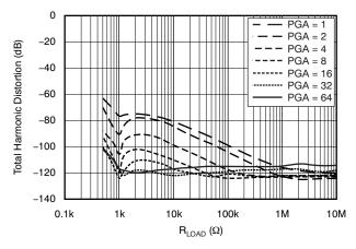
Figure 27. THD vs External Load and Signal Magnitude (PGA) (See Figure 28)
