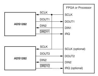
Figure 51. Interface for Multiple Devices
