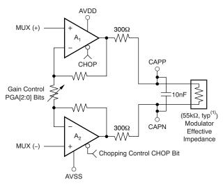
Figure 29. PGA Block Diagram
