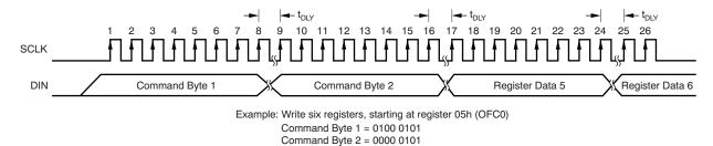
Figure 60. Write Register Data (Shows t<sub>DI Y</sub>)
