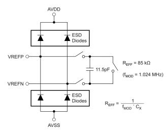
Figure 35. Simplified Reference Input Circuit
