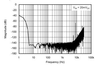
Figure 32. Modulator Output Spectrum
