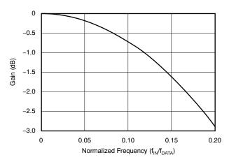
Figure 38. Sinc Filter Roll-Off
