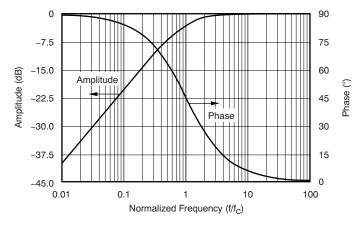
Figure 45. HPF Amplitude and Phase Response
