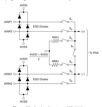
Figure 26. Analog Inputs and Multiplexer
