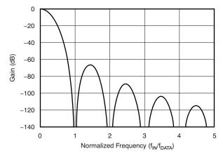
Figure 37. Sinc Filter Frequency Response
