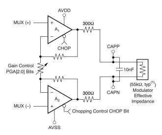
Figure 29. PGA Block Diagram
