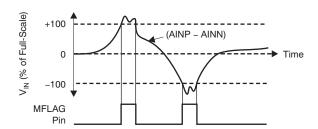
Figure 34. Modulator Over-Range Flag Operation
