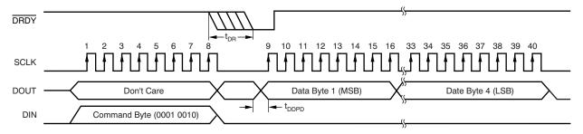
Figure 55. Read Data By Command, Rdata (T<sub>DDPD</sub> Timing Is Given In Read Data Timing Requirements)
