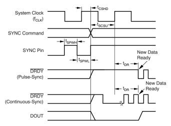
Figure 46. Pulse-Sync Timing, Continuous-Sync Timing With Single Sync
