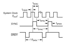
Figure 47. Continuous-Sync Timing With Sync Clock
