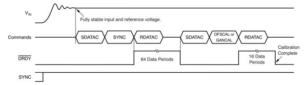
Figure 61. Offset/Gain Calibration Timing
