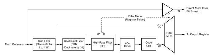
Figure 36. Digital Filter and Output Code Processing
