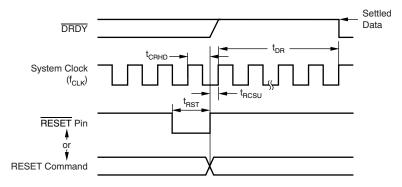
Figure 48. Reset Timing
