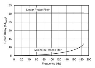
Figure 43. FIR Group Delay ( $F_{DATA} = 500 \text{ Hz}$ )
