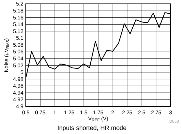
Figure 19. Noise vs V_{REF}
